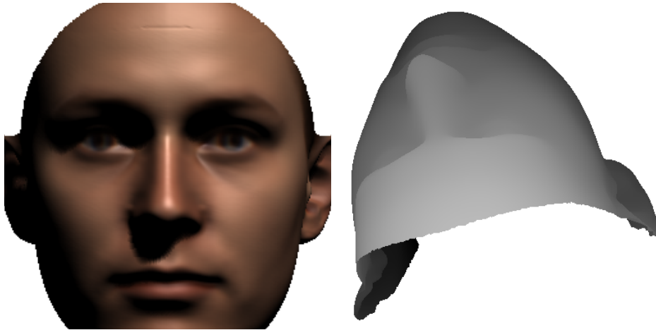
Figure 2.6: Shadow buffer (right) for a light source that is used to render the face (left), similar to rendering of a z-buffer. The angle of the light source is \approx (52^\circ, 20^\circ) . Note that the shadowed areas are not visible to the light source, and thus hidden in the visualization of the shadow buffer.
