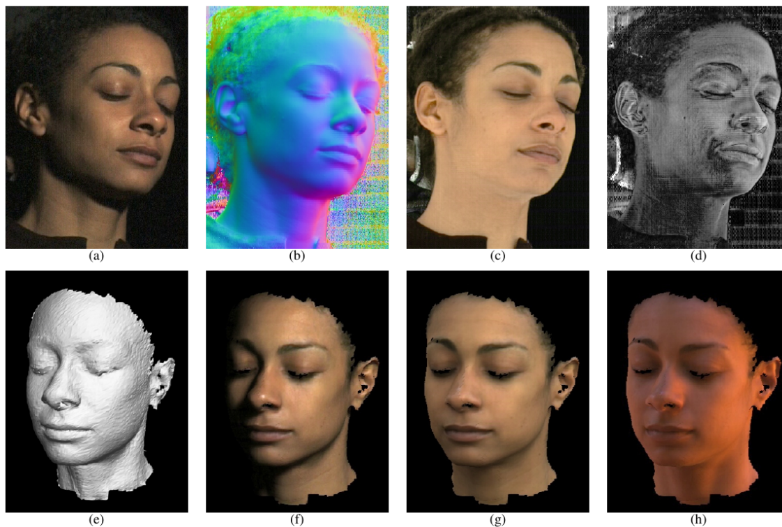
Figure 2.1: Light stage results, courtesy of Debevec et al.: “. . . (a) an original light stage image taken by the left camera. (b) recovered surface normals . . . derived from the fitted diffuse reflectance lobe for each pixel; (b) the RGB value for each pixel encodes the X, Y, and Z direction of each normal. (c) Estimated diffuse albedo . Although not used by our rendering algorithm, such data could be used in a traditional rendering system. (d) Estimated specular energy , also of potential use in a traditional rendering system. (e) Face geometry recovered using structured lighting. (f) Face rendered from a novel viewpoint under synthetic directional illumination. (g,h) Face rendered from a novel viewpoint under two sampled lighting environments . . .” [DHT + 00].
