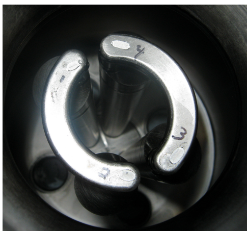
Figure 5.4: Indium Crush Test: The four indium test strips are placed at the ends of the niobium loops, and subsequently crushed by fastening the sample piece into position. The results show good agreement with the target value (red).
