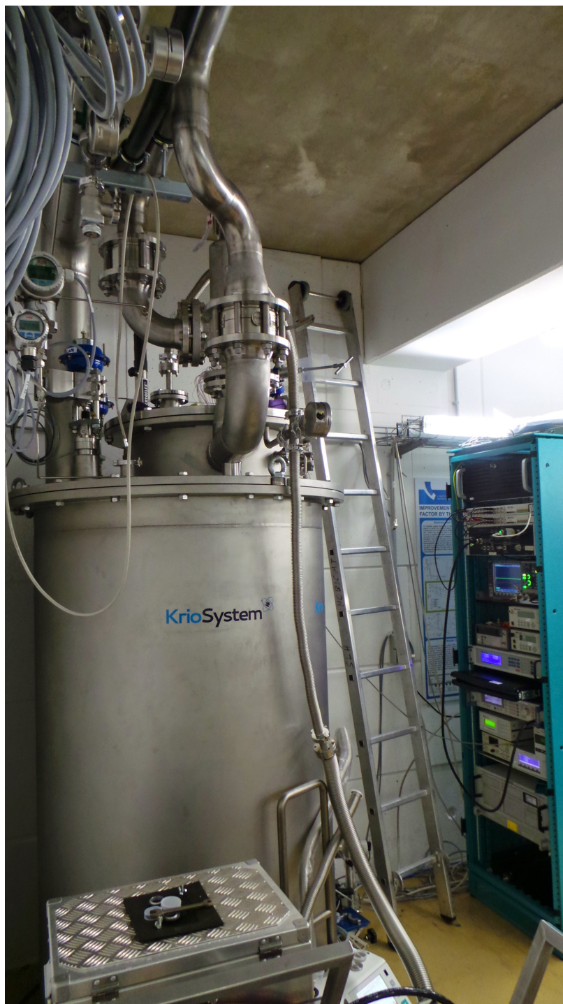
Figure 6.5: Photo of the helium cryostat and the 19 inch rack housing the RF and thermometry control system.
