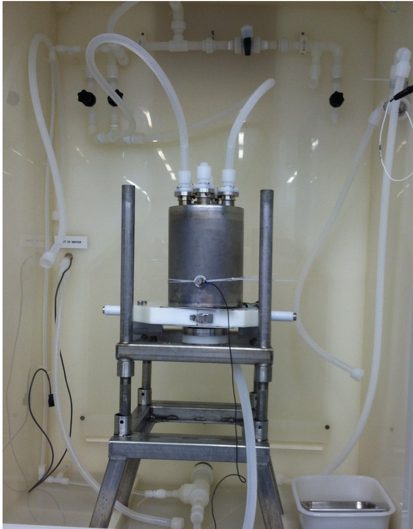
Figure 5.5: Photo of the QPR mounted in the JLab BCP cabinet. The acid inlet is through the bottom opening where the thermometry chamber is mounted, two of the top auxiliary ports are used as outlets.
