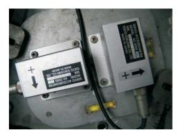
**Figure 6.10.** An example of 2 accelerometers installed on the Canton Tower (http://www.cse.polyu.edu.hk/benchmark)
