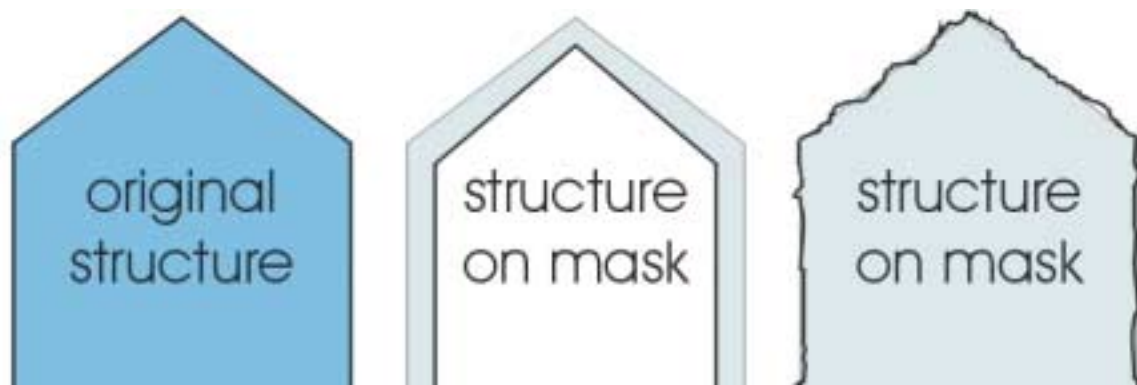
Figure 22: Example of bad absolute precision (central image) and of high edge roughness (right image). The original structure is presented in the left drawing, and is also under laid to the other two images to mark the differences. According to one's needs, a trade-off between the two characteristics is usual.
