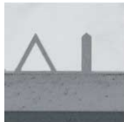
SEM micrograph of triangular and rectangular cantilevers
