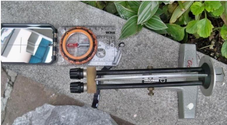
*Fig. 3: Measurement setup to determine the inclination in one place. The parallelism of the inclinorium and the connecting line of the magnetic poles is important. Photo: Volker Heck.*
