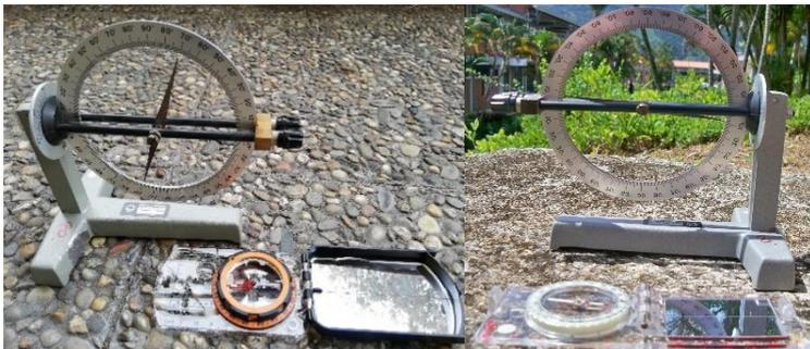
*Fig. 4: The use of an inclinometer in Siegen (left) and Quito (right): Clearly observable is the difference of inclination. Photo: Volker Heck.*
