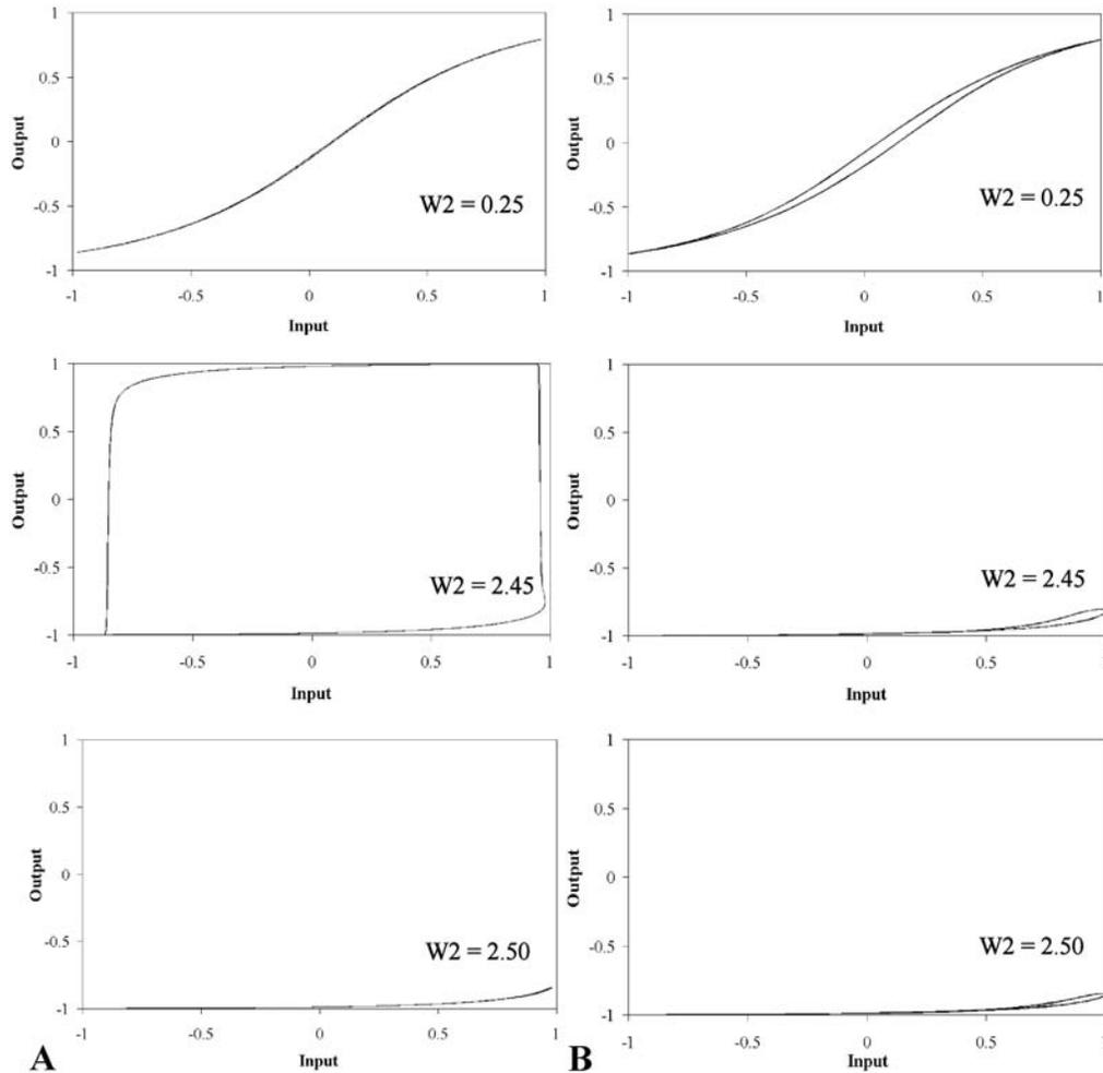
Figure 5.4: Comparison of the “hysteresis effects” between input and output signals of high- and low-frequency sounds for  $W_2 = 0.25$ ,  $2.45$  and  $2.50$ , respectively. (A) Low-frequency sound (100 Hz); (B) High-frequency sound (1000 Hz).
