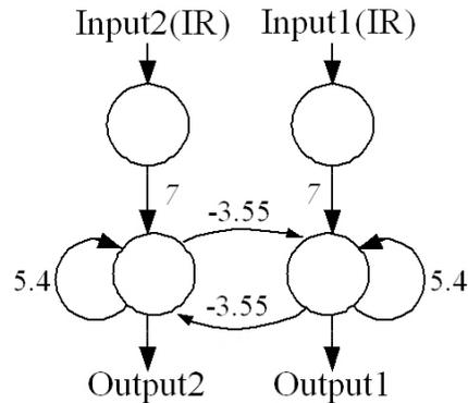
Figure 5.20: The signal processing network of antenna-like sensors with appropriate weights. The network is developed to operate at an update frequency of 75 Hz.
