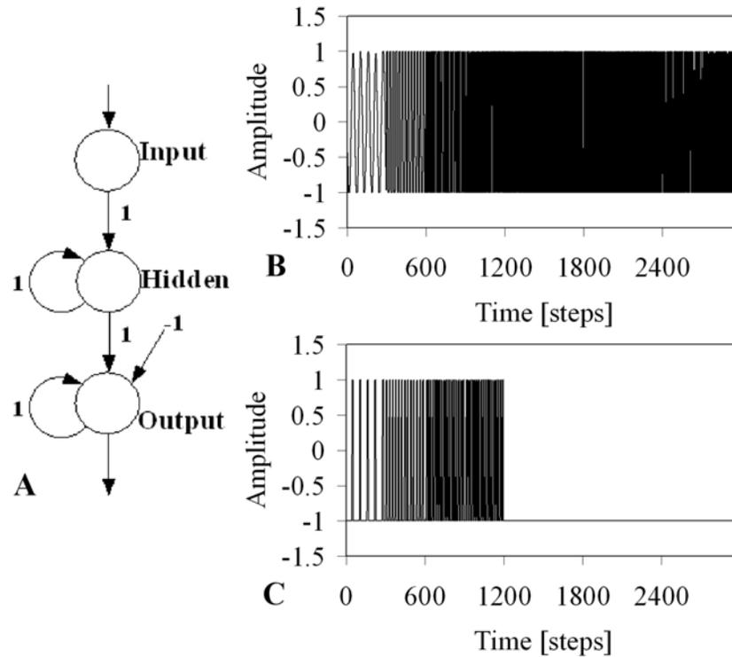
Figure 5.8: (A) An initial network structure with given weights and a bias. (B) The varying frequencies of an input signal from 100 Hz to 1000 Hz. The input signal is recorded from the physical stereo auditory sensor and then digitized through the analog to digital converter (ADC) channel of the MBoard at a sampling rate of up to 5.7 kHz. (C) A corresponding target signal.
