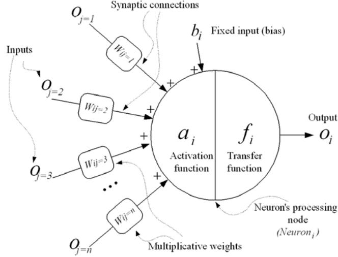
Figure 3.3: The structure of an artificial neuron. Each neuron can have multiple input connections, which can originate from other neurons or from a sensor, but there is only one output signal. Then the single output signal can be distributed in parallel (in other words, multiple connections carrying the same signal) to other neurons or to an external system, e.g. a motor system.
