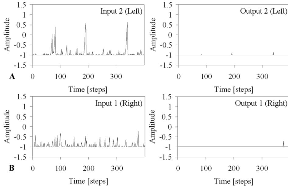
Figure 6.11: Left: The input signals which were firstly filtered via the evolved advanced auditory network before going into the sound-direction detection network. Right: The output signals of the sound-direction detection network. (A), (B) The input and output signals of the sound-direction detection network on the left and right, respectively. Both unwanted parts of noise were all removed by the sound-direction detection network.
