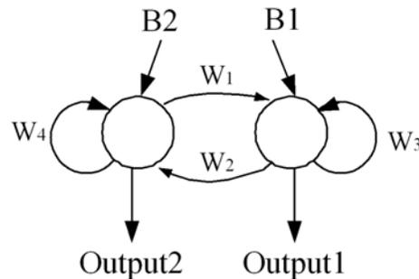
Figure 5.24: The structure of the 2-neuron network.
