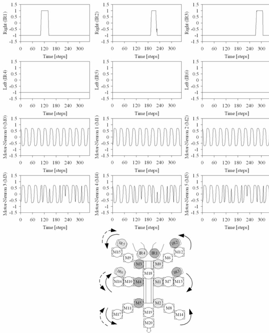
Figure 6.18: An obstacle detected by each of the right sensors (IR1, IR2 and IR3) at different time steps; this caused the left motor neurons (M3, M4 and M5) to change into the opposite direction as indicated by the arrow dashed lines in the lower picture. As a result, the walking machine turns left.
