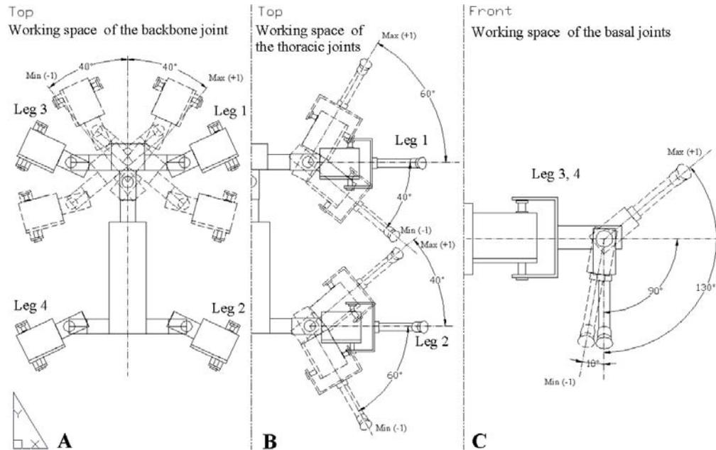
Figure 4.14: (A) The angle range of the backbone joint (top view). (B) The angle ranges of all thoracic joints of the right side of the walking machine with the left side being symmetric (top view). (C) The angle range of the basal joint of the left foreleg with the remaining legs having the same angle ranges (front view).
