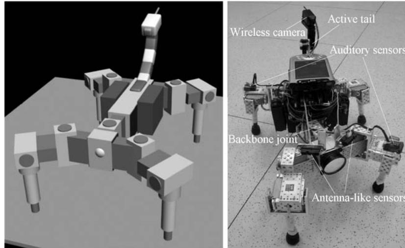
Figure 4.15: The four-legged walking machine AMOS-WD02. Left: The 3D model of the walking machine. Right: The real world walking machine.
