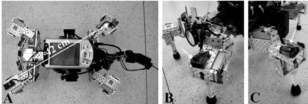
Figure 4.4: (A) The distance between the stereo auditory sensor is equal to 42 cm. (B) The real sensor built in a preamplifier circuit was installed on the left foreleg of the walking machine. (C) The sensor was installed on the right hind leg of the walking machine.
