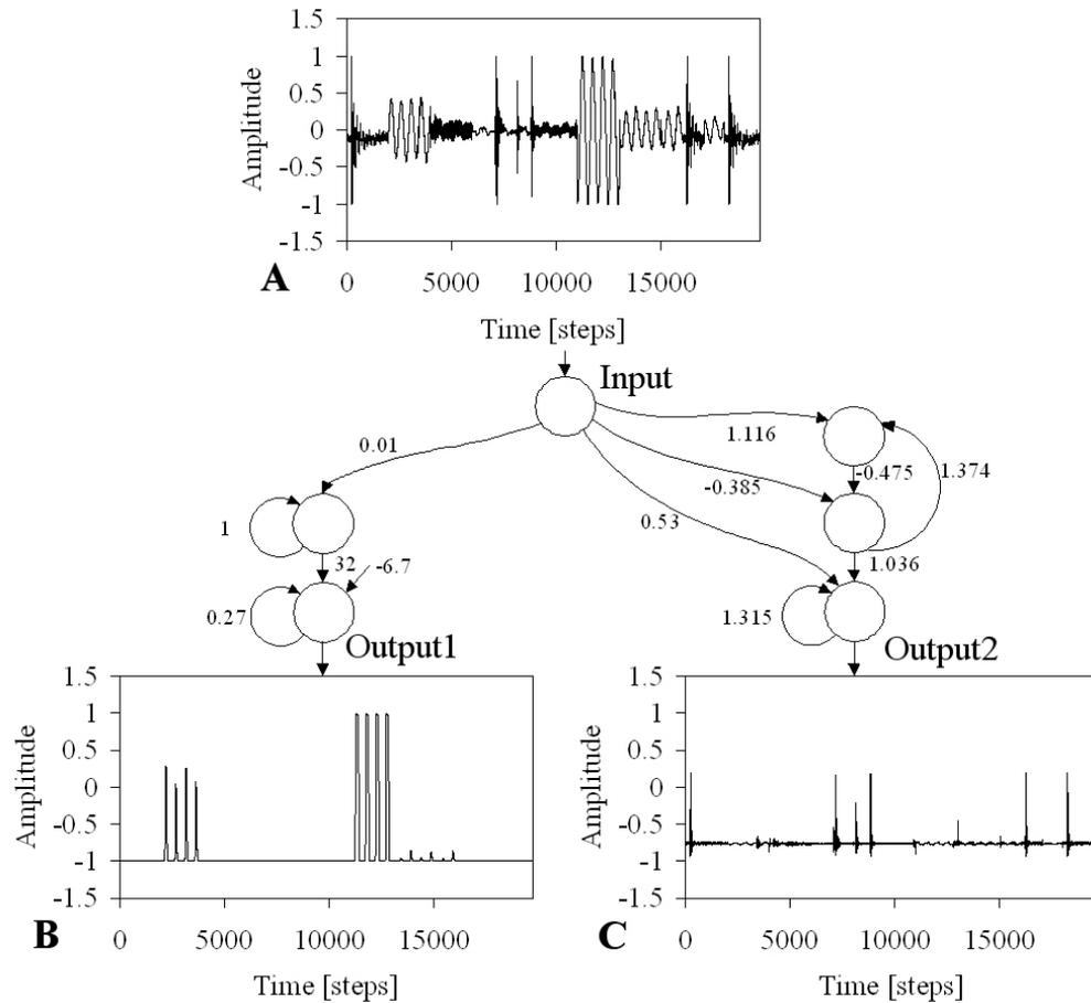
Figure 6.6: (A) The mixed signals between the low-frequency sound (100 Hz) with varying amplitudes and the tactile signal. They were recorded via the auditory-tactile sensor. (B) The response of the network to the low-frequency sound. (C) The response of the network to the tactile signal. Both outputs are active only for sound and the tactile signal. All figures have the same scale in x-axis and y-axis.
