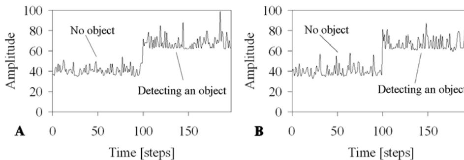
Figure 4.12: The sensory signals coming from the left fore (A) and the right fore (B) heads of the four-legged walking machine.
