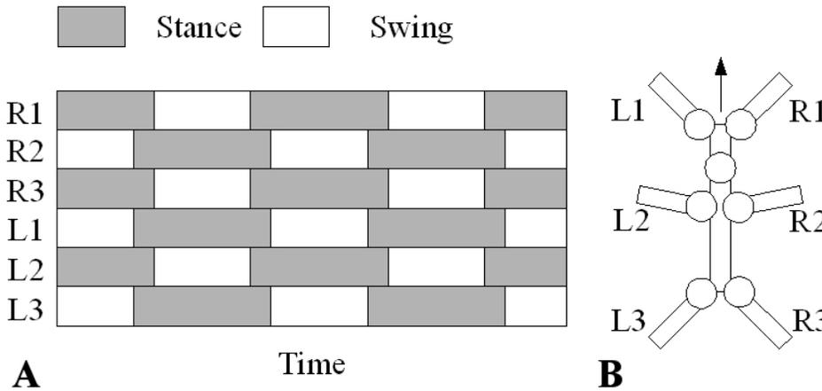
Figure 5.29: (A) The typical tripod gait. X-axis represents time and y-axis represents the legs. During the swing phase (white blocks) the feet have no ground contact. During the stance phase (gray blocks) the feet touch the ground. (B) The orientation of the legs of the AMOS-WD06.
