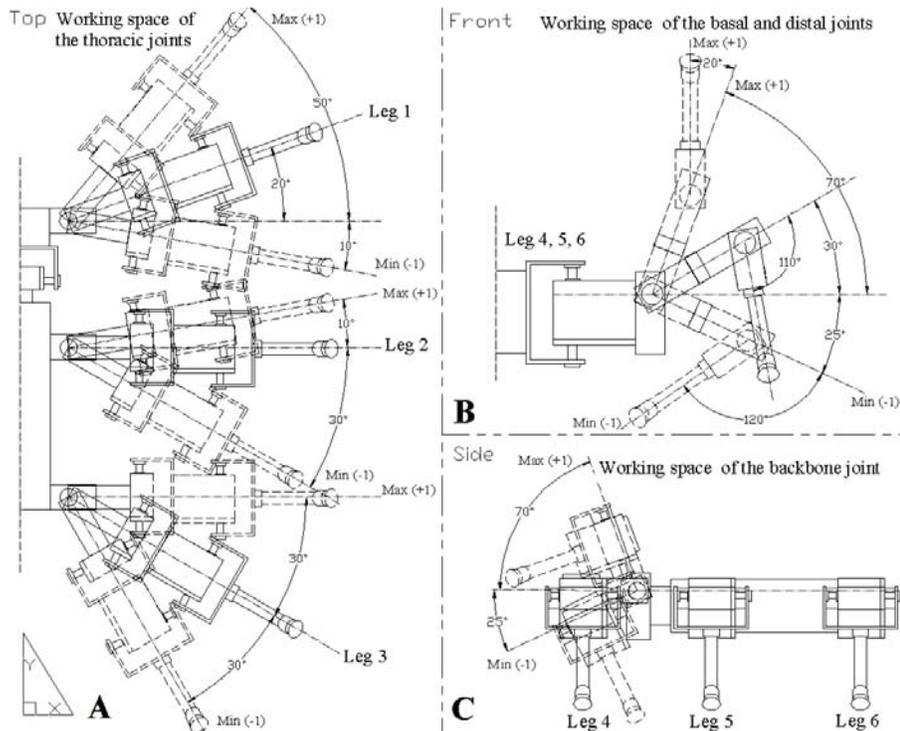
Figure 4.19: (A) The angle ranges of all thoracic joints on the right side of the walking machine with the left side being symmetric (top view). (B) The angle ranges of the basal and distal joints of the left foreleg with the remaining legs having the same angle ranges (front view). (C) The angle range of the backbone joint (side view).
