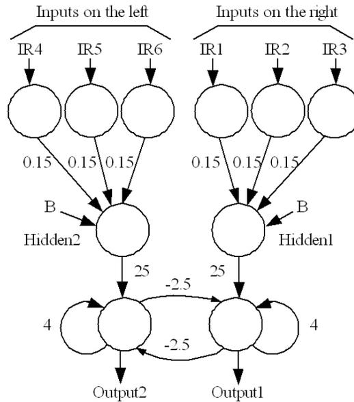
Figure 5.21: The signal processing network of antenna-like sensors for the six sensory inputs. The network is also developed to operate at an update frequency of 75 Hz.
