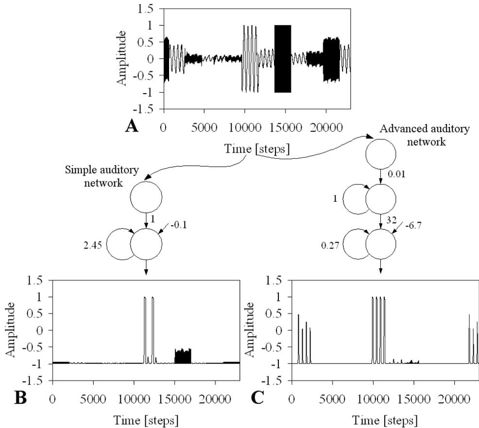
Figure 6.3: (A) The real input signals (consisting of 100 Hz and 1000 Hz) with varying amplitudes recorded via the physical auditory-tactile sensor. (B) The corresponding output signals of the simple auditory network. (C) The corresponding output signals of the advanced auditory network. All figures have the same scale in x-axis and y-axis.
