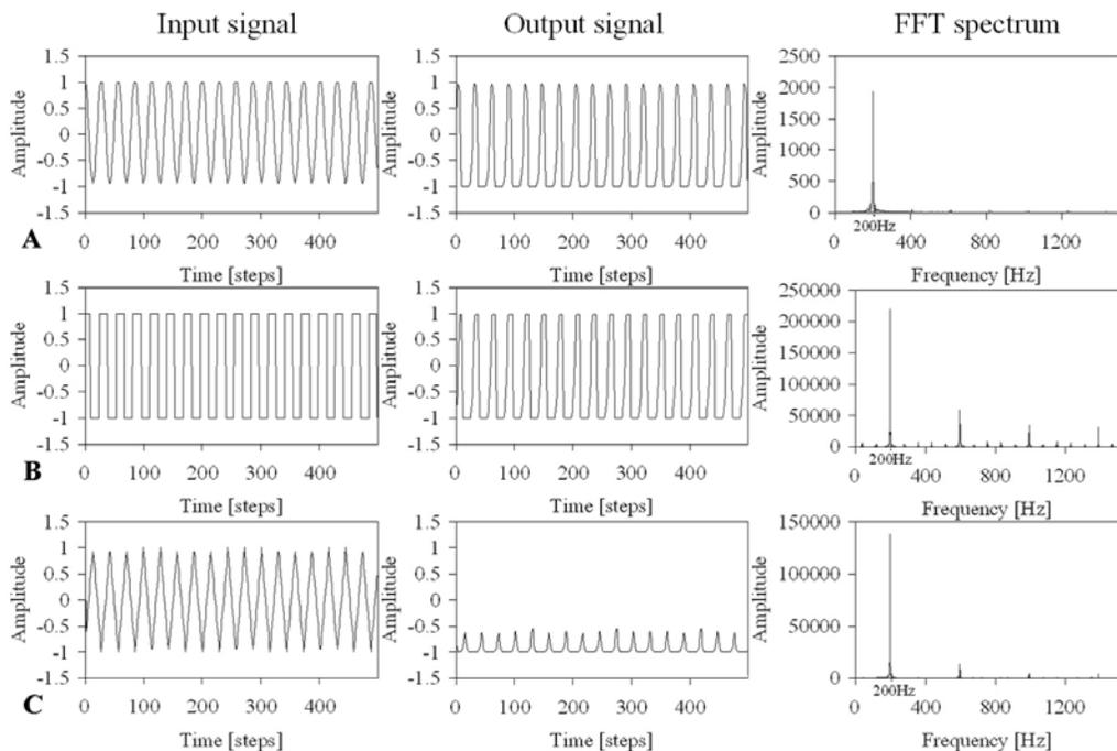
Figure 6.10: Left: The different waveforms of the input signal at 200 Hz generated by a function generator. Middle: The output signal of the network with respect to the input signal on the left side. Right: The FFT spectrum of each input signal. (A) The signal having a sine shape. (B) The signal having a square shape. (C) The signal having a triangle shape.
