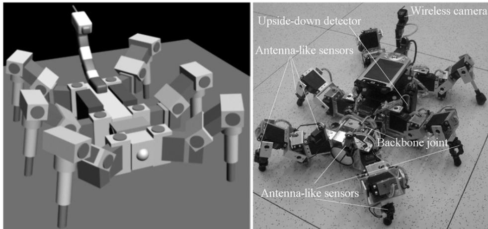
Figure 4.20: The six-legged walking machine AMOS-WD06. Left: The 3D model of the walking machine. Right: The real walking machine.
