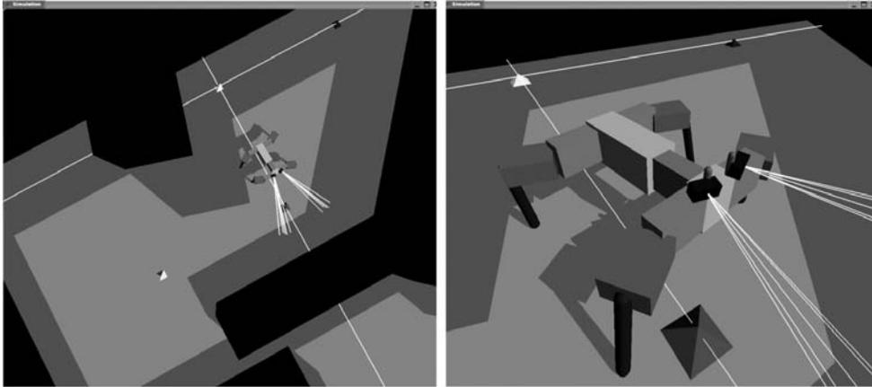
Figure 4.16: Different view of the simulated walking machine in its environment. The properties of all simulated components are defined with respect to the physical properties of the real walking machine, e.g. weight, dimension, motor torque and so on. The simulated walking machine consists of body parts (head, backbone joint, trunk and limbs), servomotors and IR sensors while the auditory sensor was not available in the simulation.
