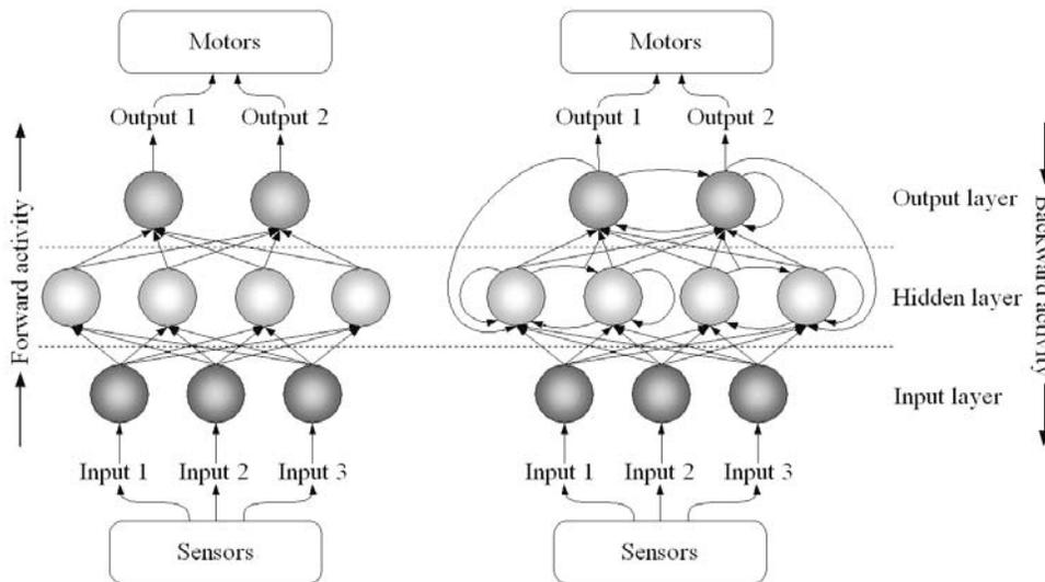
Figure 3.5: Examples of a feedforward network (left) and a recurrent network (right). Generally for robot control, the inputs of the networks can be provided by sensors while their outputs can be sent out to control motors.
