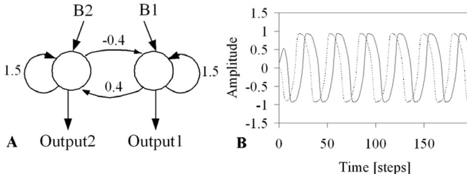
Figure 5.26: (A) The structure of the neural oscillator network with the synaptic weights for locomotion control and  $B_1 = B_2 = 0.01$ . (B) The output signals of neurons 1 (dashed line) and 2 (solid line) from the neural oscillator network. The output of neuron 1 is used to drive all thoracic joints and an additional backbone joint and the output of neuron 2 is used to drive all basal joints (and all distal joints for 3 DOF each leg).
