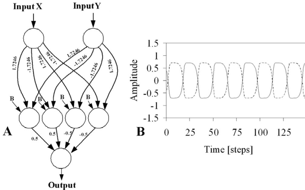
Figure 5.30: (A) The VRN with four hidden neurons and the given bias terms  $B$  which are all equal to  $-2.48285$ . The Input1  $x$  is the oscillating signal coming from the neural oscillator and the Input2  $y$  is the output signal of the neural preprocessing. (B) The output signal (solid line) when the input  $y$  is equal to  $+1$  and the output signal (dashed line) when the input  $y$  is equal to  $-1$ .
