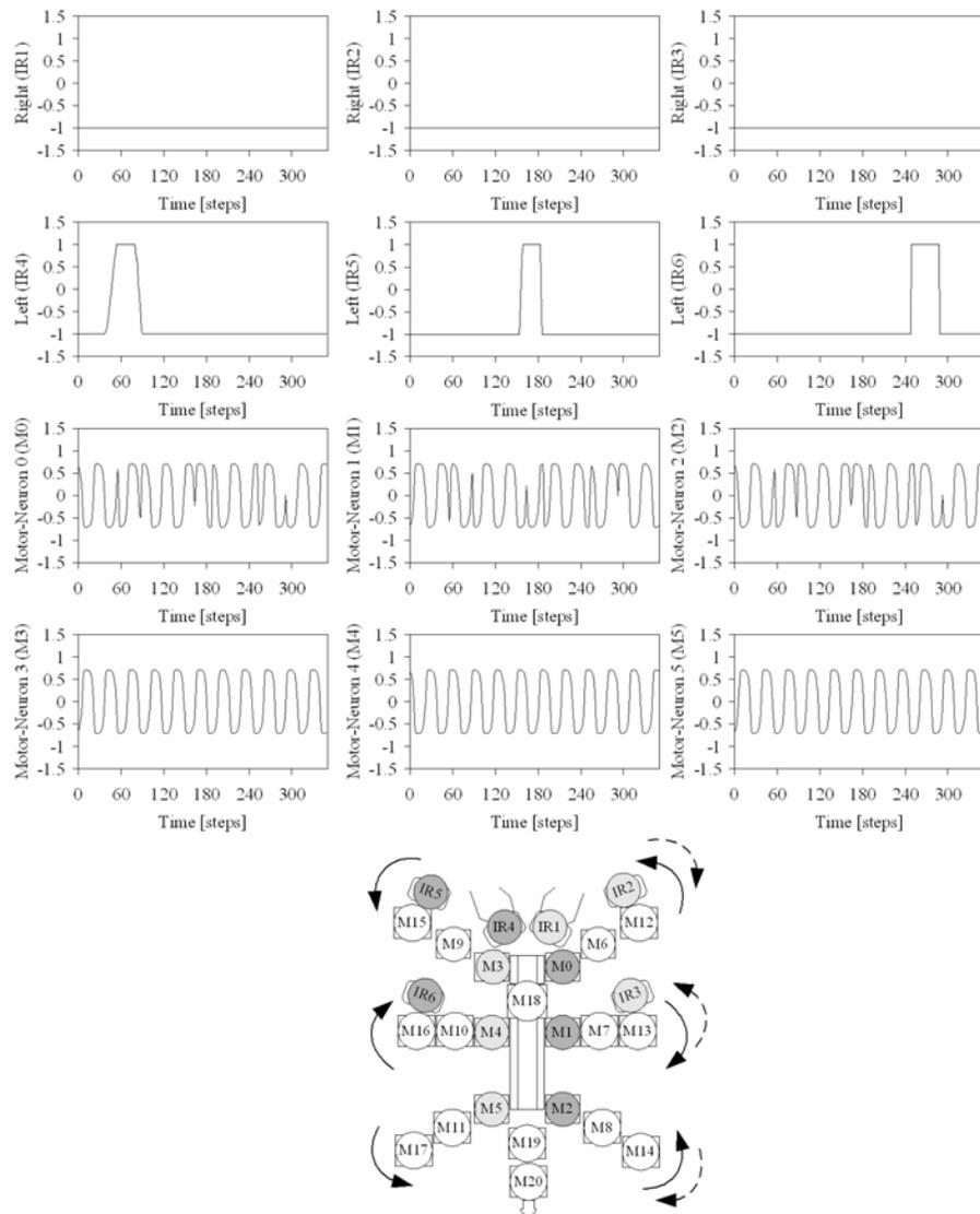
Figure 6.19: An obstacle was presented at each of the left sensors (IR4, IR5 and IR6) at different time steps; this caused the right motor neurons (M0, M1 and M2) to change into the opposite direction as indicated by the arrow dashed lines in the lower picture. As a result, the walking machine turns right.
