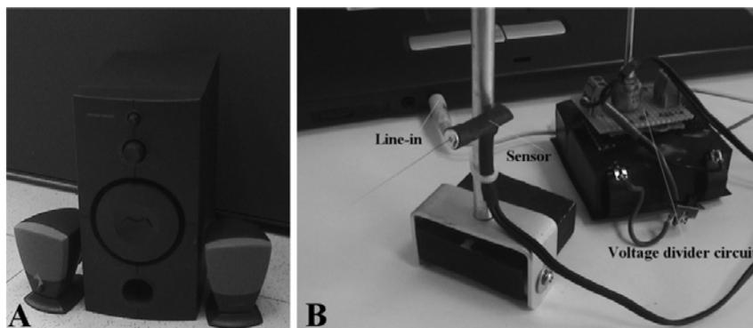
Figure 6.2: The experimental equipment to record real auditory signals via the auditory-tactile sensor. (A) The loudspeaker producing the low- and high-frequency sounds. (B) The auditory-tactile sensor system consisting of the sensor, a voltage divider circuit and a PC having a line-in port.
