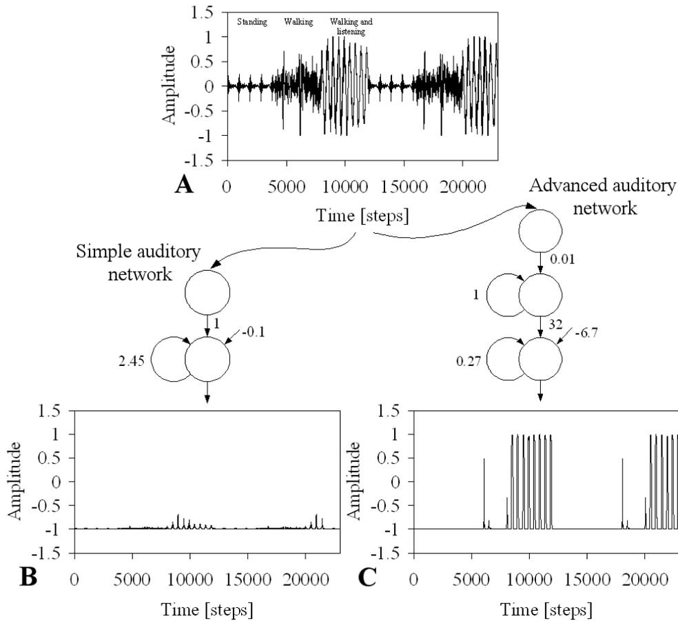
Figure 6.5: (A) The real input signals consisting of three different conditions (standing, walking and walking while listening to the sound). (B) The corresponding output signal of the simple auditory network. (C) The corresponding output signal of the principal advanced auditory network. All figures have the same scale in x-axis and y-axis.
