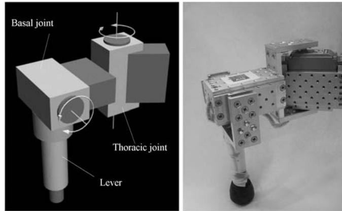
Figure 4.13: The leg with two DOF. Left: The 3D model of the leg. Right: The physical leg of the AMOS-WD02.
