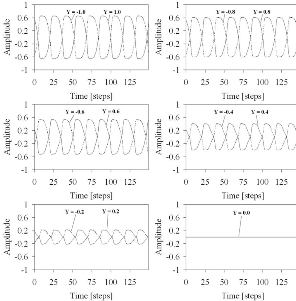
Figure 5.31: The output signal (solid line) when the input  $y$  is equal to positive value and the output signal (dashed line) when the input  $y$  is equal to negative value. The different given values of the input  $y$  result in the different amplitudes of the output signal.
