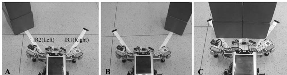
Figure 6.13: (A) The situation where objects were presented on the left side in front of the walking machine at a distance of 25 cm. (B) The situation where objects were presented on the right side having the same distance like in (A). (C) The situation where objects were presented on both sides at the closer distance of 10 cm.
