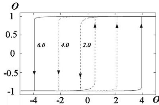
Figure 3.8: Comparison of the “hysteresis effects” between the input  $\theta$  and output  $O$  for  $w = 2.0, 4.0$  and  $6.0$ , respectively (modified from F. Pasemann 2005 [116]).
