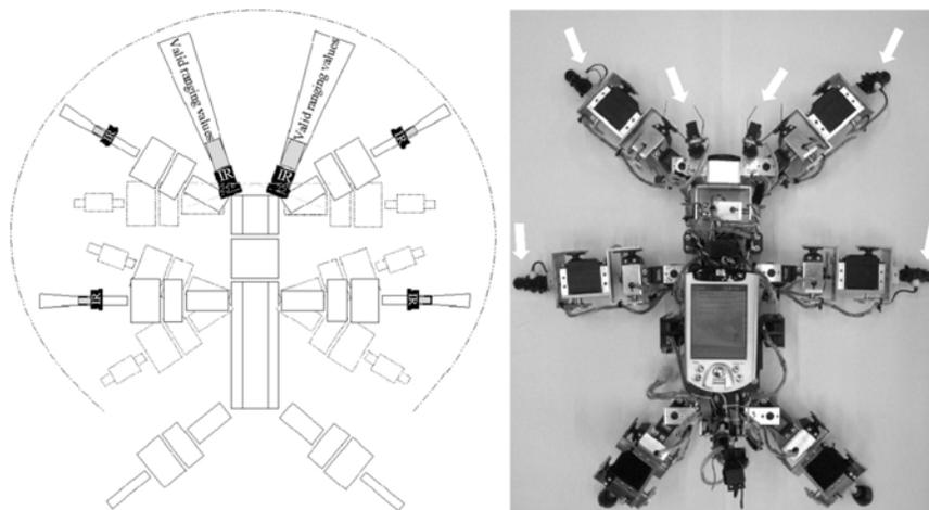
Figure 4.9: Left: The visualization of the locations where the sensors are implemented and the idealized field of the sensors protecting the walking machine from crashing into obstacles (dashed line around the walking machine). Right: The six sensors on the physical walking machine (arrow lines).
