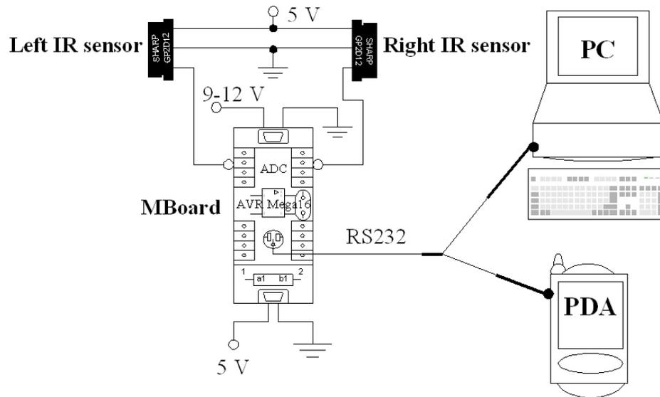
Figure 4.11: The basic schematic of the antenna-like sensor system. Here, two sensors are presented. They are connected to the ADC channels of the MBoard. The digital signals from the MBoard will be displayed or analyzed on a PC or a PDA via an RS232 interface.
