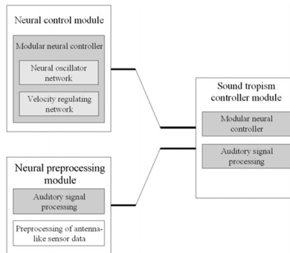
Figure 5.38: The modular architecture of the sound tropism consists of the neural preprocessing and control modules. The auditory signal processing of the neural preprocessing module is chosen to connect to the modular neural controller (of a four- or six-legged walking machine).
