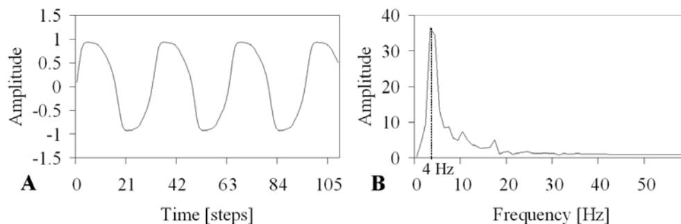
Figure 5.27: (A) The sinusoidal output generated by the neural oscillator network is recorded for 5 seconds. (B) The FFT spectrum of the recorded sinusoidal output shows that the output has the eigenfrequency around 4 Hz. Then, the walking frequency of the machines can be approximately  $(4/5)$  0.8 Hz.
