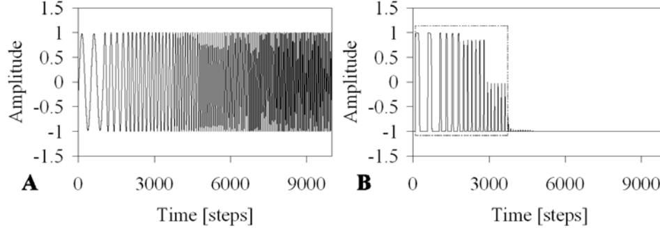
Figure 5.6: (A) The varying frequencies of an input signal from 100 Hz to 1000 Hz. (B) The output signal of the network. The dashed frame is the frequency range (from 100 Hz to approximately 400 Hz) in which the network can detect the auditory signal. Here, the amplitude of the signal which is smaller than a threshold value, e.g. 0.5, is neglected.
