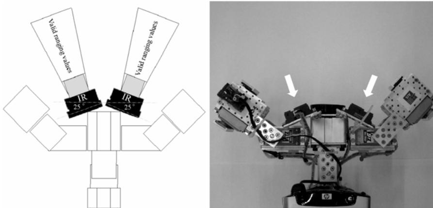
Figure 4.7: The antenna-like sensors implemented on the forehead of the four-legged walking machine. Left: The outline of the sensors from a top view. Right: The real sensors fixated on the forehead of the physical four-legged walking machine AMOS-WD02 (arrow lines).
