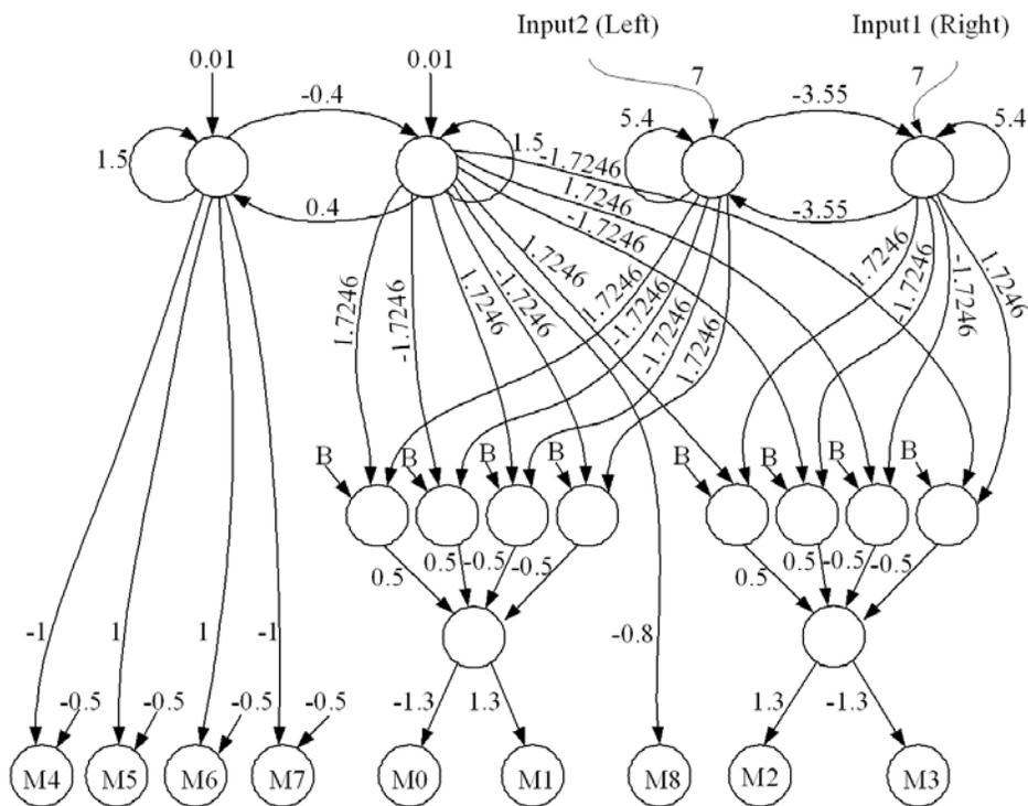
Figure 5.36: The controller is built from a combination of the preprocessing of antenna-like sensor data and the modular neural controller of the four-legged walking machine. The left and the right signals of the antenna-like sensors are directly connected to input neurons of the signal processing network.
