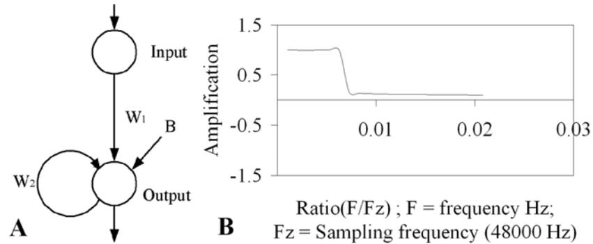
Figure 5.2: (A) The simple auditory network realizing a low-pass filter; parameters are  $W_1 = 1$ ,  $W_2 = 2.45$  and  $B = -0.1$ . (B) The characteristic curve of this network with its cutoff frequency at approximately 300 Hz.
