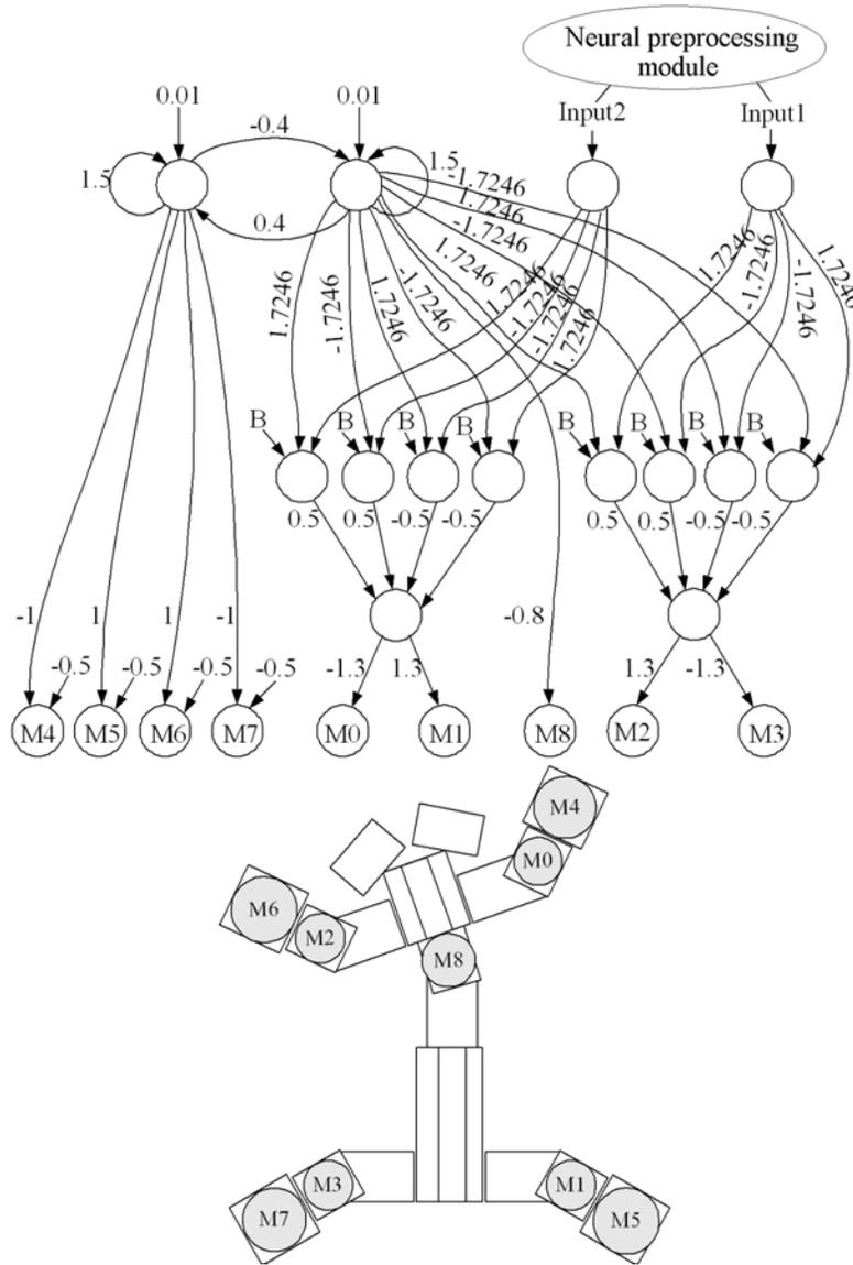
Figure 5.33: The modular neural controller of the four-legged walking machine AMOS-WD02. It generates a trot gait which is modified when  $I_1$  or  $I_2$  is changed by the sensory signals. The bias terms  $B$  of the VRNs are all equal to  $-2.48285$ . The outputs from the neural preprocessing module are directly connected to the input neurons ( $I_1$ ,  $I_2$ ) of the neural control module.
