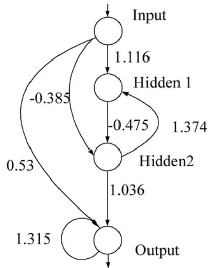
Figure 5.17: The tactile signal processing network. It filters the low-frequency sound. Its output signal follows the tactile signal, which consists of many frequencies and which has resonance frequencies at relatively high.
