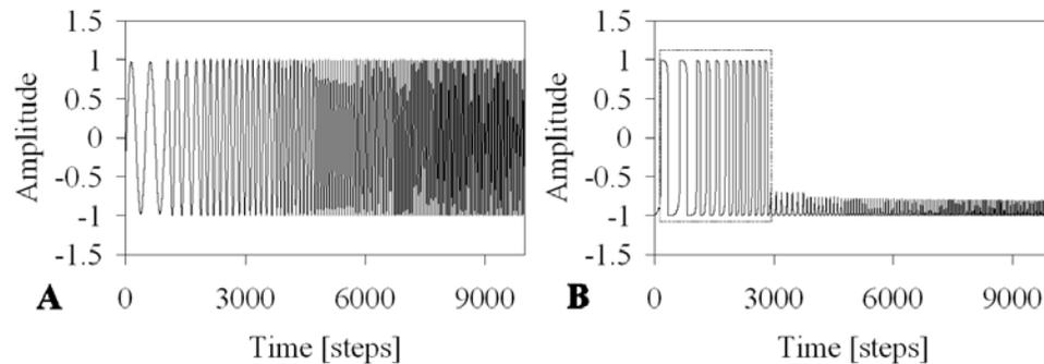
Figure 5.3: (A) The varying frequencies of an input signal from 100 Hz to 1000 Hz. (B) The output signal of the network. The dashed frame is the frequency range (from 100 Hz to approximately 300 Hz) in which the network can detect the auditory signal.
