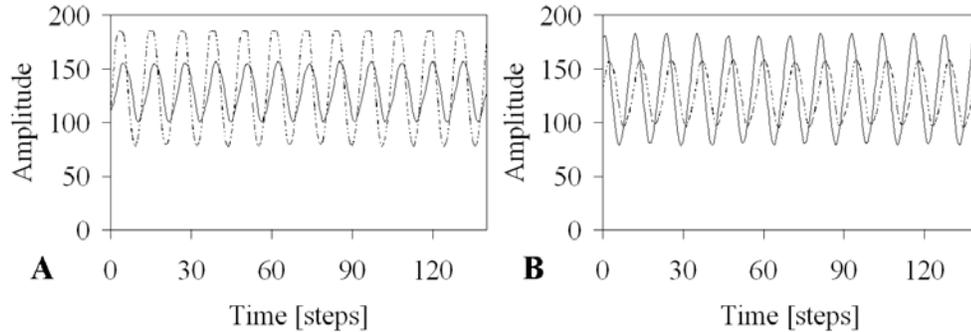
Figure 4.6: (A) The sound source is close to the fore left microphone. This results in the signal coming from the fore left microphone (dashed line) having high amplitude and it is followed by the signal coming from the rear right microphone (solid line) with a delay while the reverse case is presented in (B). All figures have the same scale in x-axis and y-axis.
