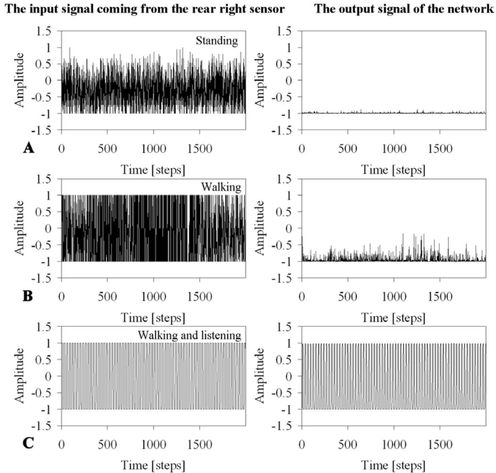
Figure 6.9: Left: The input signal coming from the rear right sensor under three different conditions. Right: The output signal of the evolved advanced auditory network with respect to the input on the left side. (A) The noisy signal when the machine was in a standing position. (B) The noisy signal during the walk. (C) The noisy signal which was compensated between the sound and a noise during the walk. All figures have the same scale in x-axis and y-axis.
