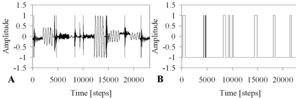
Figure 5.16: (A) A real input signal coming from the physical sensor. It is mixed between the tactile signal and the low-frequency sound at 100 Hz. (B) The corresponding target function.
