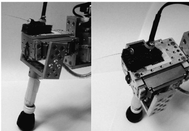
Figure 6.4: The auditory-tactile sensor was installed on one leg of the AMOS-WD02. The sensor has the extension part (the whisker of a real mouse) around 4.0 cm from the leg.
