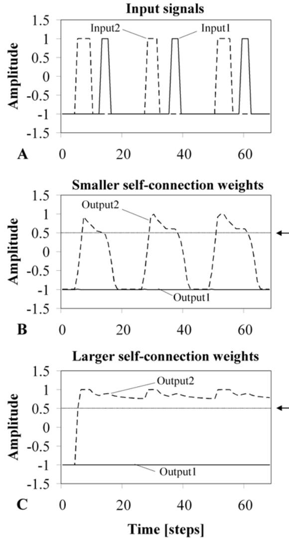
Figure 5.13: (A) The input signals with a delay. (B) shows the corresponding oscillating  $O_2$  (dashed line) for the smaller self-connection weights ( $w_1 = 2.0$ ,  $w_2 = 3.5$ ) while  $O_1$  (solid line) is suppressed. (C) shows that  $O_2$  jumps and stays higher than a threshold (here 0.5 (arrow lines)) for larger self-connection weights ( $w_1 = 2.206$ ,  $w_2 = 3.872$ ).
