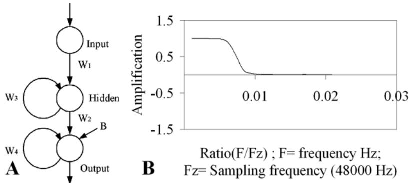
Figure 5.5: (A) The principal advanced auditory network, performing as a low-pass filter of the noisy signal with varying amplitudes. The bias term  $B$  is equal to  $-6.7$  and all weights are positive,  $W_1 = 0.01$ ,  $W_2 = 32$ ,  $W_3 = 1$  and  $W_4 = 0.27$ . (B) The characteristic curve of this network with its cutoff frequency at approximately  $400$  Hz.
