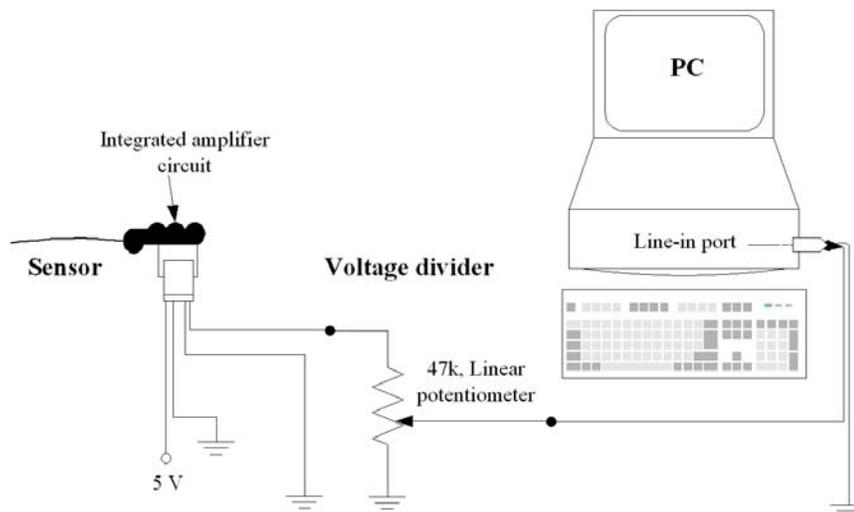
Figure 4.2: The basic schematic of the auditory-tactile sensor system. The detected signal is firstly amplified via an integrated amplifier circuit of the mini-microphone, then the amplitude of an amplified signal is reduced by a variable voltage divider. Eventually, the scaled signal goes into the line-in port for digitizing which then feeds it into the neural processor.
