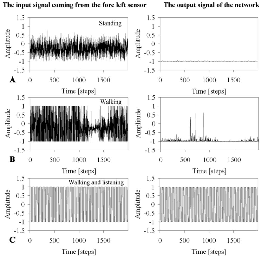
Figure 6.8: Left: The input signal coming from the fore left sensor under three different conditions. Right: The output signal of the evolved advanced auditory network with respect to the input on the left side. (A) The noisy signal when the machine was in a standing position. (B) The noisy signal during the walk. (C) The noisy signal which was compensated between the sound and a noise during the walk. All figures have the same scale in x-axis and y-axis.
