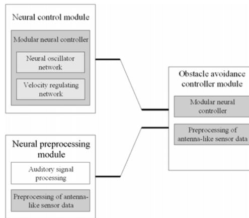
Figure 5.35: The modular architecture of the obstacle avoidance controller consists of the neural preprocessing and control modules. The preprocessing of antenna-like sensor data from the neural preprocessing module is selected and linked to the modular neural controller (of a four- or six-legged walking machine).
