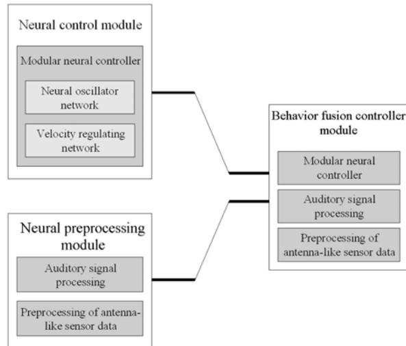
Figure 5.40: The modular architecture of the behavior fusion controller, which completes the perception-action systems, consists of the neural preprocessing and control modules. The auditory signal processing and the preprocessing of antenna-like sensor data are selected to connect to the modular neural controller (of a four- or six-legged walking machine).
