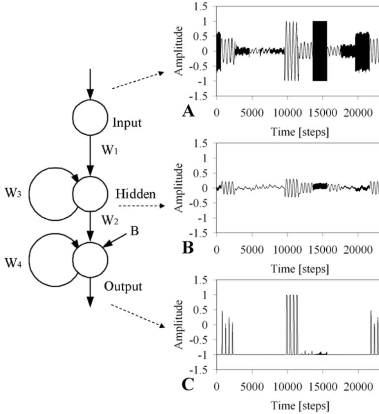
Figure 5.7: The mixed signals between low- and high-frequency sounds with varying amplitude from all neurons. (A) The signals from an input neuron. (B) The signals from a hidden neuron. (C) The signals from an output neuron.
