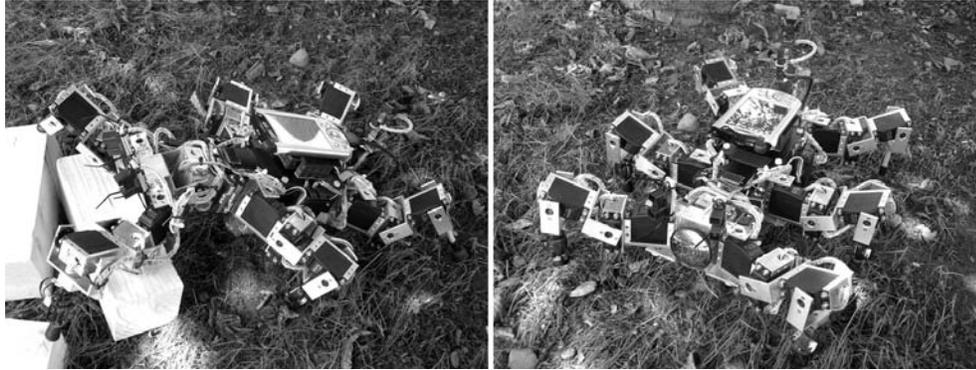
Figure A.2: The physical six-legged walking machine AMOS-WD06. Left: Top view with climbing position. Right: Front view with standing position.
