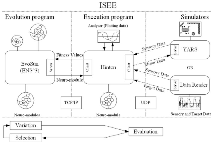
Figure 3.11: The schematic of the evolutionary process with the ISEE modified from B. Mahn 2003, pp. 32 [91] (see text for details).
