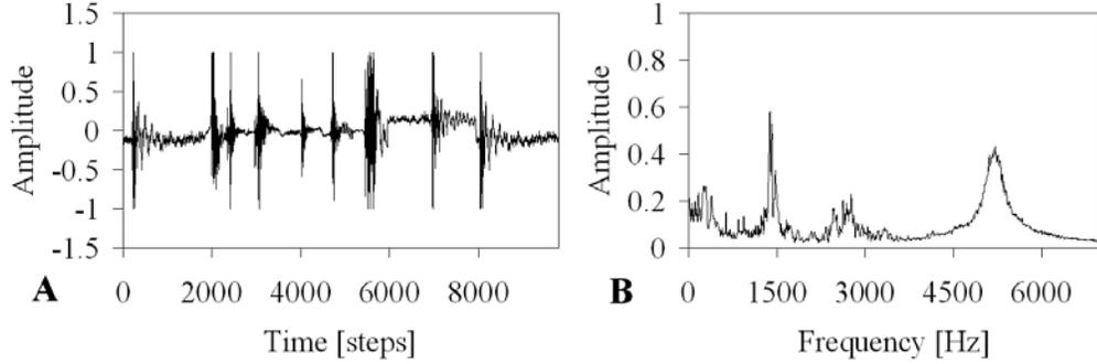
Figure 5.15: (A) The oscillating peaks are the tactile signal coming from the auditory-tactile sensor. (B) The FFT spectrum displays the compound frequency of the signal. By observing the compound frequency, the first and the second resonance frequencies appear at around 1400 Hz and 5200 Hz.
