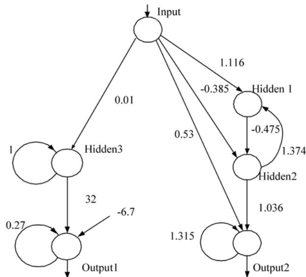
Figure 5.19: The auditory-tactile signal processing network recognizes low-frequency sound up to 400 Hz ( $O_1$ ), and the described tactile signal ( $O_2$ ). It is developed to operate at the update frequency of 48 kHz.
