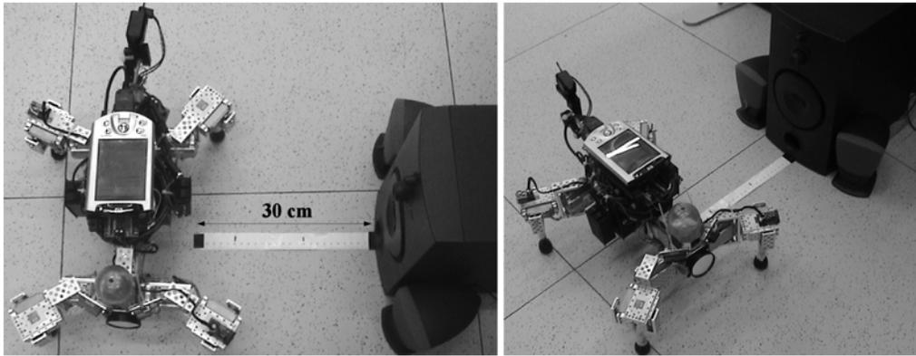
Figure 6.7: The walking machine AMOS-WD02 was initially placed in front of a loudspeaker at a distance of 30 cm to test the effect of motor noise while it was walking and listening to the sound at the same time.
