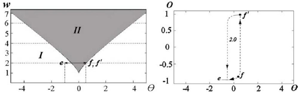
Figure 3.9: The example of the dynamics of the recurrent neuron with the dynamic input. Left: The dynamic input  $\theta$  varies between  $\approx -1$  which is in region  $I$  and  $\approx 0.5$  which is near to the border where the system can jump from one fixed point (low) to another fixed point (high). Right: The hysteresis effect of the dynamic input for a fixed  $w = 2$ , see text for details, (modified from F. Pasemann 2005 [116]).
