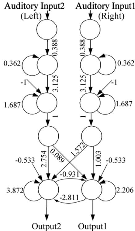
Figure 5.14: The auditory signal processing network which functions as a low-pass filter circuit and which has an ability to detect the directionality of the corresponding signals. The network is developed to operate at an update frequency of approximately 2 kHz.
