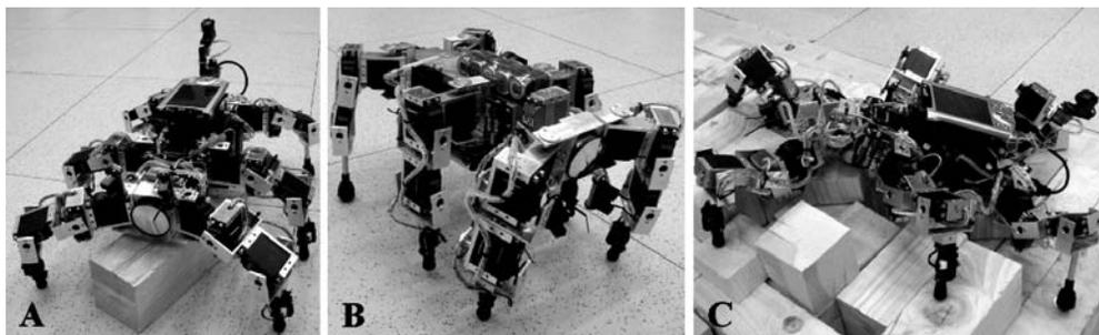
Figure 4.18: The walking machine AMOS-WD06 walking over an obstacle with the maximum height of 7 cm (A), standing in an upside-down position (B) and climbing over obstacles (C).
