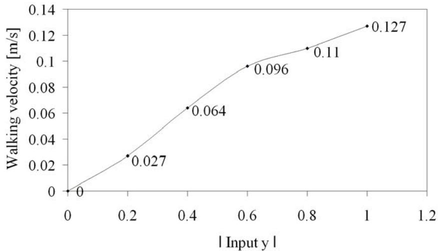
Figure 5.32: Comparison of the walking velocity with different input  $y$  of the VRN.
