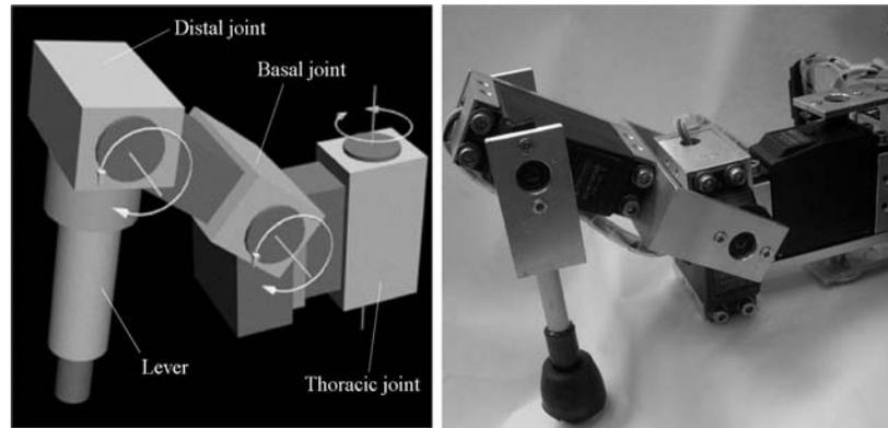
Figure 4.17: The leg with three DOF. Left: The 3D model of the leg. Right: The physical leg of the AMOS-WD06.
