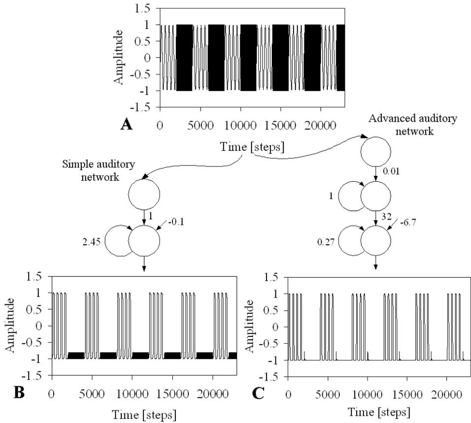
Figure 6.1: (A) The simulated input consisting of two different frequencies (100 Hz and 1000 Hz). (B) The corresponding output of the simple auditory network. (C) The corresponding output of the principal advanced auditory network. All figures have the same scale in x-axis and y-axis.
