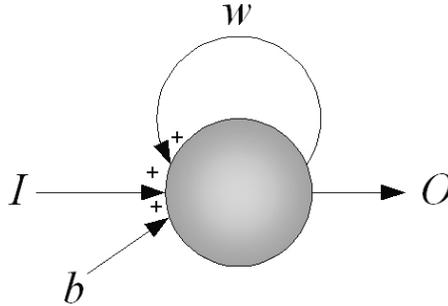
Figure 3.6: The model neuron with a self-connection.
