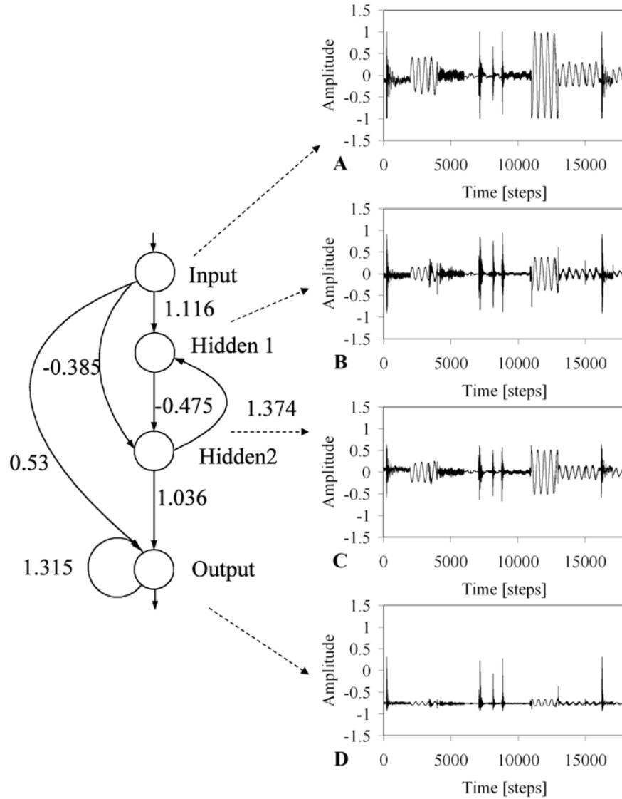
Figure 5.18: The mixed signals between low-frequency sound (100 Hz) and the tactile signal from all neurons. (A) The signals from an input neuron. (B), (C) The signals from hidden neurons. (D) The signals from an output neuron.
