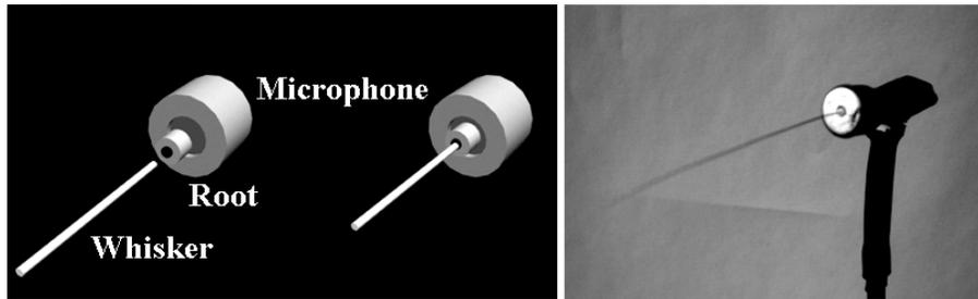
Figure 4.1: The auditory-tactile sensor consists of a whisker of a real mouse, a rubber root and a capacitor microphone built in an integrated amplifier circuit. Left: Assembly parts of a sensor. Right: The real sensor built in an amplifier circuit.
