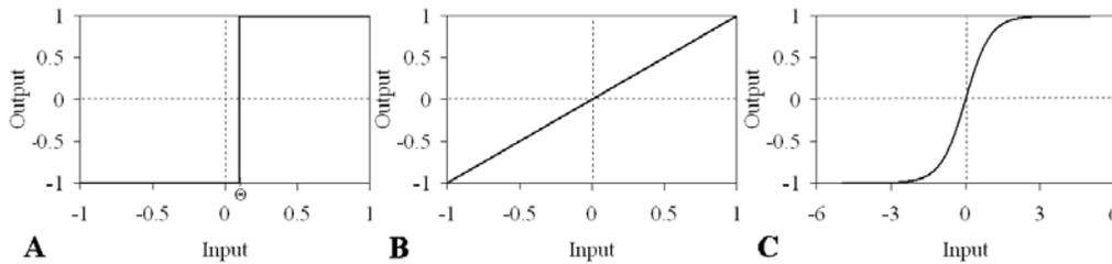
Figure 3.4: Most widely used transfer functions. (A) Linear threshold transfer function. (B) Linear transfer function. (C) Nonlinear sigmoid transfer function.
