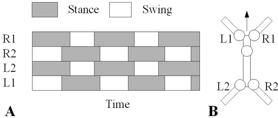
Figure 5.28: (A) The typical trot gait. X-axis represents time and y-axis represents the legs. During the swing phase (white blocks) the feet have no ground contact. During the stance phase (gray blocks) the feet touch the ground. (B) The orientation of the legs of the AMOS-WD02.
