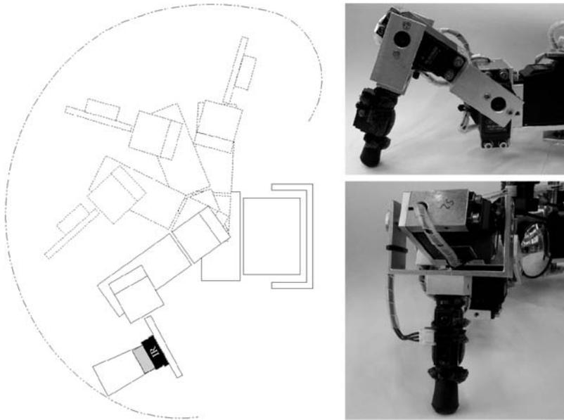
Figure 4.10: Left: The idealized field of the antenna-like sensor on the right foreleg of the six-legged walking machine (dashed curve) with the remaining sensors operating on the other legs. The sensor moves in a vertical direction when the basal and distal joints are activated. Right: The physical sensor on the right foreleg.
