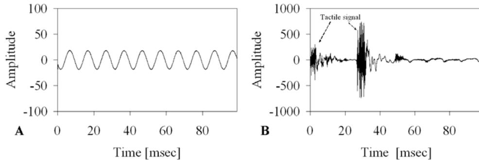
Figure 4.3: (A) The response of the auditory-tactile sensor to an auditory signal at a frequency of 100 Hz which is generated by a loudspeaker. (B) The response of the sensor to a tactile signal which is generated by sweeping the sensor over an object back and forth. All figures have the same scale in x-axis while y-axis is different.
