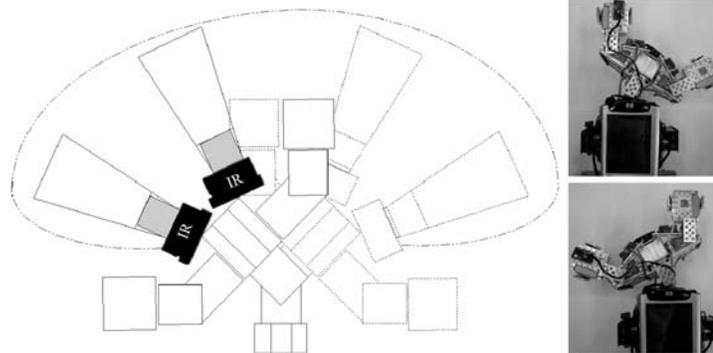
Figure 4.8: The idealized field of the antenna-like sensors when the backbone joint of the walking machine is activated. Left: The outline of the idealized field where the sensors can scan obstacles (dashed curve). Right: The visualization of the sensors moving with the head of the walking machine when the backbone joint turns right (upper picture) and left (lower picture).
