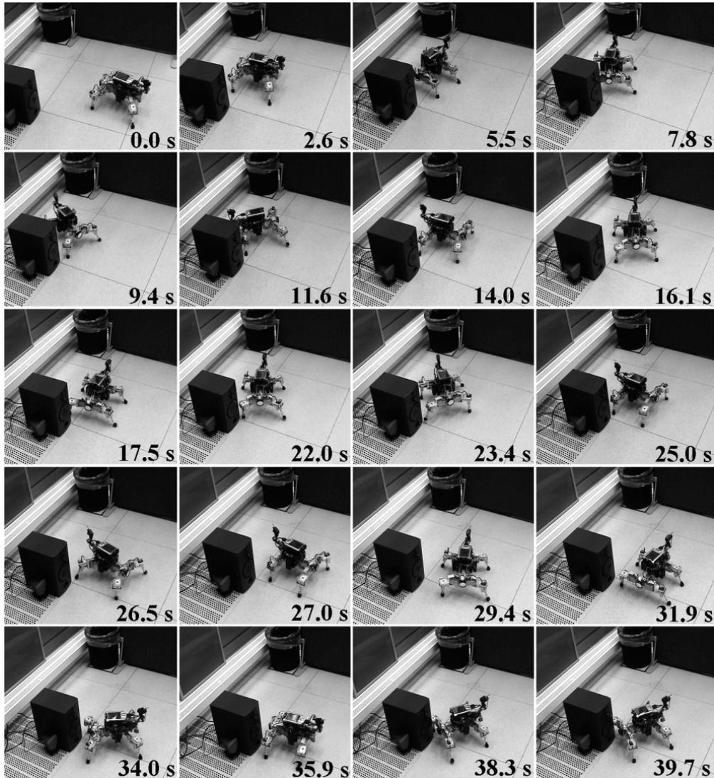
Figure 6.26: The example of the sound tropism where the sound source was initially in front of the walking machine and was generated during the walk. In this situation, the walking machine also behaved like the previous example. It walked forward and then turned into the direction of the sound source when the sound was detected. After that, it approached and stopped beside the sound source.
