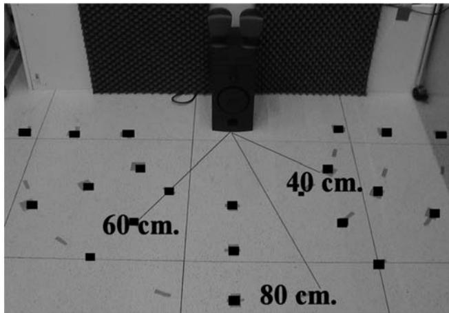
Figure 6.21: The experimental set-up with the sound source and the markers (black square areas) where the walking machine was placed.
