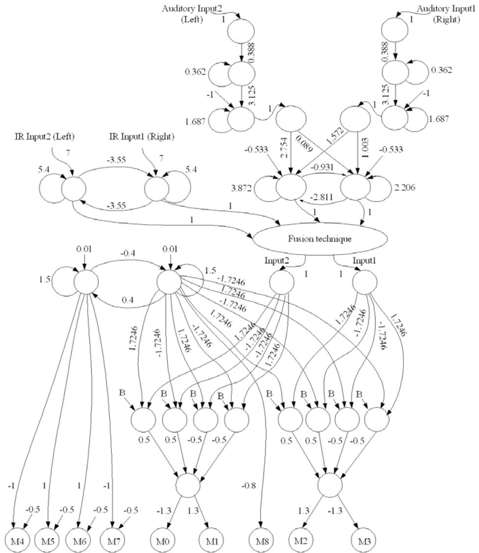
Figure 5.43: The behavior fusion controller for generating the different reactive behaviors of the four-legged walking machine.
