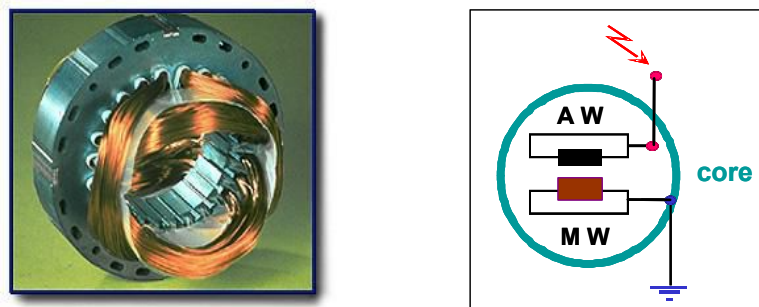
Fig. 2.7: Stator windings of a small motor and a schematic representation of the electrical connection
