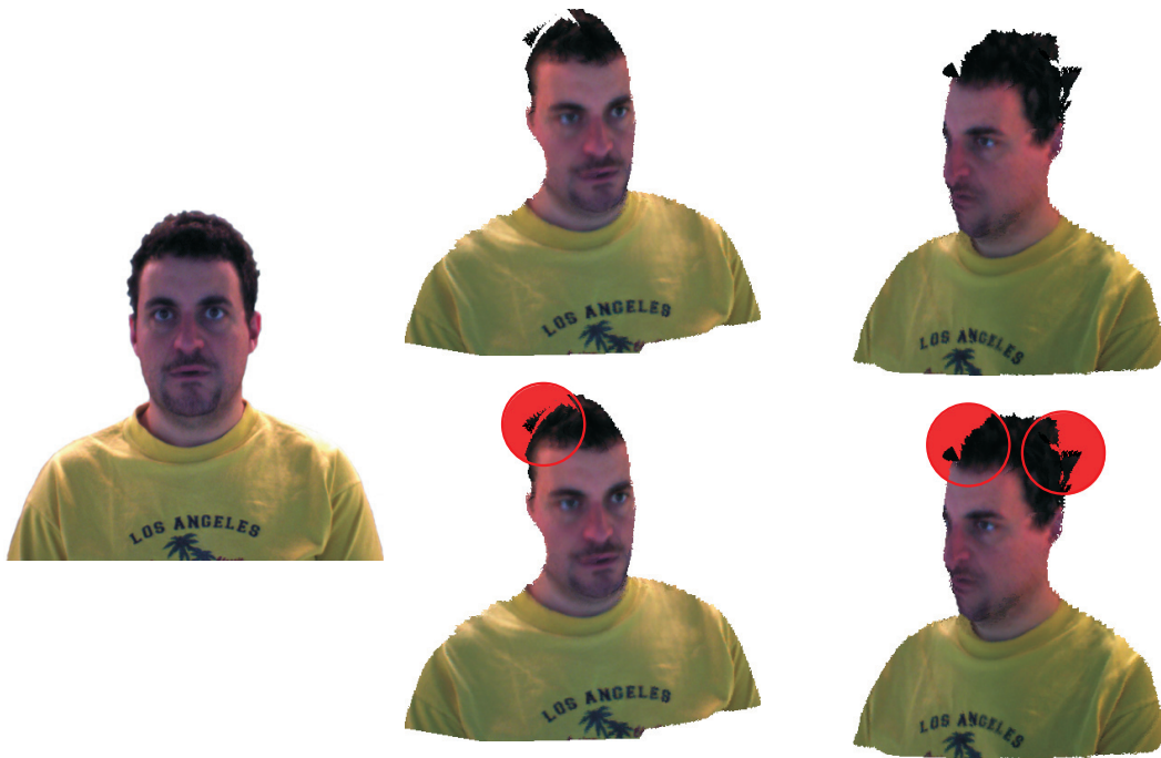
Figure 5.9: Light field being captured from Christof Rezk Salama. Discontinuity artifacts appear in regions of infrared light being absorbed during acquisition. Left: RGB input image with the background being culled. Middle and Right: Light field rendering with the discontinuity artifacts being highlighted in the bottom row.
