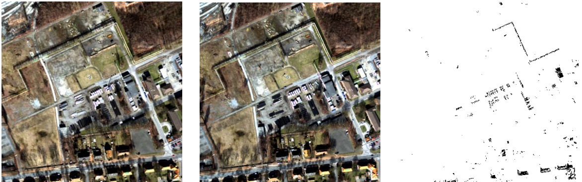
Figure 1.3: Example of target detection in multi temporal images contribution. Images from left to right: original Daedalus image at time 1; original Daedalus image at time 2; map of changes between images.
