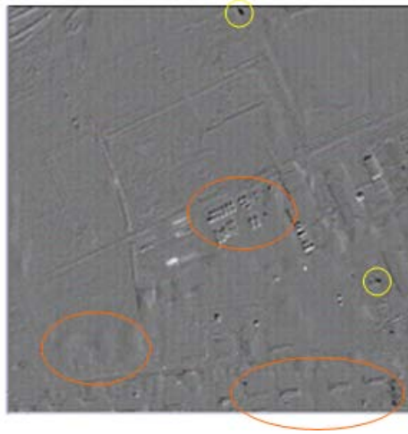
Figure 5.4: Detected targets (yellow) and false alarms (red) obtained by applying the MAD transformation.
