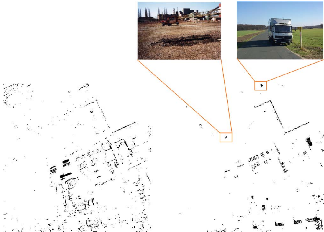
Figure 10.2: Image on the left side shows the synergy of TSAD map and CNG applied to Dorsten site; Image on the right side displays the synergy of NDVI map and CNG over Dorsten scene. The top row images show the ground truth of two detected targets.
