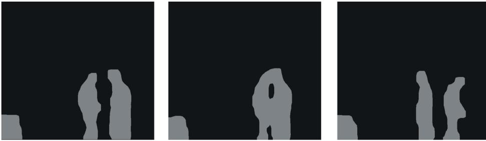
Figure 4.9: Left: Before occlusion, the number of detected objects= 3. Middle: Partial occlusion happening, number of detected objects= 2 and the change of area size of one of the objects (occluded objects) is bigger than the predefined threshold. Right: After occlusion, two objects split, the number of detected objects increases to 3 and the size of detected objects (split ones) reduce dramatically.
