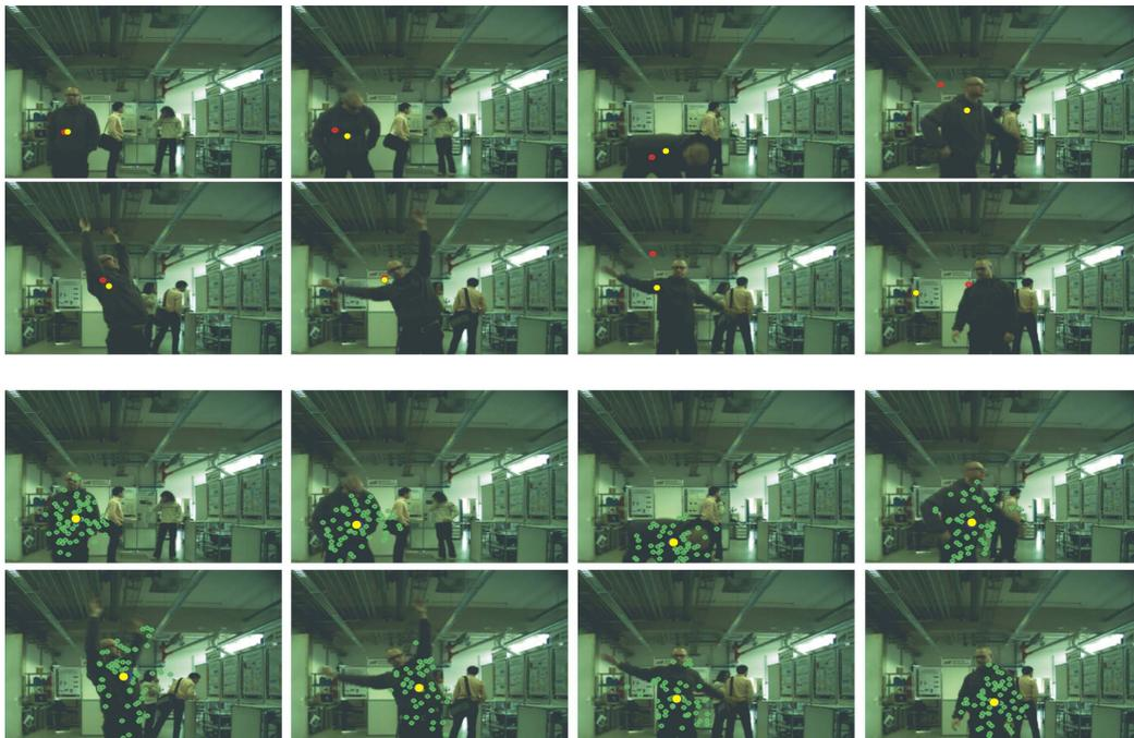
Figure 4.19: Some results of person tracking using the Kalman filter and the CONDENSATION technique (frame number 25, 40, 70, 85, 120, 230, 280, 355). First two rows represent the Kalman filter results. Red point shows the predicted (intermediate) position and yellow shows the corrected point (final result). Last two rows represent the CONDENSATION result where the particles are depicted in green and the mean of all (final result) is in yellow.
