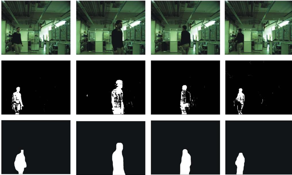
*Figure 4.1: Some results of background subtraction under normal lighting conditions. First row: Original 2D images, frames number 55, 105, 160, 220 and 260. Second row: Corresponding foreground images derived using the adaptive Gaussian mixture model technique on the 2D images. Third row: Corresponding foreground images derived using range thresholding and the connected components technique from corresponding 3D images.*
