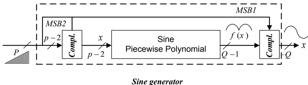
Figure 6.2: Quadrant compression architecture for single phase chirp generator
