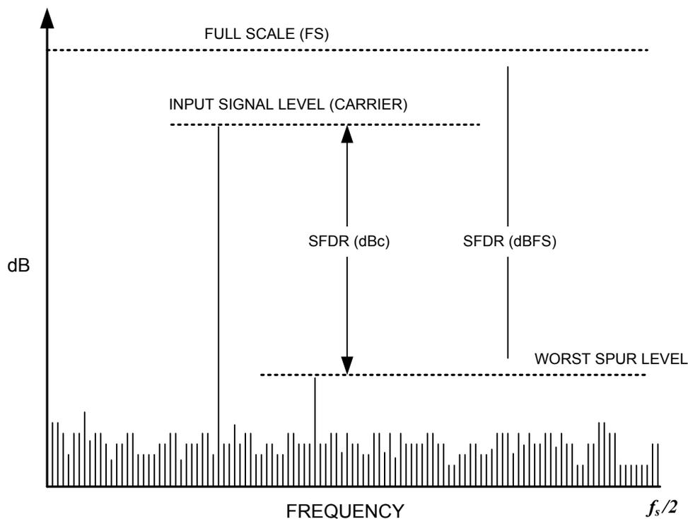
Figure 6.8: Measure of Spurious Free Dynamic Range (SFDR), as measured in [37]
