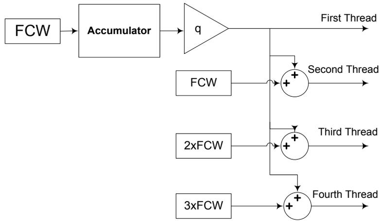
Figure 7.18: Simplified block diagram for the throughput at each thread
