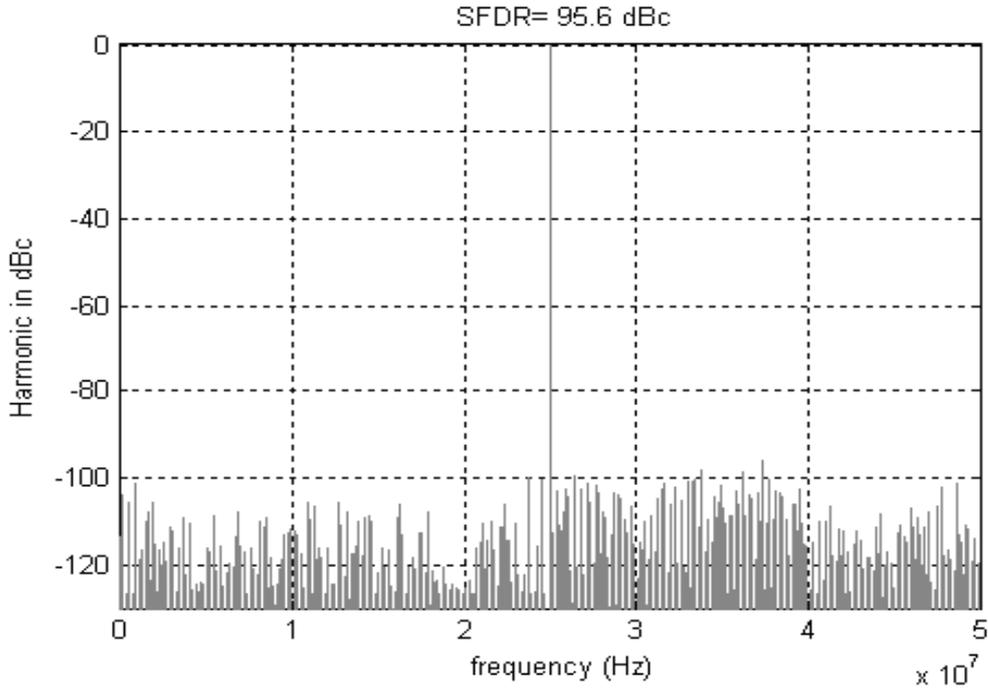
Figure 6.9: Output spectrum with 16 sections/quad
