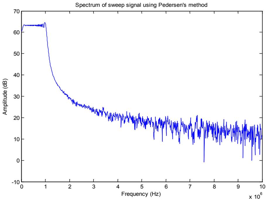
Figure 6.19: Output spectrum of the chirp signal using Pedersen's method
