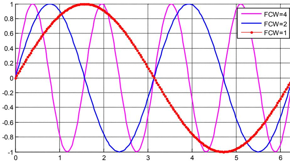
Figure 4.2: Effect of FCW values on output sine wave.
