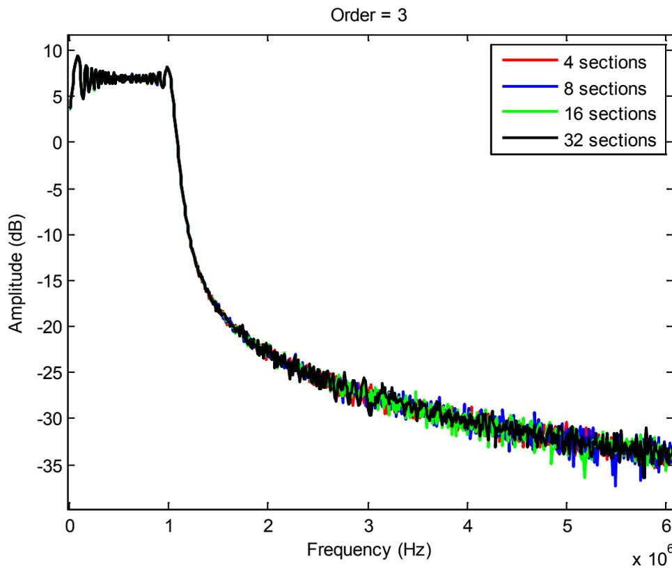
Figure 6.24: Signal spectra in the case of third order interpolation equation and different number of sections/quadrant
