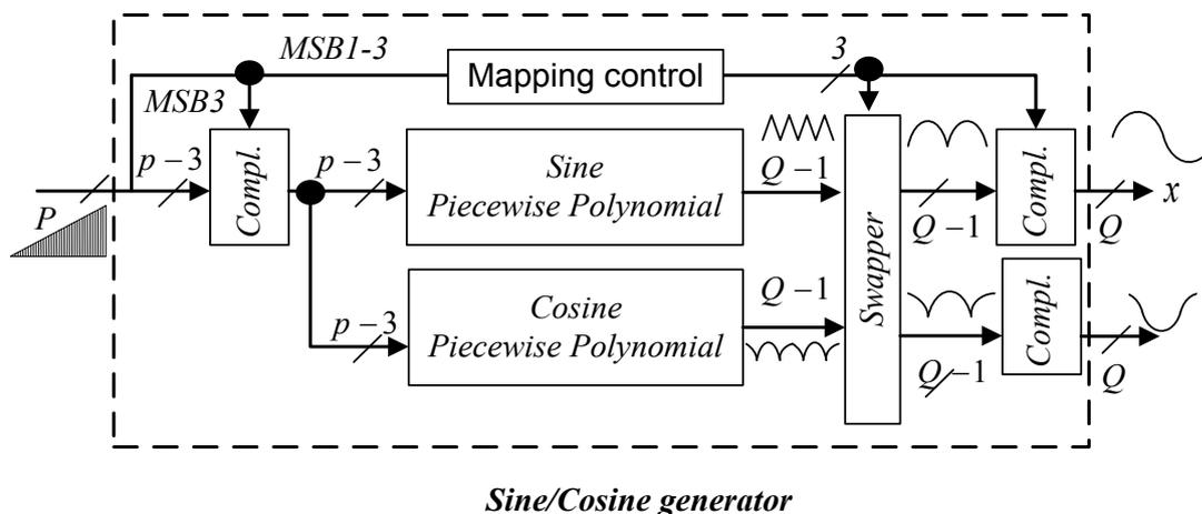
Figure 6.3: Quadrant compression architecture for quadrature phase chirp generator
