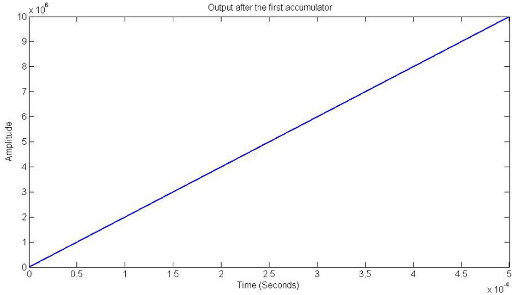
Figure 6.13: The output after the counter or the first accumulator
