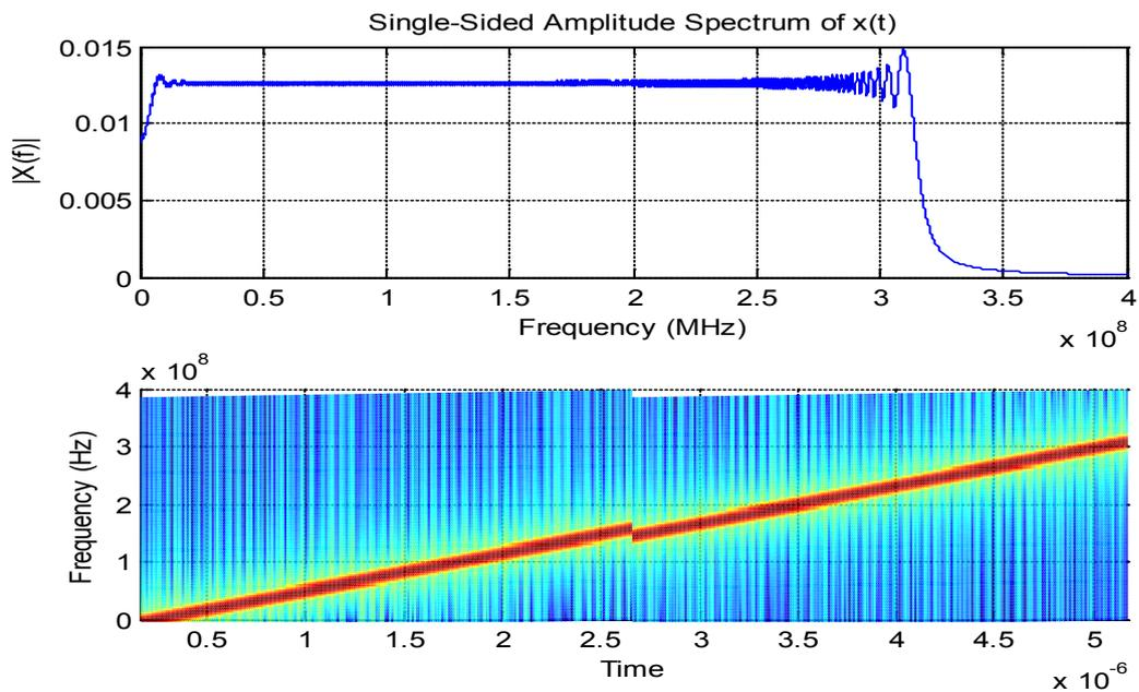
Figure 7.24: A 320 MHz digital chirp signal using the proposed method: (a) single sided amplitude spectrum, (b) The energy spectrogram
