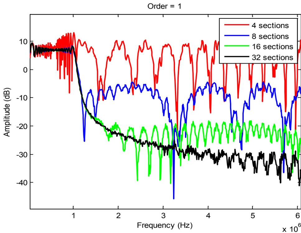
Figure 6.21: Signal spectra in the case of linear interpolation with different number of sections/quadrant
