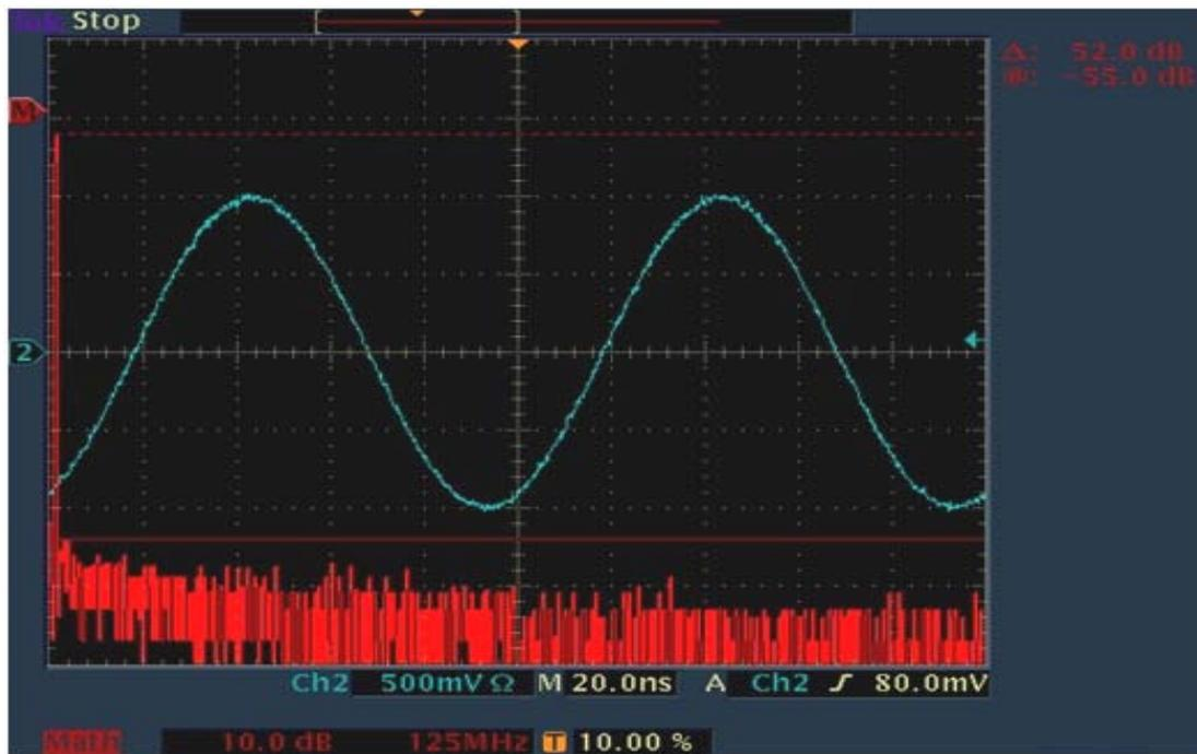
Figure 7.21: Spurious Free Dynamic Range (SFDR) of the generated signal with 125 MHz.
