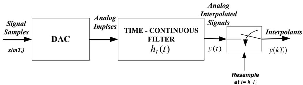
Figure 6.4: Rate conversion with time-continuous filter
