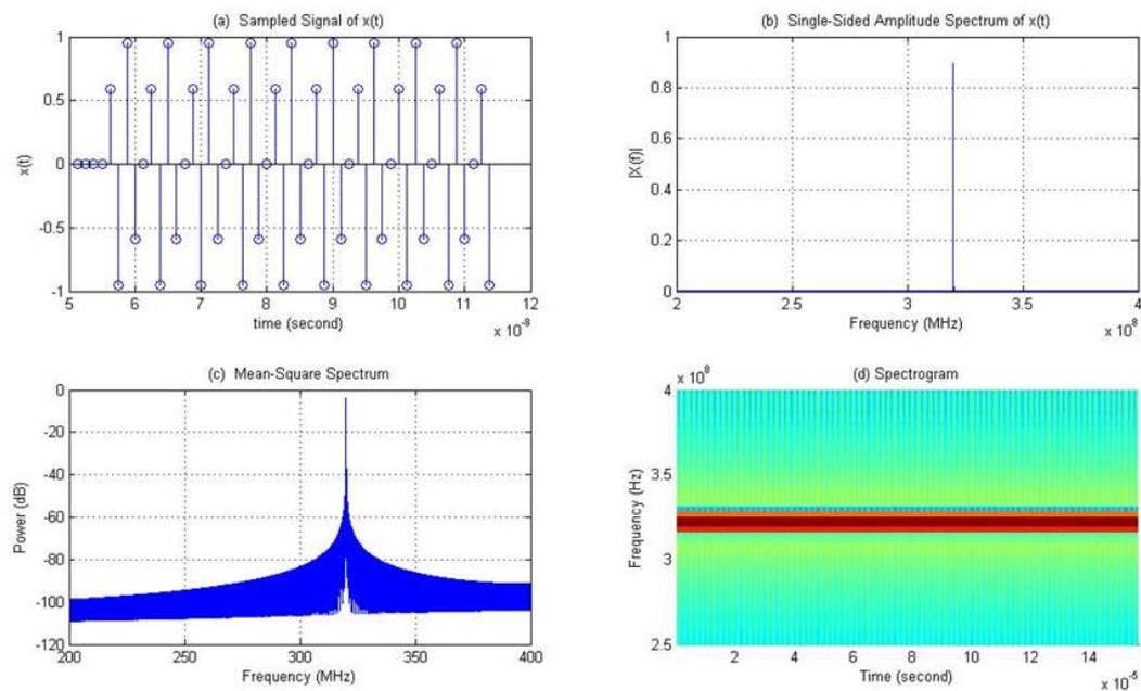
Figure 7.20: The generated single tune signal with 320 MHz. (a) Sampled Signal (b) Single-Sided Amplitude Spectrum (c) Mean Square Spectrum (d) The spectrogram
