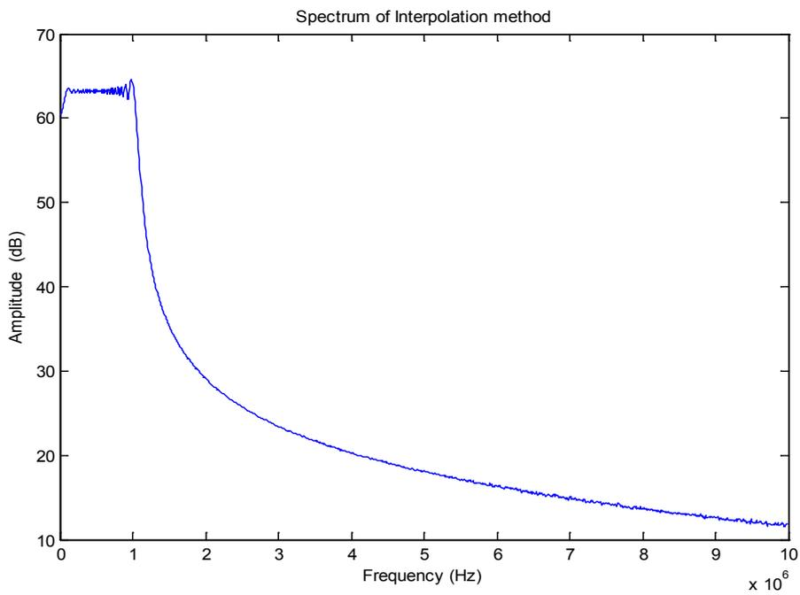
Figure 6.20: Spectrum of the chirp signal using the interpolation method
