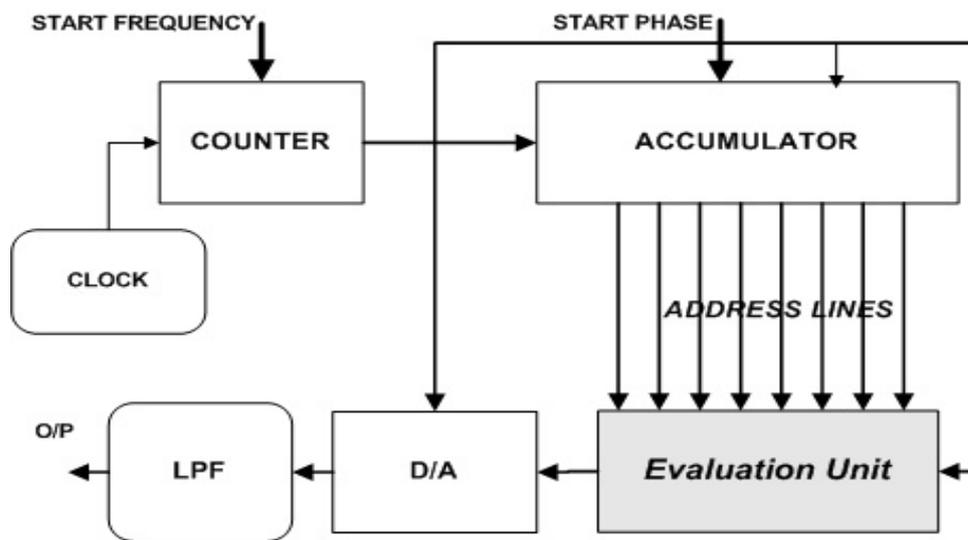
Figure 6.12: Block diagram of the proposed digital chirp generator
