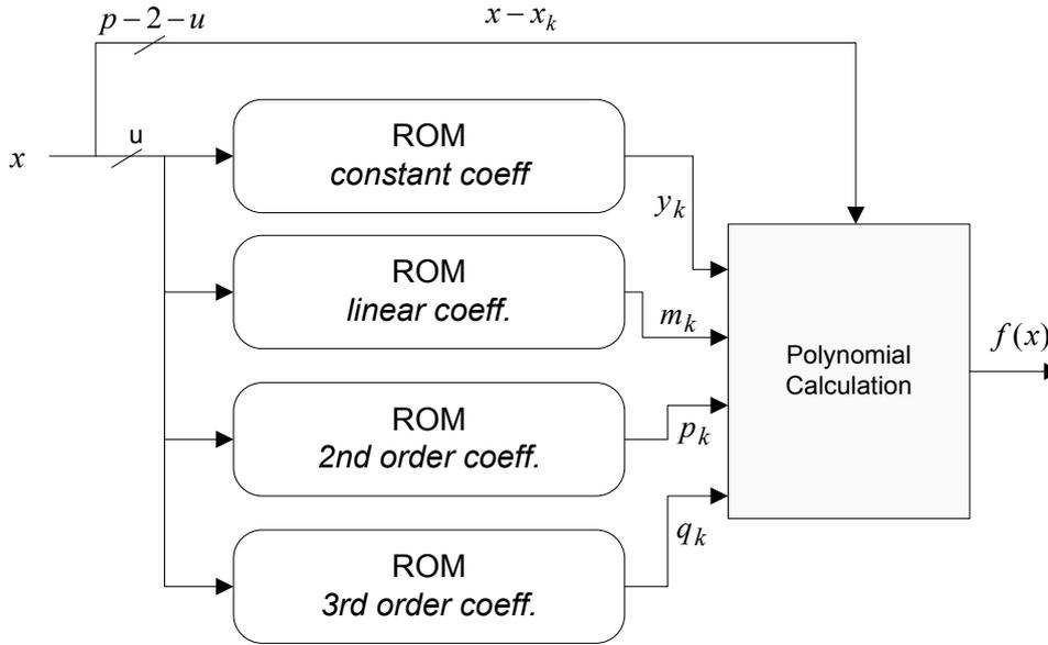
Figure 6.7: Piecewise-polynomial interpolation of sine function in  $[0, \pi / 2]$  for a third-order approximation
