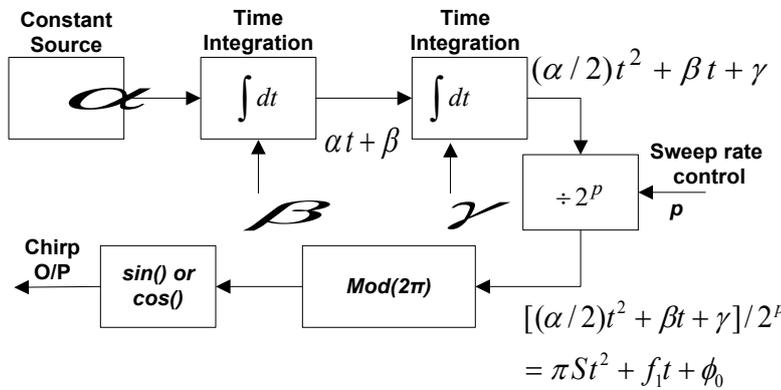
Figure 3.1: Functional block diagram of the digital chirp generator
