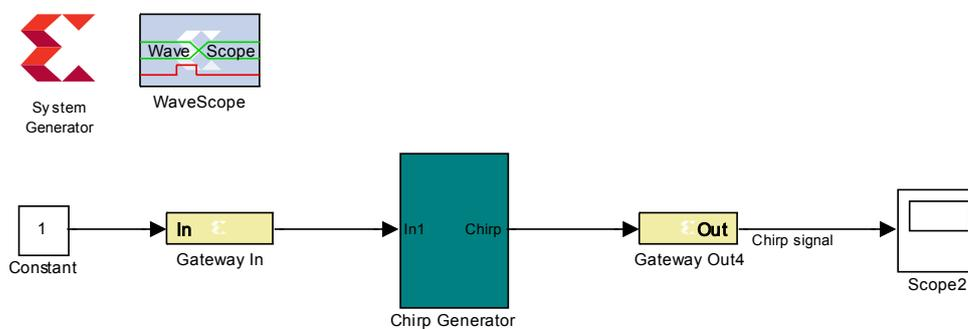
Figure 7.14: The complete FPGA design of the chirp generator
