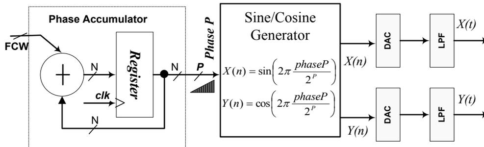
Figure 4.1: Simplified schematic of a quadrature DDFS
