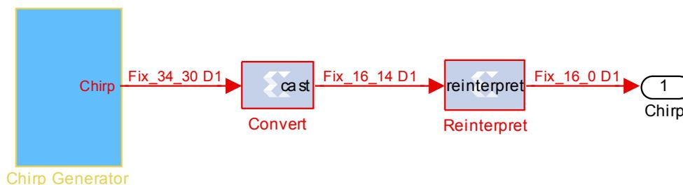
Figure 7.15: The block diagram of converting the data in order to fit the DAC
