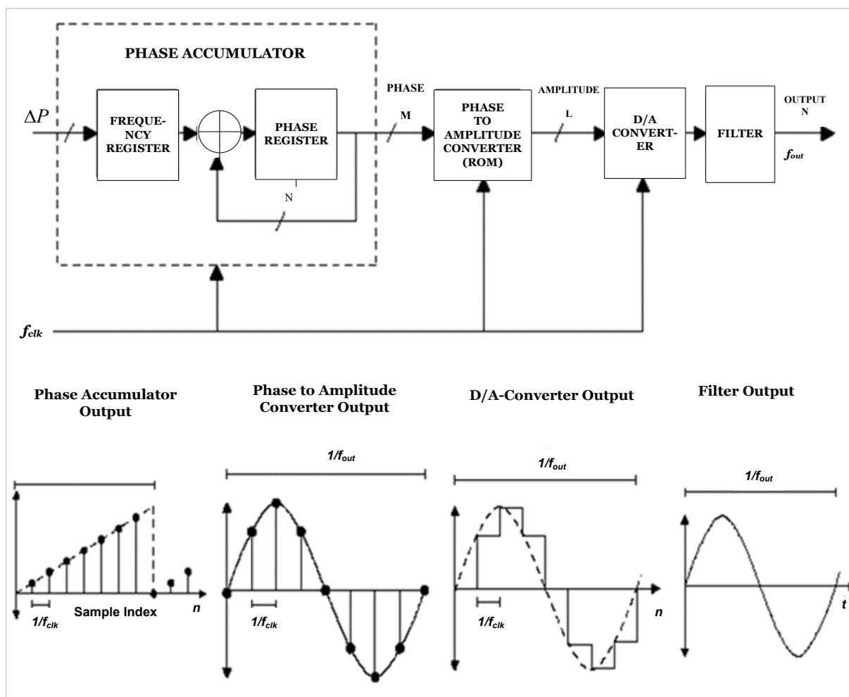
Figure 4.4: General structure of a practically realizable DDFS.
