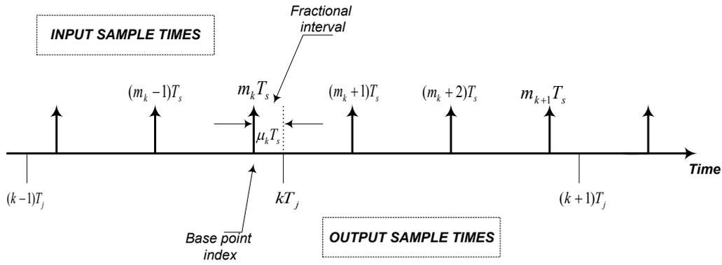
Figure 6.5: Base point pivoting
