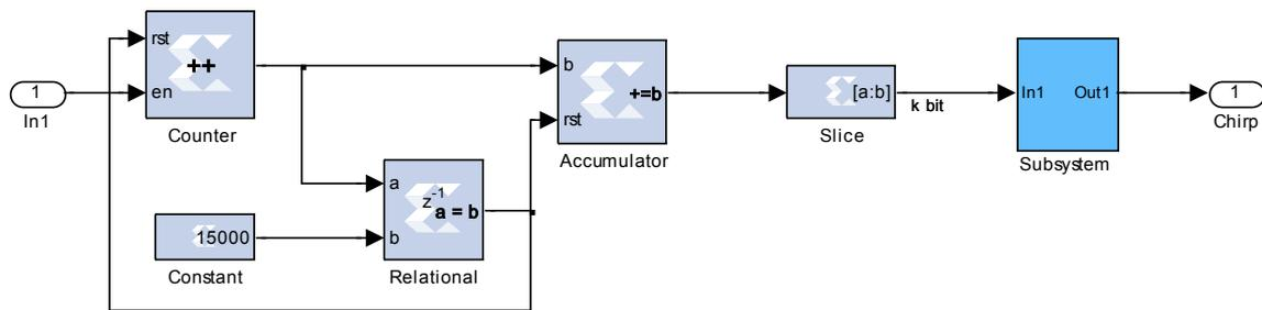
Figure 7.10: Equivalent FPGA implementation of the Simulink model of Figure 7.9
