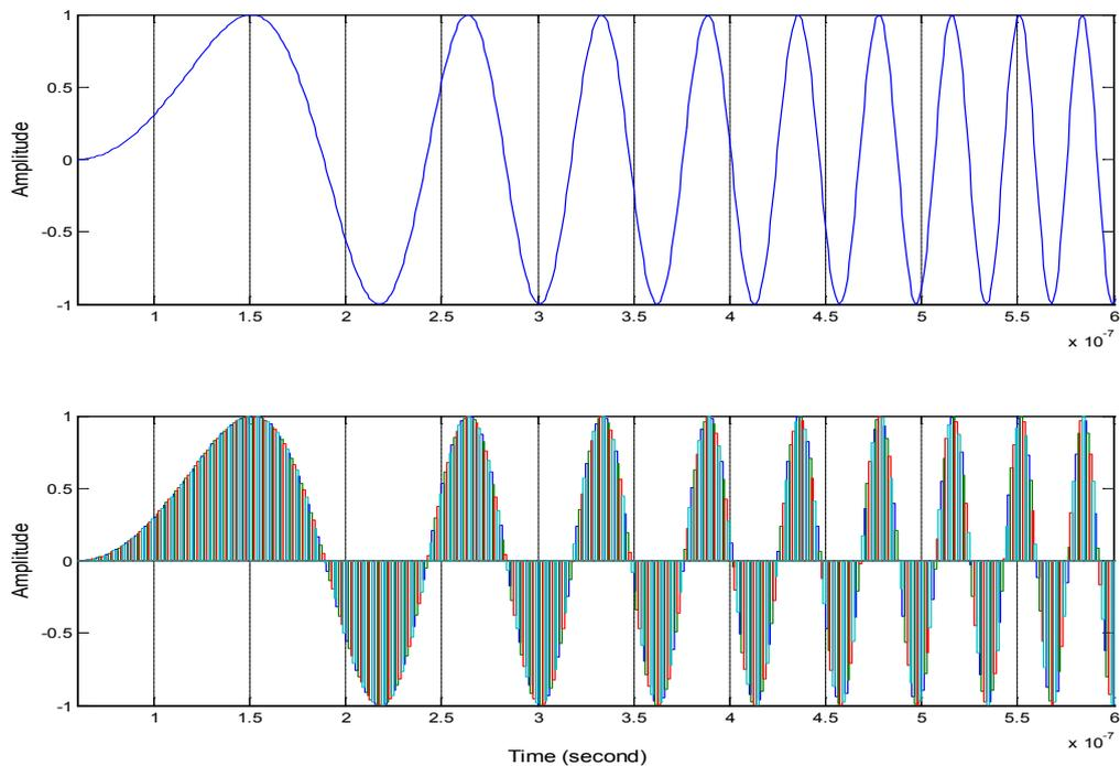
Figure 7.23: The generated chirp signal using 4 threads parallel processing technique and the interpolation methodology.
