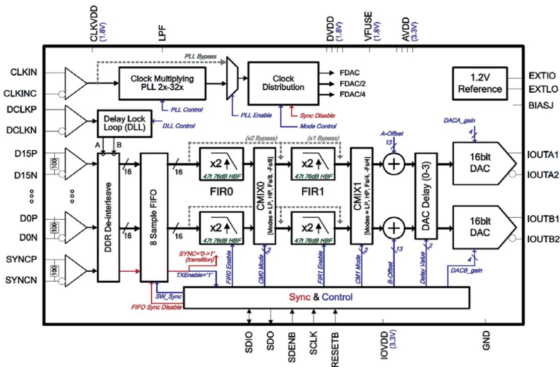
Figure 7.3: DAC functional block diagram
