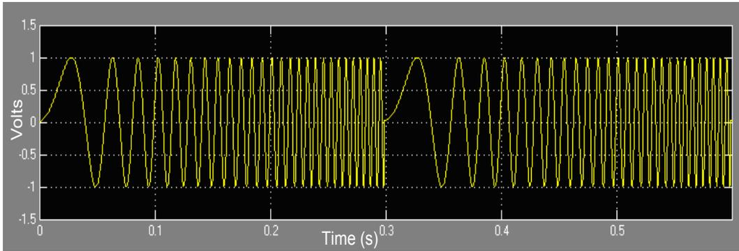
Figure 6.23: The generated coherent swept signal by the new technique (2 periods)
