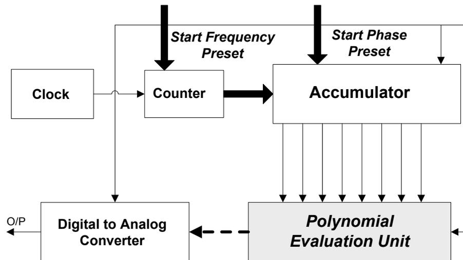
Figure 6.1: Block diagram of the proposed digital chirp generator
