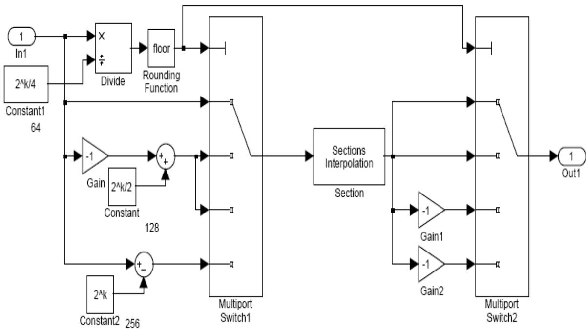
Figure 6.16: The block diagram of the simulated structure works as Farrow structure to generate the sine wave
