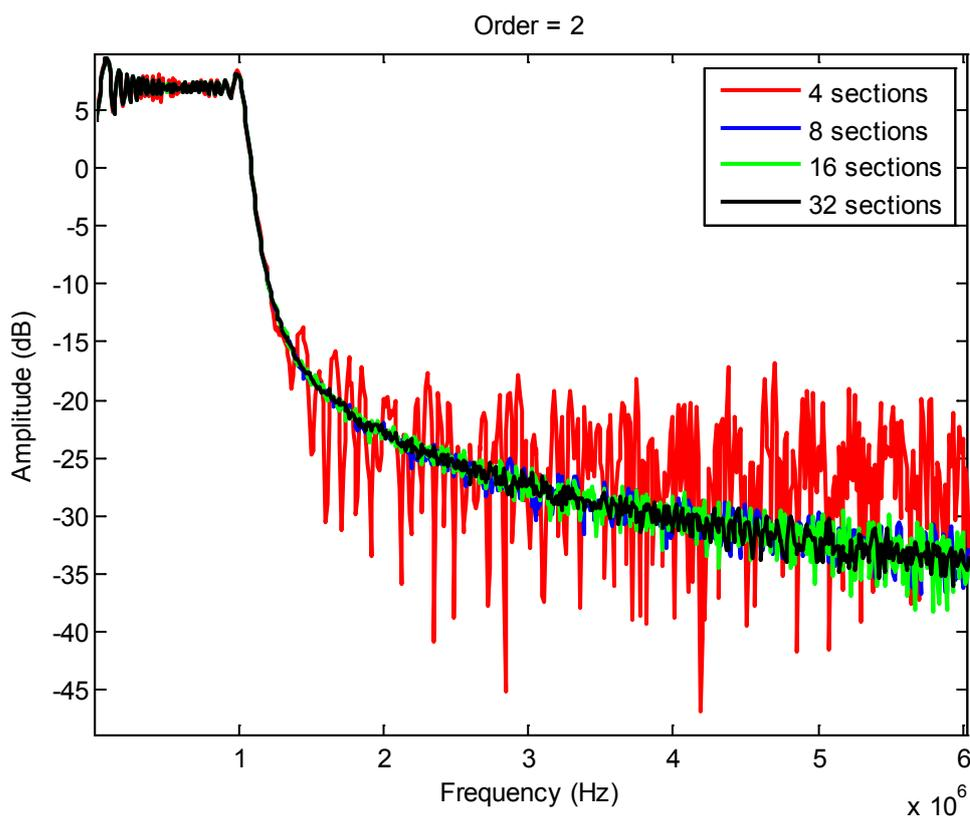
Figure 6.22: Signal spectra in the case of piecewise parabolic interpolation with different number of sections/quadrant.
