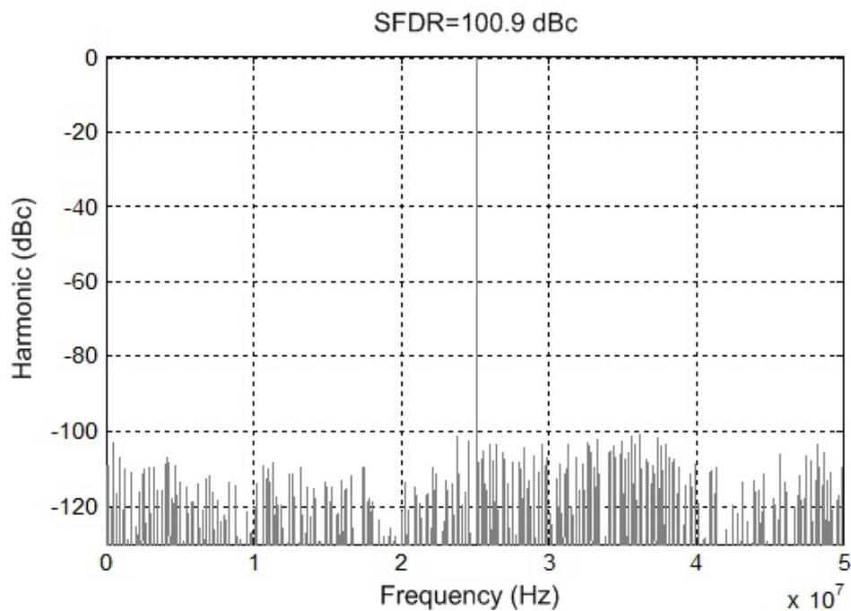
Figure 6.11: Output spectrum for 32 sections per quadrant with optimized parabolic approximation.
