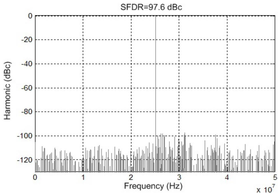
Figure 6.10: Output spectrum for 32 sections per quadrant with non-optimized parabolic approximation
