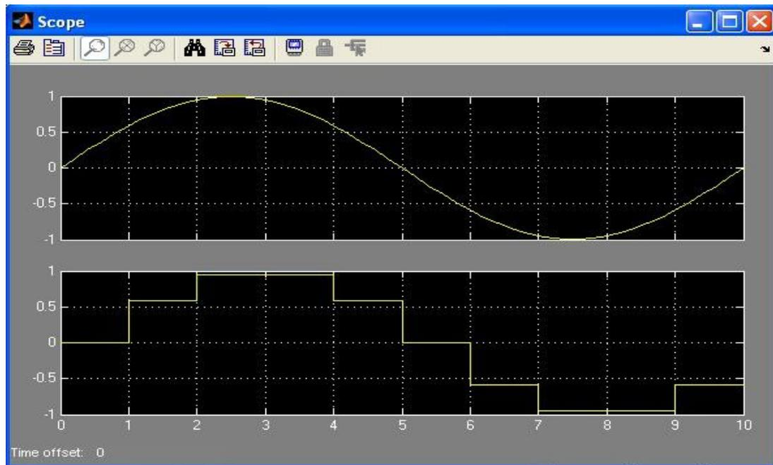
Figure 7.7: unaltered and sampled versions of the sine wave
