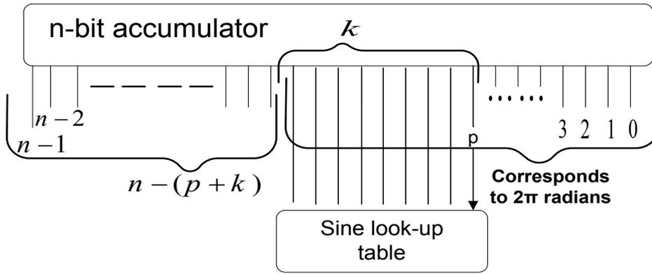
Figure 3.3: Definition of the output lines from the accumulator
