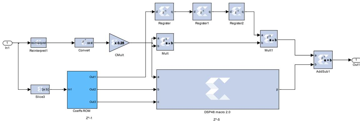
Figure 7.12: The FPGA implementation of the interpolation algorithm
