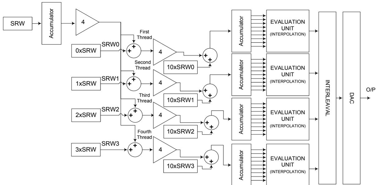
Figure 7.22: The generation of the digital chirp signal using 4 threads parallel processing structure and the interpolation methodology
