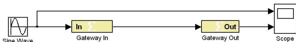
Figure 7.6: A simple System Generator model
