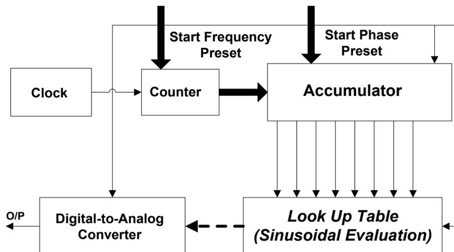
Figure 3.2: Simplified Block diagram of the implementation of the digital sweep generator
