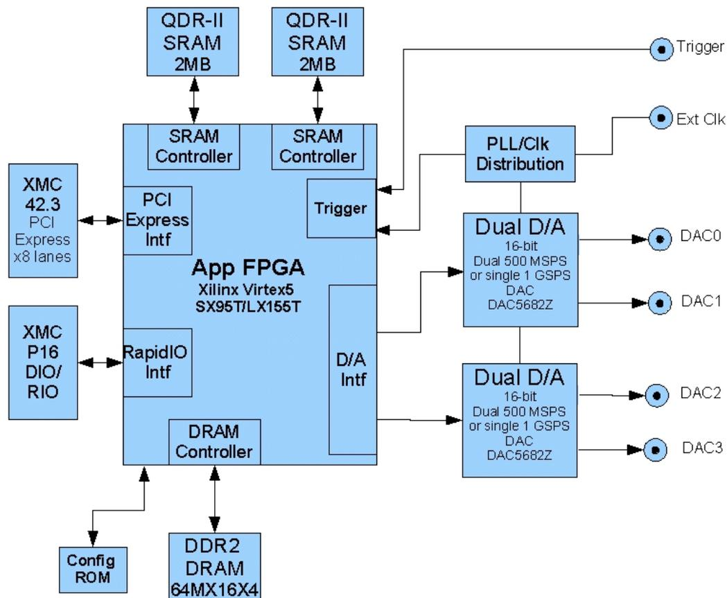
Figure 7.2: X5-TX Block Diagram
