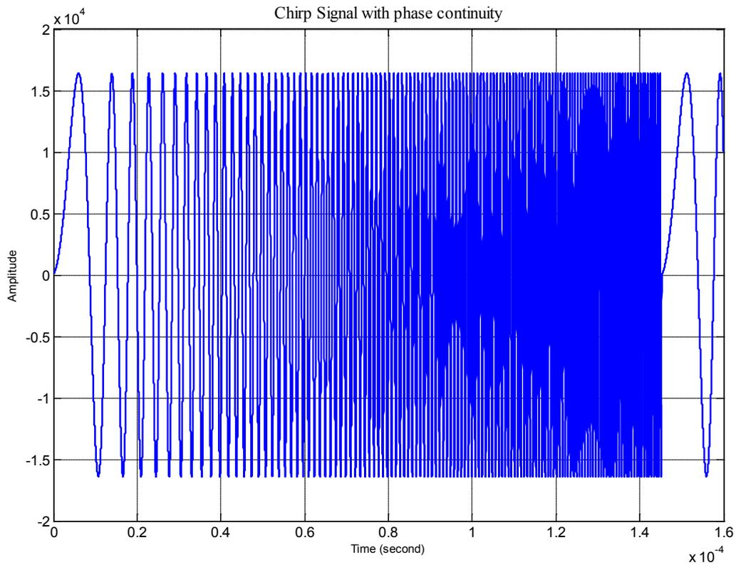
Figure 7.16: The generated chirp signal based on the proposed method and using the FPGA technology
