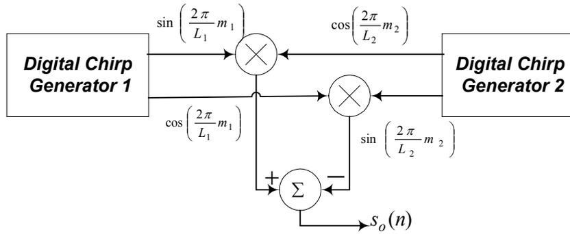
Figure 3.4: Schematic diagram of the fractional bit digital chirp generator structure
