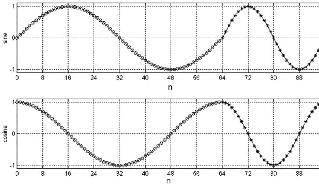
Figure 4.3: Sine and cosine DDFS outputs generated from the PA outputs
