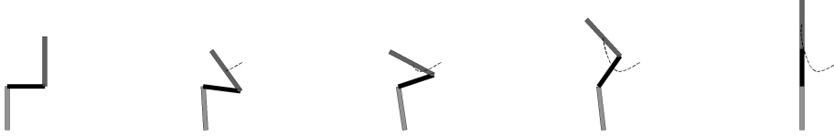
Figure 6.3.: Optimal control of a 3-link manipulator with linear viscous friction ( N = 20 ): Snapshots for the optimal movement at t \in \{0, 0.75, 1.5, 2.25, 3\} for REM.
