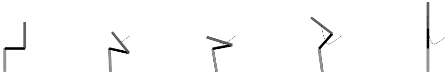
Figure 7.4.: Optimal control of a 3-link manipulator ( N = 20 ): Snapshots for the optimal movement at t \in \{0, 0.75, 1.5, 2.25, 3\} for BEM.
