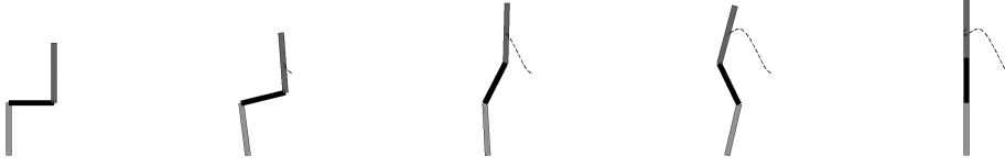
Figure 6.2.: Optimal control of a 3-link manipulator with limited control ( N = 20 ): Snapshots for the optimal movement at t \in \{0, 0.75, 1.5, 2.25, 3\} for REM.
