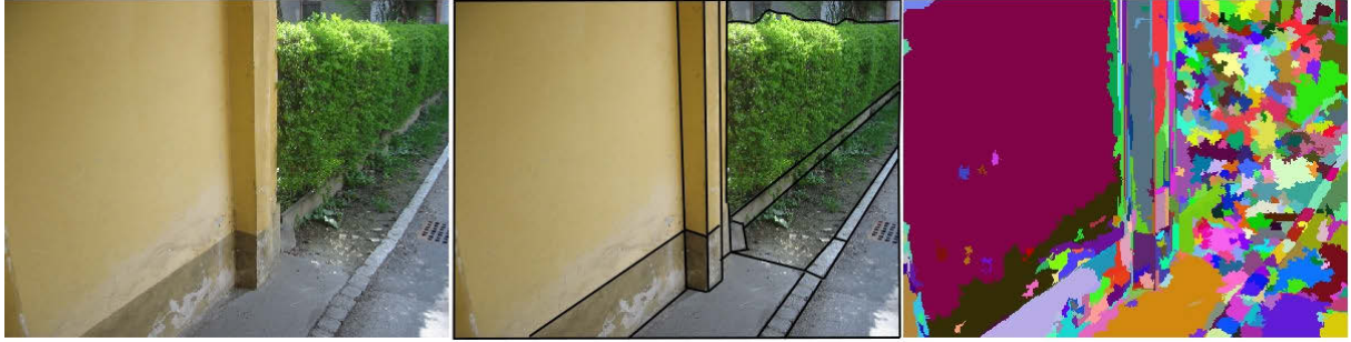
Figure 2.12: Left: An image of a scene. Middle: Simple cuts to construct 3D scene from one single 2D image. Right: over-segmented image where each small region (superpixel) lies on a plane in the 3D world.
