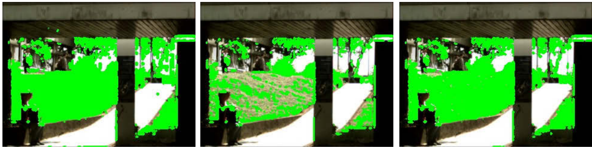
Left: The threshold is too low. Middle: the threshold is too high. Right: output from the algorithm.
