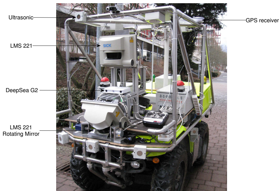
Figure 2.3: Autonomous mobile robot with TYZX DeepSea Camera mounted at the front for 3D scene visualisation.
