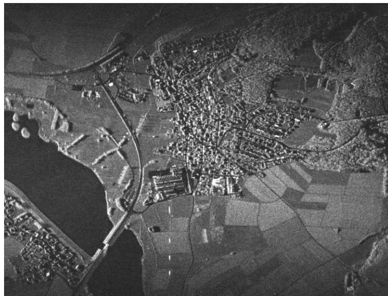
Figure 41: Focusing Result of Hybrid Experiment (Niederweidbach) using Frequency Domain Focusing Algorithm
