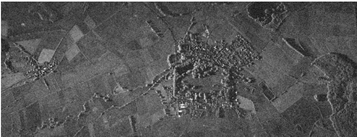
Figure 37: Focusing Result of Hybrid Experiment (Pommersfelden) using Back Projection Algorithm
