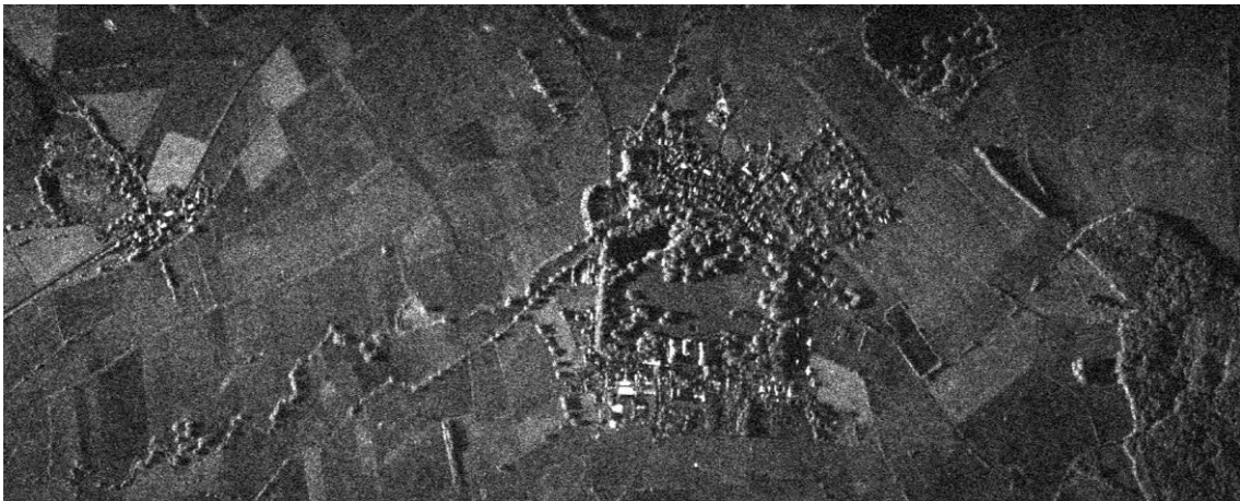
Figure 36: Focusing Result of Hybrid Experiment (Pommersfelden) using Frequency Domain Focusing Algorithm
