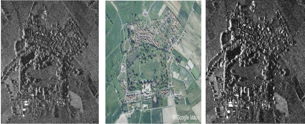
Figure 38: Comparison of Castle (Weißenstein) Image (Left) Back Projection Algorithm (Middle) Google Maps (Right) Frequency Domain Focusing Algorithm.
