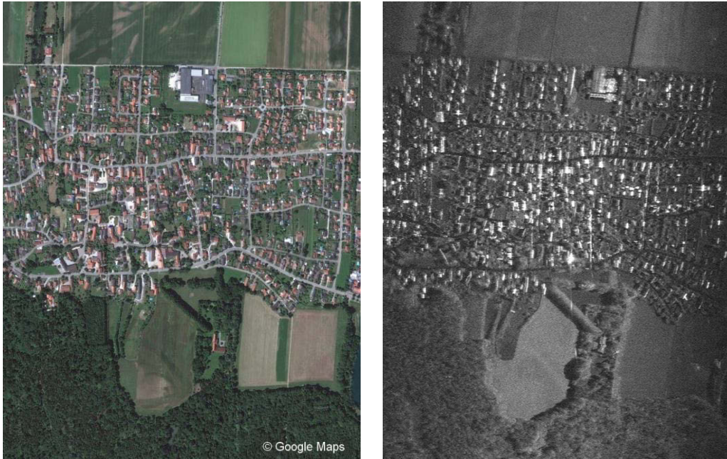
Figure 35: Focusing Results of Bistatic Azimuth Invariant Configurations: [Left] Optical Image (Google Maps), [Right] Bistatic SAR Image using a SIFT
