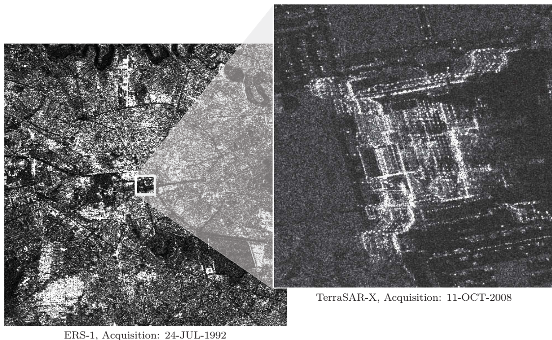
Figure 3.2: Example of the tremendous increase in details with growing resolution. ERS image of a part of the city of Bucharest (Romania) at a resolution of 25 meter ( 512 \times 512 pixels), (inset) TerraSAR-X image at a resolution of \approx 1 meter ( 512 \times 512 pixels) of the area marked by the white-rectangle in (left). Both of the images are shown at the same scale in comparison to the respective resolution.
