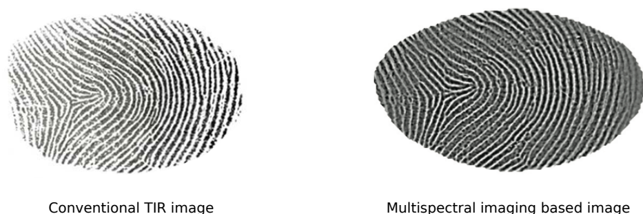
Figure 2.7: Example for application field of biometrics. A conventional TIR image is compared to a composed multispectral fingerprint image of one finger. As can be seen, fine structures are visible throughout the multispectral image. Adapted from [RNB08].
