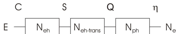
Figure 4.1.: Scheme of the conversion of the deposited energy, E , into signal electrons, N_e , at the SDD anode, with the efficiencies \bar{C} , \bar{S} , \bar{Q} and \bar{\eta} .
