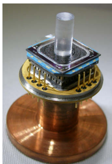
Figure 6.1.: Photo of a 100 mm 2 SDD coupled to a cylindrical scintillator.
