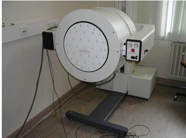
**Fig. 4.17:** Anger camera used as an absorption detector for the Compton camera system
