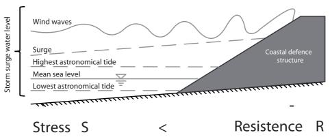
Figure 1-1: Coastal engineering concept for the design of coastal defence structures.
