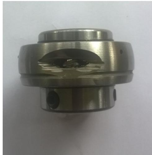
Figure 7.28: Fault at the damaged bearing
