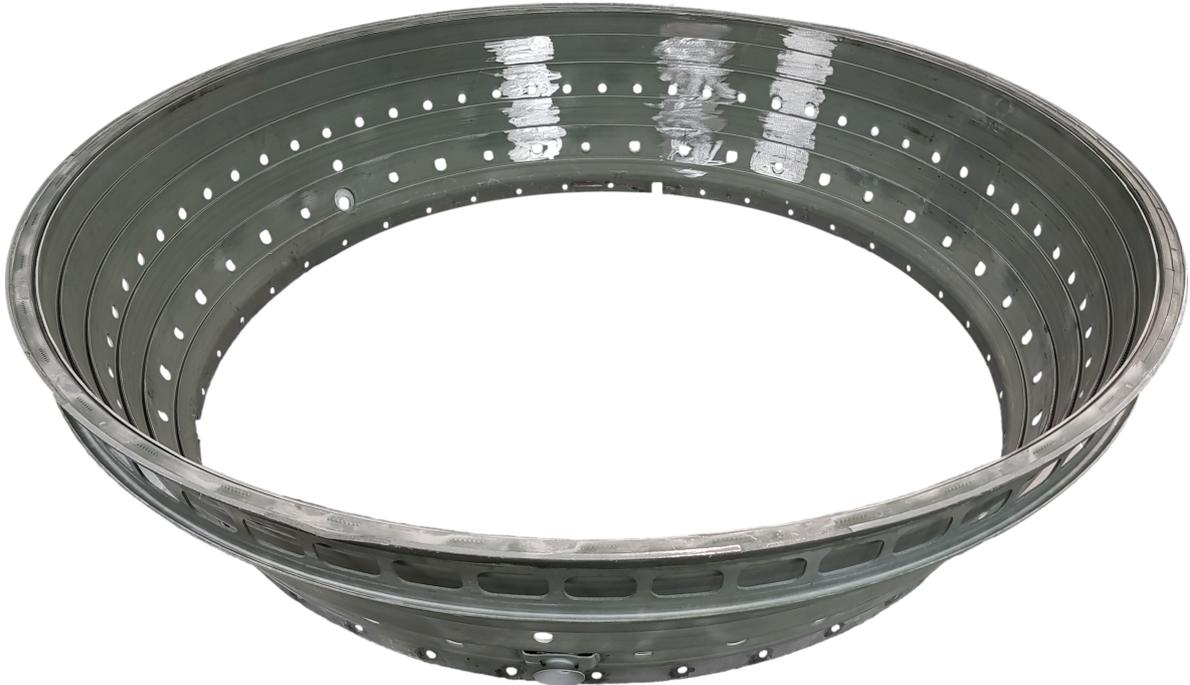
*Figure 1.2: A CFM-56 outer liner. The liner has been heavily repaired before and is no longer an active component.*
