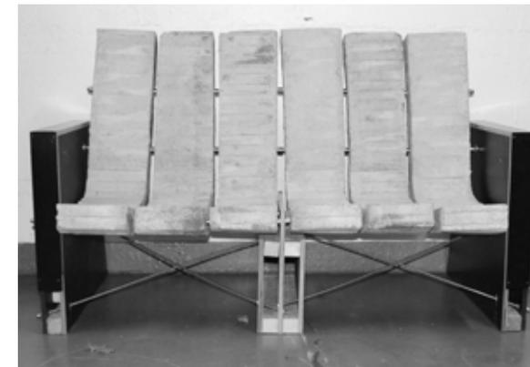
Working in groups of up to eight people, students were tasked with creating a bench with concrete seat shells, with the bench made up of different shells, each about 21 cm in width. Material was provided for the concrete elements to enable students to design the base frame themselves.
