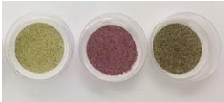
Figure SI 2: F/pF loaded feeding filters. Left: control F/pF; middle: AuNP containing F/pF AuNP ; right: AgNP containing F/pF AgNP .
