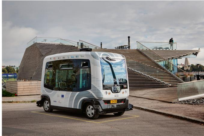
**Fig. 1.3:** Automation level-4 vehicle EZ10 of the company EasyMile in Helsinki. The system is capable to follow learned routes and is used to for last-mile transportation with a maximum velocity of 12 km/h [16].
