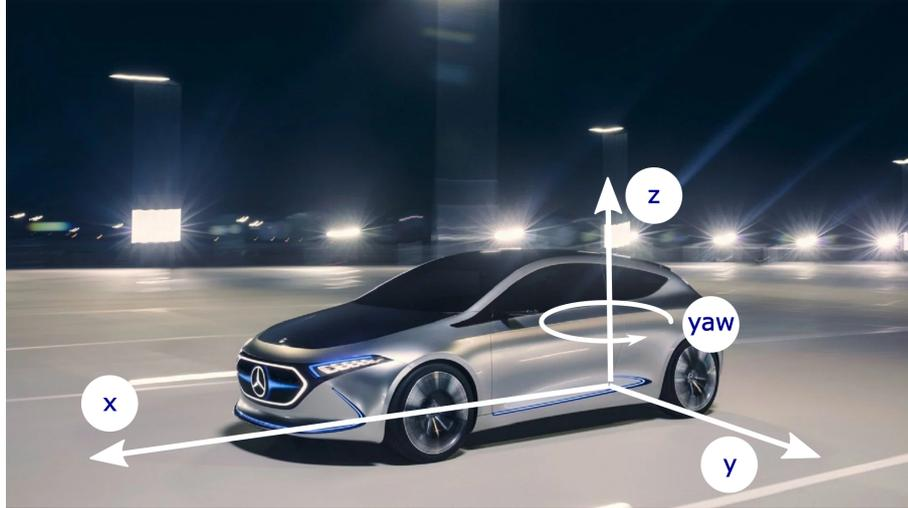
**Fig. 2.2:** Visualization of the intermediate axis system as defined by ISO 8855 and used within this thesis.
