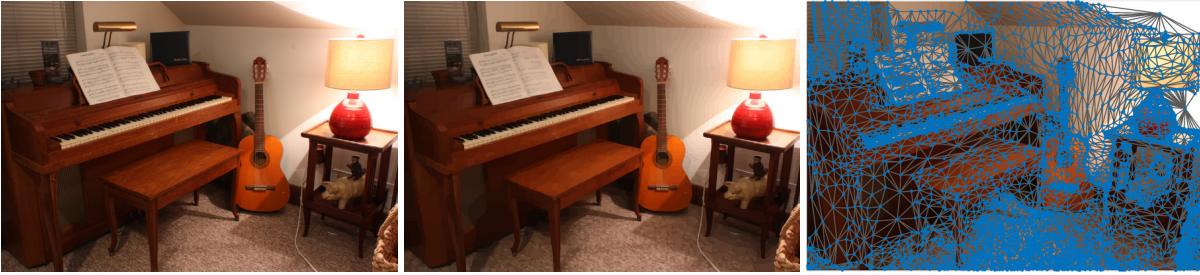
Figure 2.8: Reduction of the raw image (left) to 6031 nodes in the graph structure (Right). In the middle we reproject the graph structure onto the original image, visualizing the high fidelity of the representation, even as the number of nodes reduces to 0.45% of the full grid.
