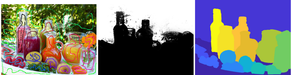
Figure 2.4: Illustrating the use of model-based segmentation methods: The user scribbles different objects to be segmented (left) from which a unary data term f is generated, e.g. by approaches like [207] or a pointwise neural network. As the unaries are insufficient for a good segmentation (illustrated by the fact that a thresholding of the unaries shown in the middle does not segment the background well), the proposed framework offers an efficient approach to obtain accurate segmentations as shown on the right.
