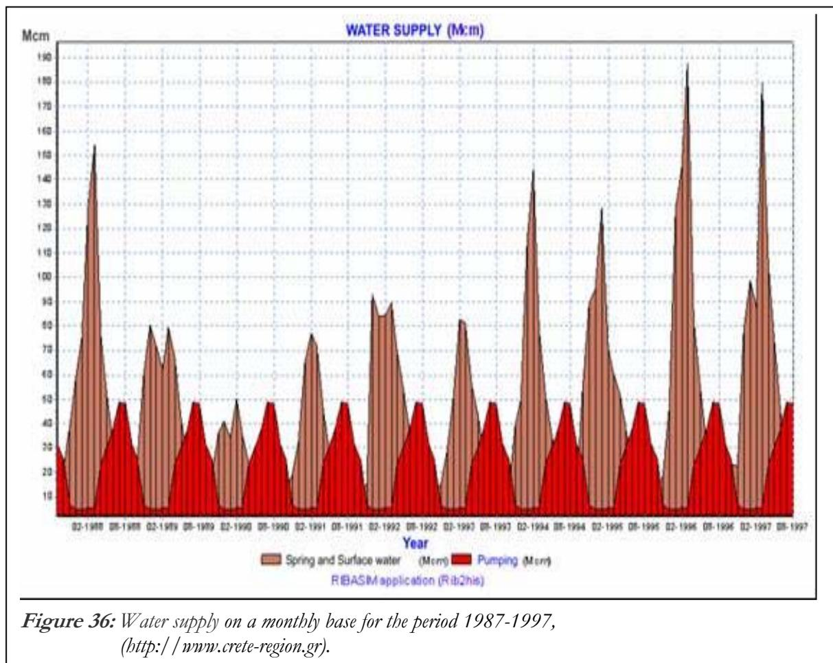
*Figure 36: Water supply on a monthly base for the period 1987-1997, (<http://www.crete-region.gr>).*
