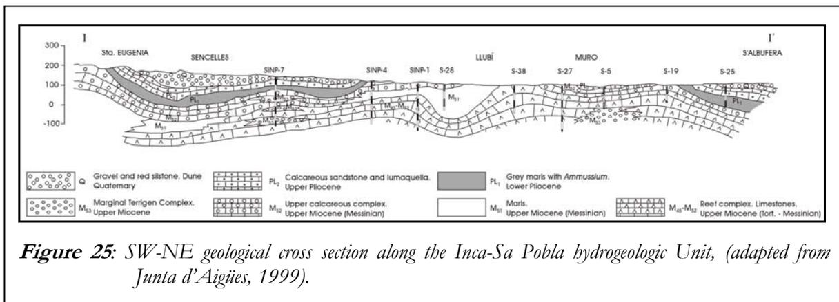
**Figure 25:** SW-NE geological cross section along the Inca-Sa Pobla hydrogeologic Unit, (adapted from Junta d'Aigües, 1999).
