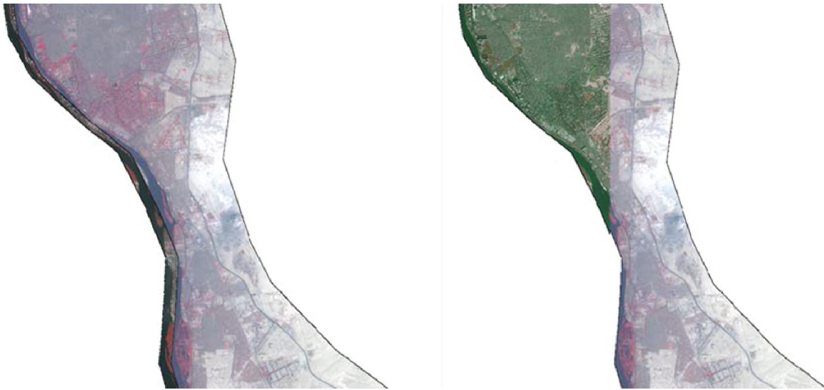
Figure 26: Pre-classification synchronizing process to match the used images to detect dynamic changes. Left: two images before synchronizing. Right: after synchronizing process (Erdas Imagine)
