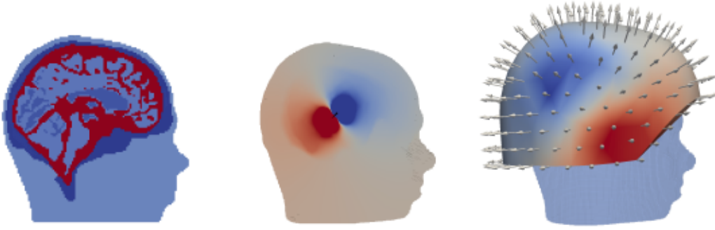
Figure 3.15.: Exemplary EEG and MEG forward computation for an auditory source computed using DG-FEM in a realistically shaped head model. Hexahedral mesh with 2 mm resolution, 6 compartments, sagittal slice (left); electric potential distribution visualized on the clipped volume conductor model in the sagittal plane where the auditory dipole (black cone) lies (middle); MEG solution interpolated on the radial magnetometers including a volume rendering of the head model (right).
