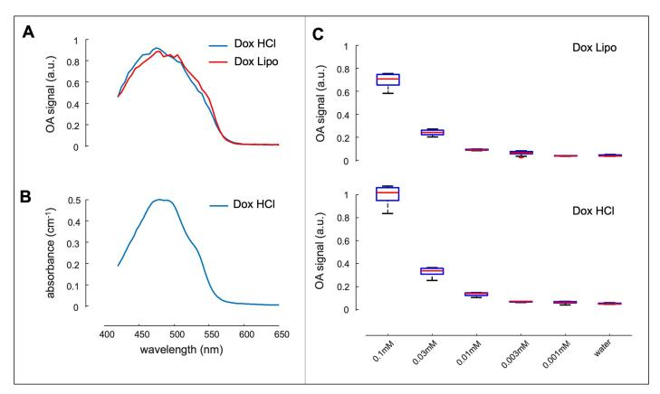
**Fig 1. Optoacoustic properties of DOX** *in vitro*. (A) Optoacoustic measurement of Dox·HCl and Dox·Lipo. Both formulations show a maximum peak at 480/490 nm. (B) Spectrophotometric assessment of Dox·HCl revealed a peak fluorescence at 480/490 nm. (C) Detection limit *in vitro* of Dox·HCl (lower curve) and Dox·Lipo (upper curve). For both formulations the limit was determined at 0.01 mM. Experiments were done in triplets.
