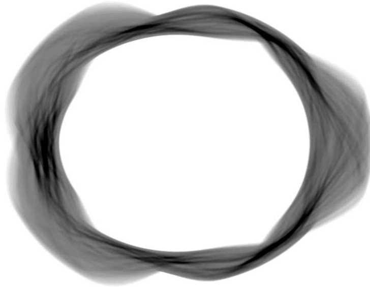
Figure 3.5: RZG VisualKit visualization of a Wendelstein 7-X flux tube. The physical data was calculated by P. Xanthopoulos using the GENE code, with the geometry stemming from the TRACER code. In the case depicted here, the flux tube seems to loop onto itself after one toroidal cycle, but this effect is purely coincidental.
