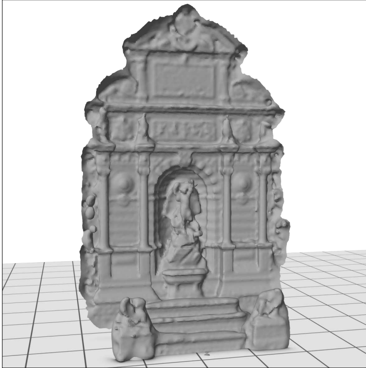
(a) Screened Poisson Surface Reconstruction.
