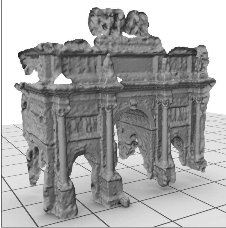
(a) Screened Poisson Surface Reconstruction.
