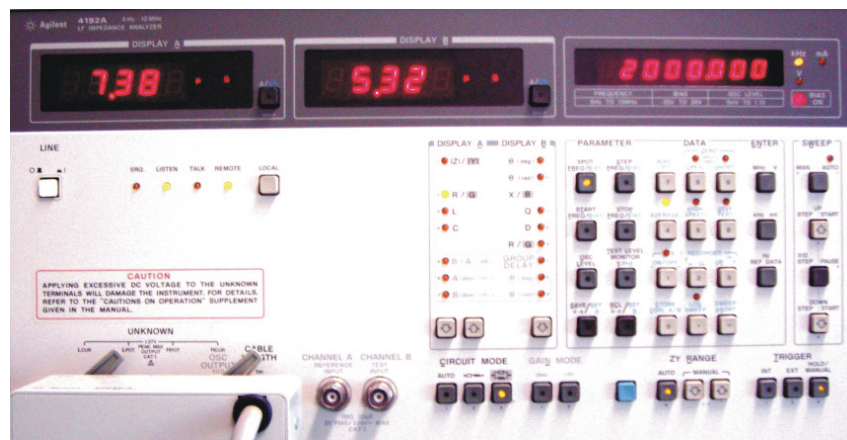
Fig. 2.9 Impedance analyser Agilent 4192 LF.
