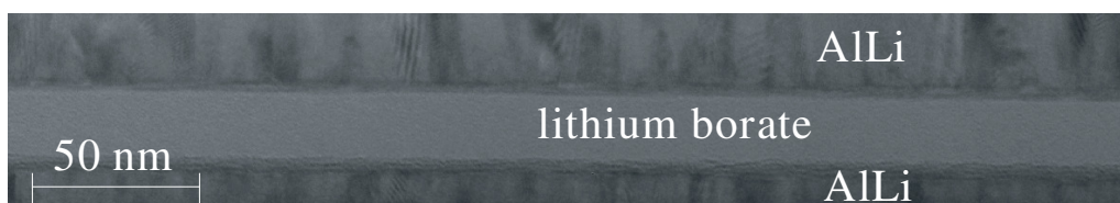
Fig. 3.18 A sputtered lithium borate glass film with a thickness of 21 nm between two AlLi electrodes
