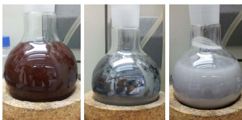
Figure 54: Preparation of PdSO 4 -Alox. Left: directly after addition, middle: after 2 h, right: after 5 h.
