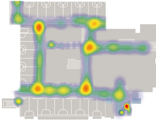
Figure 5.1: Example for a heat-map laid upon a floor plan. Often visited areas such as corridor intersections (e. g., the T-junction on top left) appear thicker and are colored in yellow or even red as several data points converge on the same coordinates. Less frequented corridors have fewer data points on top of each other to visualize. Their visualizations are faint and therefore colored in green or even blue (e. g., the corridor between the top two T-junctions). Source: [404].
