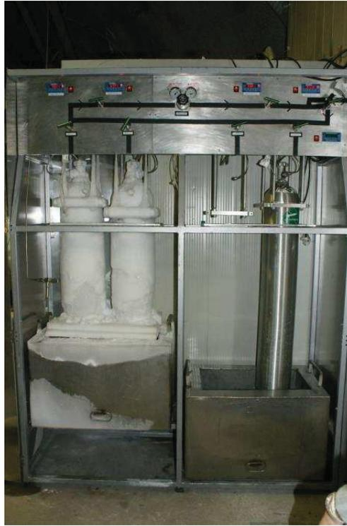
Figure 3.15: Picture of the bottle rack while recuperation is ongoing. The bottles are frozen with LN2.
