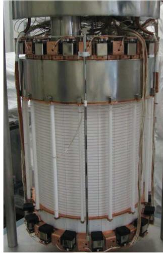
Figure 3.4: The XENON100 Detector [15]
