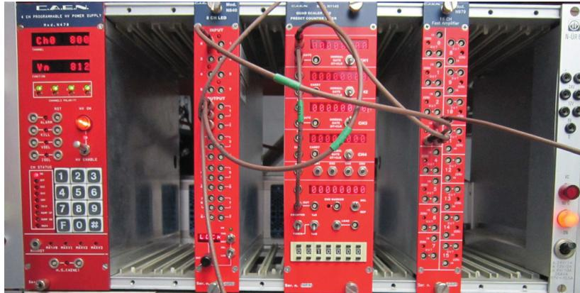
Figure 7.13: A photo of the trigger logic for data acquisition. From left to right, the high voltage supply, the LED, the counter timer and the fast amplifier.
