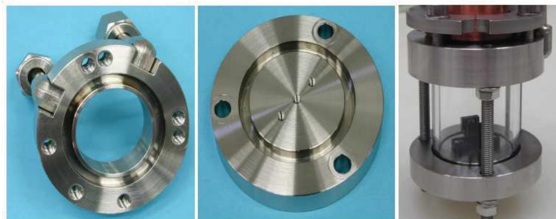
Figure 7.5: The sealing of the quartz tube. Left: the top flange with the xenon supply and return lines welded to it. Middle: the bottom flange, with the holes to screw the teflon holder in place. Right: the final assembly with the tube sealed and the teflon and teflon holder inside
