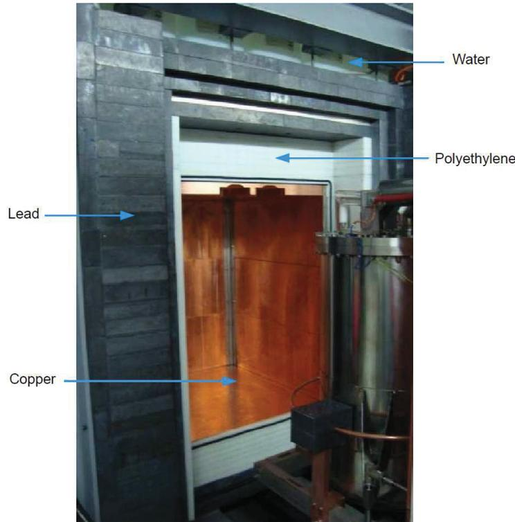
Figure 3.12: The shielding structure of the XENON100 experiment. The copper, polyethylene and two lead layers are clearly visible while the water boxes are starting to show on top.
