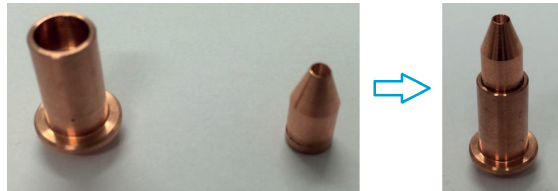
Figure 3.6: The final Laval nozzle for the jet target MCT-M for the MAGIX experiment. Left: The nozzle holder (right) and the Laval nozzle (left) which is shrunk on the nozzle holder. Right: The final nozzle consisting of the Laval nozzle and the nozzle holder. Pictures taken by D. Bonaventura.
