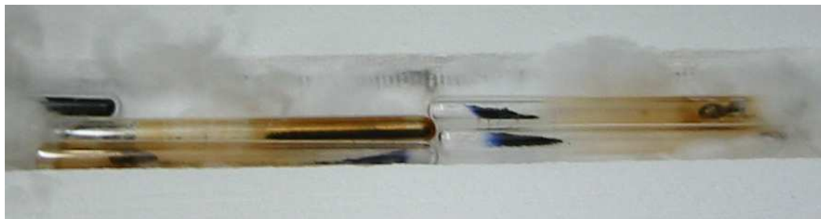
Figure 4-1: Glass ampoules inside an opened tube furnace. The sodium metal is on the cooler side of the tubes. The sodalite powder is located near the center of the furnace. The two tubes on the right clearly show the black frontier of already doped sodalite moving through the undoped part. The central sample on the left side is already completely doped. The sample in the upper left part is being distilled (one end of the glass tube sticks out of the furnace. The white material is glass-wool.
