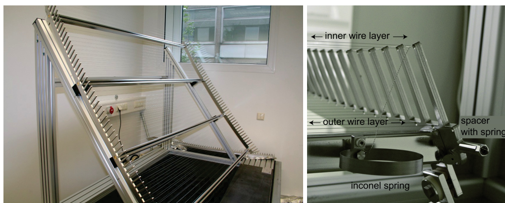
Figure 3.4: Double layer wire electrode module before installation. The left picture shows the combs and c-profiles representing the support structure of an electrode module. In-between, the wire layers are stretched from comb to comb. The other picture denotes a detailed view of a module edge, equipped with the high voltage distribution connectors.
