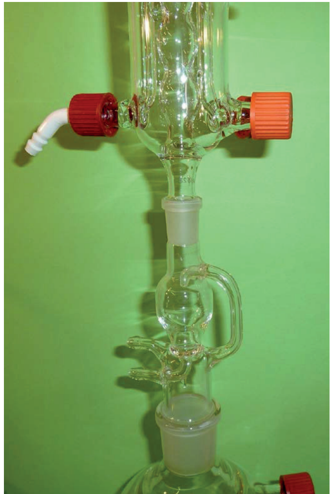
Fig. 4.4.04.: Glass oxygenator with associated reservoir. Both are jacketed for temperature control by means of a circulatory thermostat. On the left is an interrupted overflow outlet to which a valve can be attached to regulate the input of compressed air, on the right there is shown an uninterrupted overflow from the oxygenator to the reservoir (design by Schurek, unpublished).
