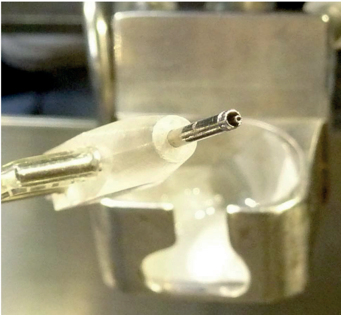
Fig. 8.2.09.: Detailed view of the double-barreled cannula. Note the protruding inner (pressure-measuring) cannula, as well as the circumferential groove used to fix the binding ligature. The protruding inner cannula acts as a "pioneer" and facilitates intubation of the slit-cut aorta. For further details see Technical Appendix.
