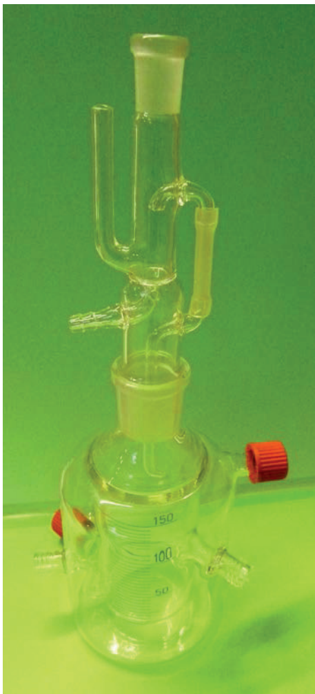
Fig. 4.4.04.: Glass oxygenator with associated reservoir. Both are jacketed for temperature control by means of a circulatory thermostat. On the left is an interrupted overflow outlet to which a valve can be attached to regulate the input of compressed air, on the right there is shown an uninterrupted overflow from the oxygenator to the reservoir (design by Schurek, unpublished).
