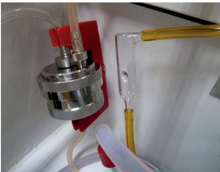
Fig. 5.1.10.: Windkessel-extension . The pressure buffer can be varied in height or fully clamped off, e.g. to achieve a pulsatility of flow and pressure. On the left is an in-line filter with a vent port (Sartorius, Göttingen, Germany).
