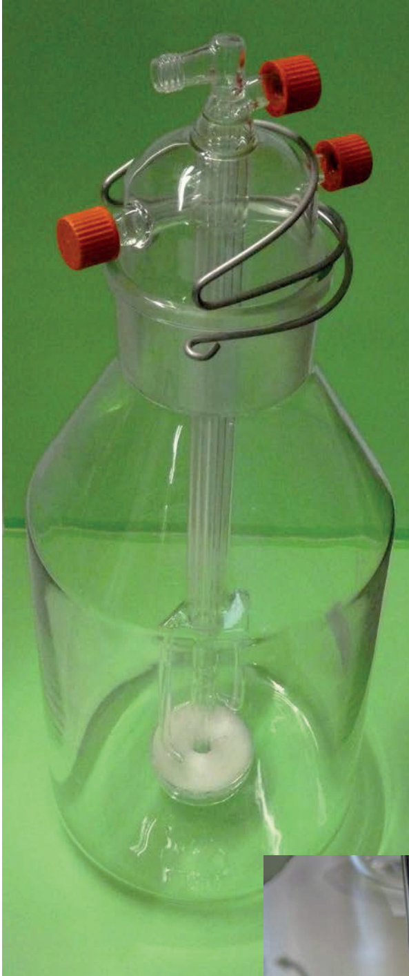
Fig. 5.1.02.: 5-liter wide-mouth bottle with ground-glass frit (size NS86/55) attached to a plunger with four ports.
