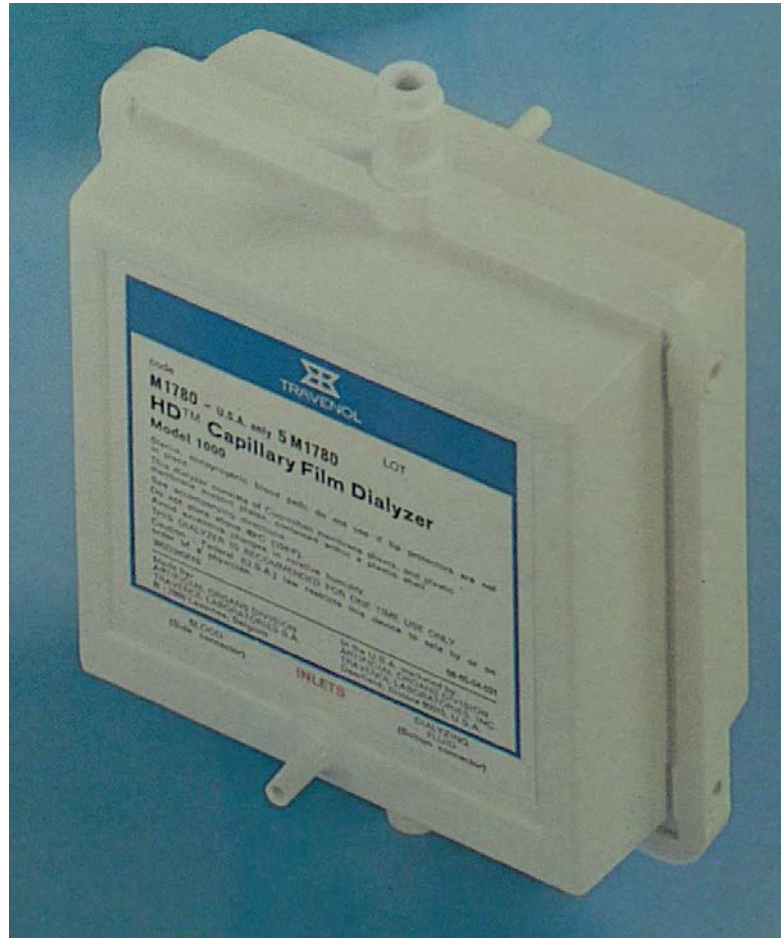
Fig. 4.4.12.: Hoeltzenbein-dialyzer (HD™ Capillary Film Dialyzer). Historical model M1000, once produced in Belgium by Travenol Laboratories Inc. The inlet for blood/perfusate is on the front, the outlet on the rear face. Dialysate enters and exits via the Hansen couplings on the bottom and top, respectively. The surface area of the dialyzer membrane was 0.92 m 2 , the filling volume 65ml and the ultrafiltration coefficient was low. Dialysate flow was driven by a centrifugal pump at low pressure (Type 1022 Eheim GmbH, Delzisau, Germany), see Chapter 5.3.
