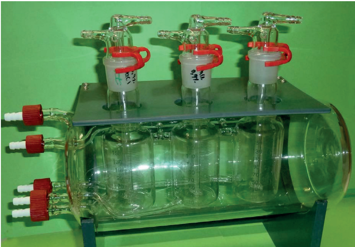
Fig. 5.4.3.: Temperature-controlled triple chamber. This allows three different solution variants to be used sequentially for recirculation perfusion. Between changes, an aliquot is discarded in single-pass mode to avoid a contamination of the following solution. The upper ports are connected to the circulation thermostat. The three ports below connect the three chambers.
