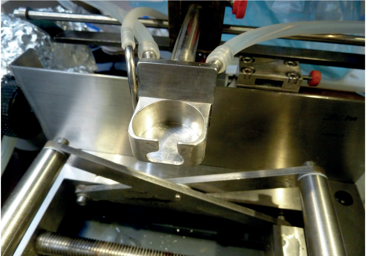
Fig. 8.2.06.: The heated stainless-steel tray currently used for the right kidney. Note the lateral suction tube. The asymmetrical cutout in the front wall is designed to accommodate the ureter caudally. The tubing attached to the rear block feeds into a U-shaped channel. Also visible is the scissor lift for the operating table.
