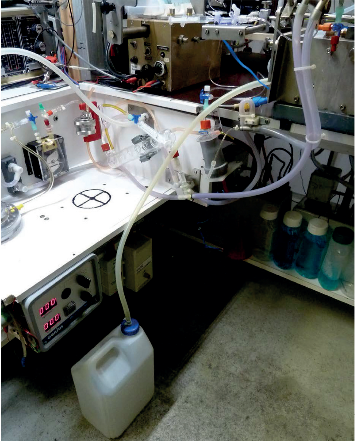
Fig. 5.1.16.: Effluent reservoir with inlet tube. On the left the perfusion pump, the in-line filter and the jacketed glass coil. The (bronze-colored) feedback-controlled infusion pump is mounted on top. On the bottom left are control modules for the magnetic stirrer that mixes perfusate with the test infusion and for the peristaltic pump for the gas pressure measurement ( pO_2 ).
