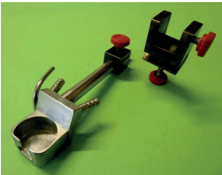
Fig. 5.1.12.: Water bath heated kidney tray made of stainless steel. The insert holder permits loading from above, so that the kidney can be placed in the kidney tray with the renal hilum projecting from the opening in the front wall. The tray on the left has a suction tube laser-welded to the sidewall. For details and dimension, see Fig. 15.0.8 at the Appendix.
