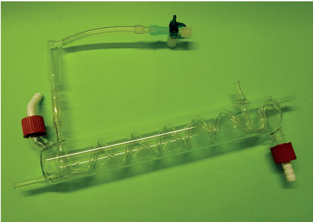
Fig. 4.5.4.: Temperature controlled glass coil with buffering chamber ( Windkessel ), bubble trap , and return connection. Perfusate flows from left to right. The volume of the buffering chamber visible at the left end can be changed by adding an extension on top, as shown (s.a. Fig. 4.5.3.). On the right is a T-outlet that provides for the return of medium to the reservoir prior to the start of perfusion, which avoids “no flow” areas. Dimensions: overall length: 295mm, o.d. of glass tube 38mm, glass coil o.d. 6mm, i.d. 2.5mm. Glass screw thread standard GL 14 for water circulation thermostat.
