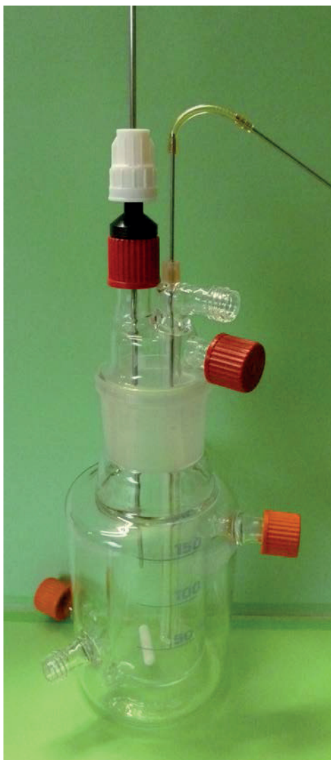
Fig. 15.1.3.: Detailed view of perfusate reservoir with level control. The sensing probe on the left is adjustable in height, and serves as one of the electrodes for the refill control to compensate for losses during ultrafiltration of the dialyzer and withdrawal of urine samples. The thin stainless steel tube on the right serves both as a second electrode and as the return path for aliquots used for oxygen pressure measurements. See Fig. 5.3.2.
