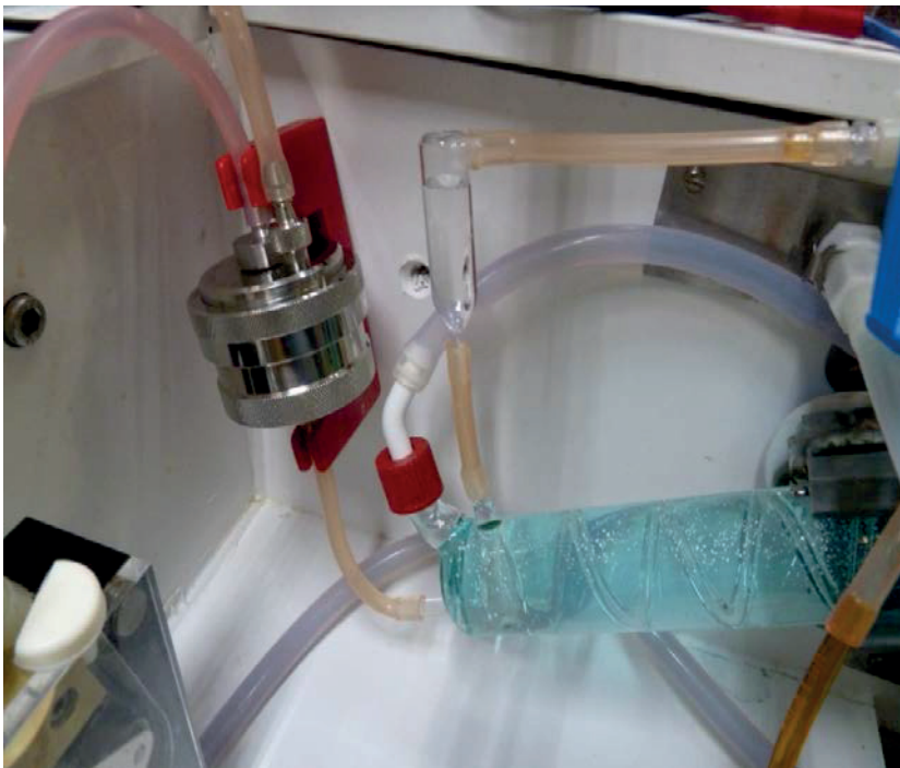
Fig. 4.5.3.: In-line filter. The cellulose nitrate filter (42mm diameter, pores 8 \mu\text{m} ; Sartorius, Göttingen, Germany) on the left is inserted between the perfusion pump and the glass heating coil with pressure buffer (Windkessel) and bubble trap. A screw-vent connection can be seen at the front end of the filter. To vent the lower chamber, rotation of the filter is necessary during the preparation.
