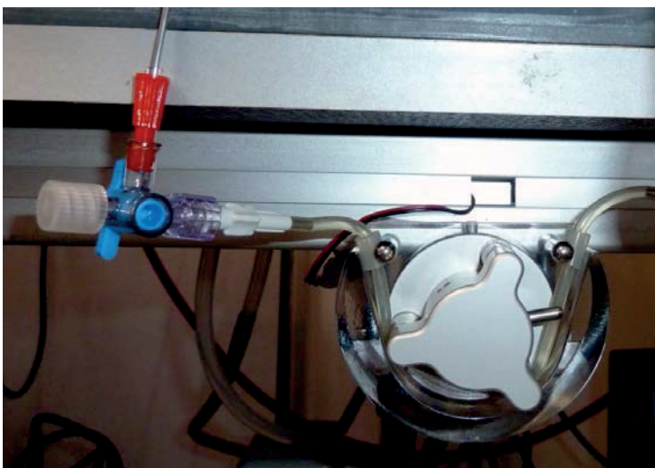
Fig. 5.1.14.: Small roller pump. This is used to supply the flow cell (at 3 - 4ml/min) during pO_2 -measurement.
