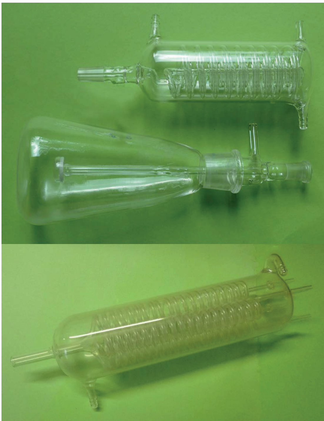
Fig. 15.0.1.: Ensemble for humidification and heating of gases. Gases are pre-warmed in the water-jacketed glass coil at the top, humidified by passage through the ground-glass frit into distilled water in the Erlenmeyer flask which is placed in a water bath (see Fig. 5.1.01). Gas is reheated by passage through the glass coils in the lower panel, thus avoiding transfer of condensate into the perfusate. The 4-fold coil was originally designed for studies (in the single-pass mode) of the effects of different substrates on sodium transport. Up to 4 Woulff bottles, each filled with 2 liters of a different perfusate, could be connected in series (256, 257).
