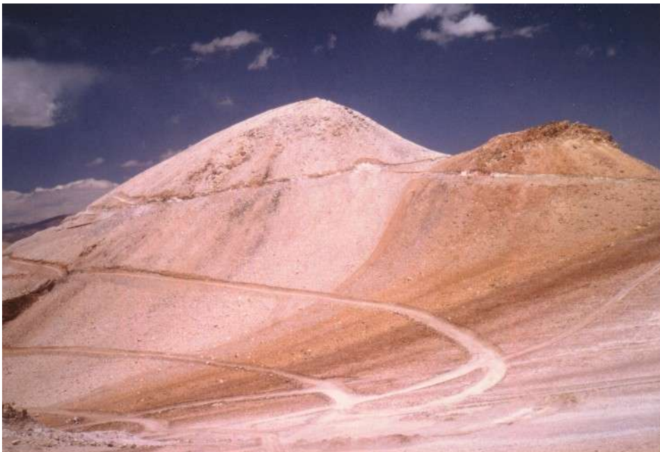
Fig. 3: Hydrothermally altered and argillized Neogene pyroclastics southwest of Can Can (test site II), showing a high albedo in the visible spectra.
