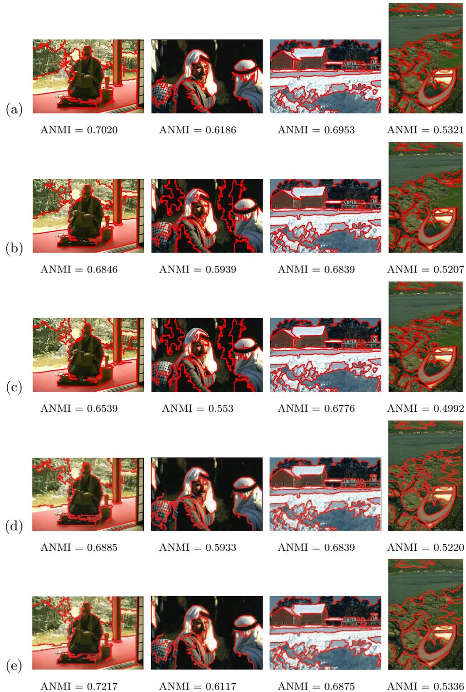
**Figure 8.4.** Examples of segmentation results on parameter subspace data. (a)-(c) The best, average and the worst input segmentations. (d) Set median segmentation. (e) Generalized median segmentation.
