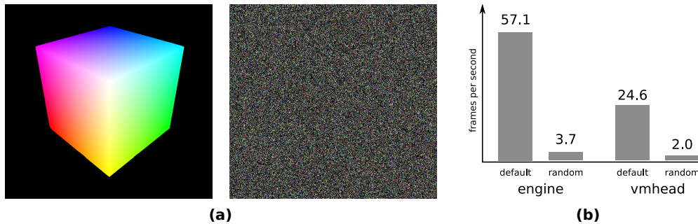
Figure 6.1: (a) Ray start point texture before and after applying a random permutation. (b) Frame rates for raycasting two data sets using the default as well as the randomized start points.
