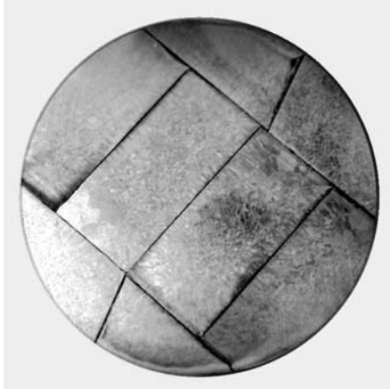
Figure 3.18: \text{Ni}_x\text{Fe}_{(1-x)} target prepared by melting pure Ni and Fe materials.
