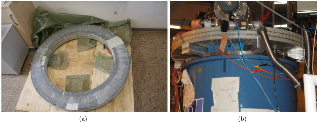
Figure 3.7.: Pictures of the compensation magnet just unpacked right after delivery from the company (a). The compensation magnet after installation on top of the cryostat that holds the two superconducting magnets (b).
