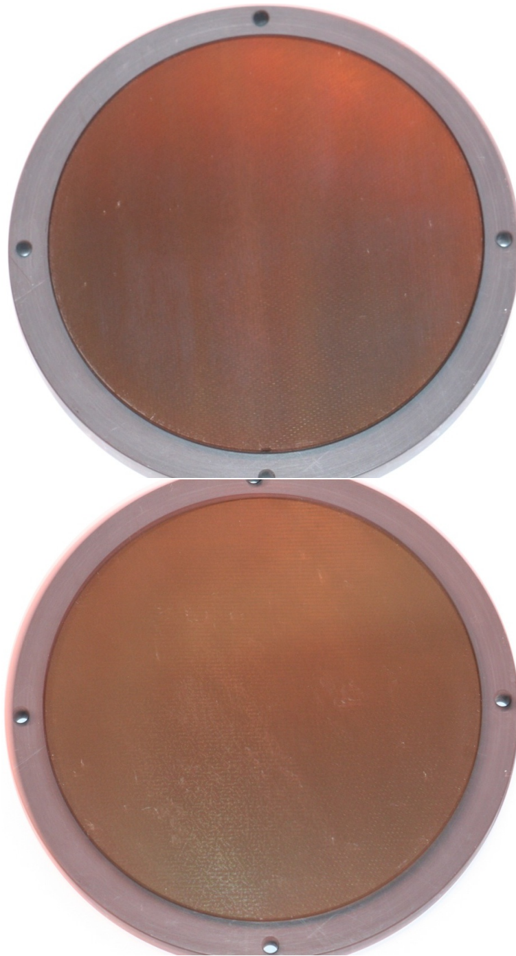
Figure 2.8.: Pictures of the back MCP laying in the transport box from the front side (top) and the back side (bottom).
