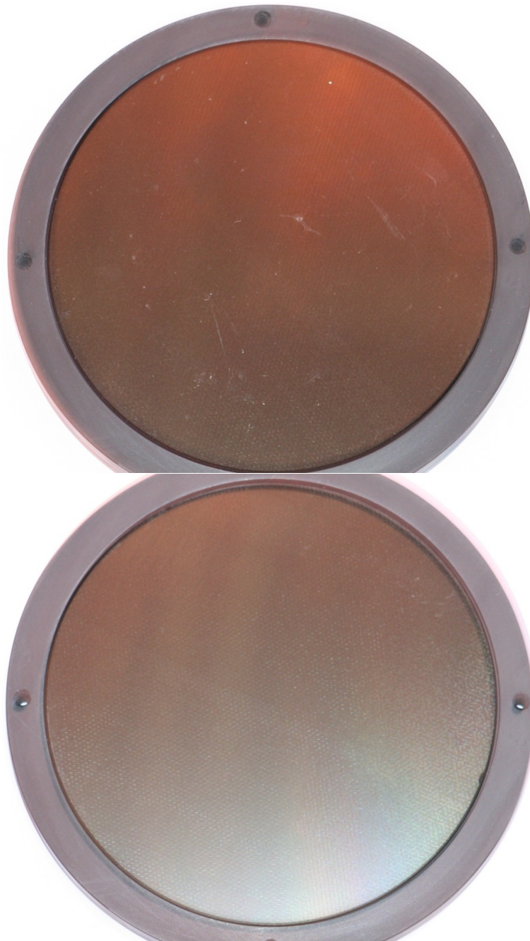
Figure 2.7.: Pictures of the front MCP laying in the transport box from the front side (top) and the back side (bottom). The top side of the MCP has been longer exposed to atmosphere, which explains why it is more contaminated with dust.
