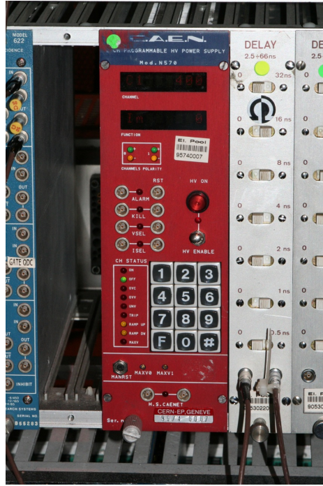
Figure 2.19.: The CAEN 570N power supply used for the voltage supply of the detector.
