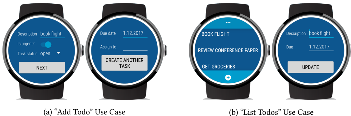
Figure 4.18: Generated Wear OS App for the System Modelled in Figure 4.17 (cf. [RK19a])
