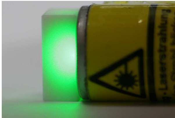
Figure 5.10.: Light transmittance through a PTFE sample: a laser pointer (right) with the wavelength 532 nm shining vertically on a PTFE sample of 5 mm thickness. The light penetrates into the sample and also leaves through the side walls.
