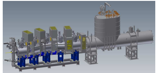
(b) CAD drawing of the transport section of the KATRIN experiment.
