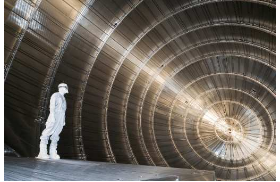
(b) Picture inside the KATRIN main spectrometer with the wire electrode installed.
