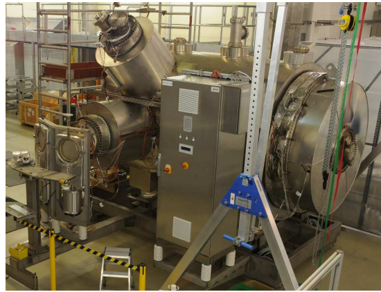
(b) Picture of the KATRIN pre-spectrometer during build up in the KATRIN hall.
