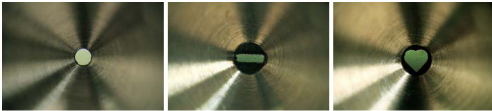
Figure 5.51.: Installed collimators with circular (diameter 0.5 mm), rectangular (( 780 \times 190 ) \mu\text{m}^2 ), and heart shaped opening (maximal length 760 \mu\text{m}^2 ).
