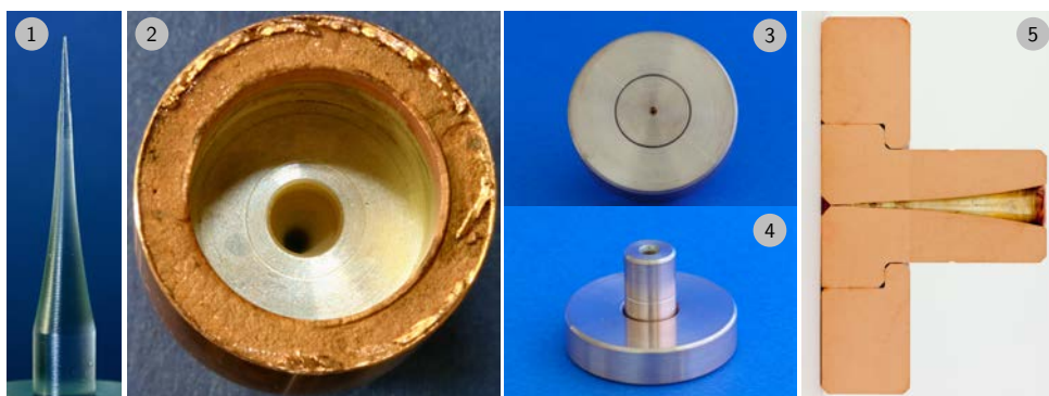
Figure 4.6.: Laval nozzle production: (1) positive model of the nozzle trumpet (polymethyl methacrylate), (2) galvanised nozzle body (copper), (3) finished Laval nozzle inlet and (4) outlet part, and (5) cross-section of the Laval nozzle (Image (1) and (2) taken by W. Hassenmeier, (3) to (5) taken by D. Bonaventura).
