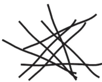
(a) The isotropic case. Fibres are not aligned.
