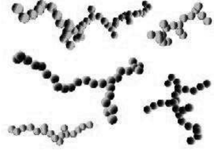
**Fig 2.1** Three-dimensional reconstructions of agglomerates consisting of  $\text{SiO}_2$  spheres with  $0.95\mu\text{m}$  monomer radius. In the CODAG experiment, stereo images were obtained which allowed to reconstructing the precise agglomerate morphologies (Wurm 2003; Blum et al. 2000).
