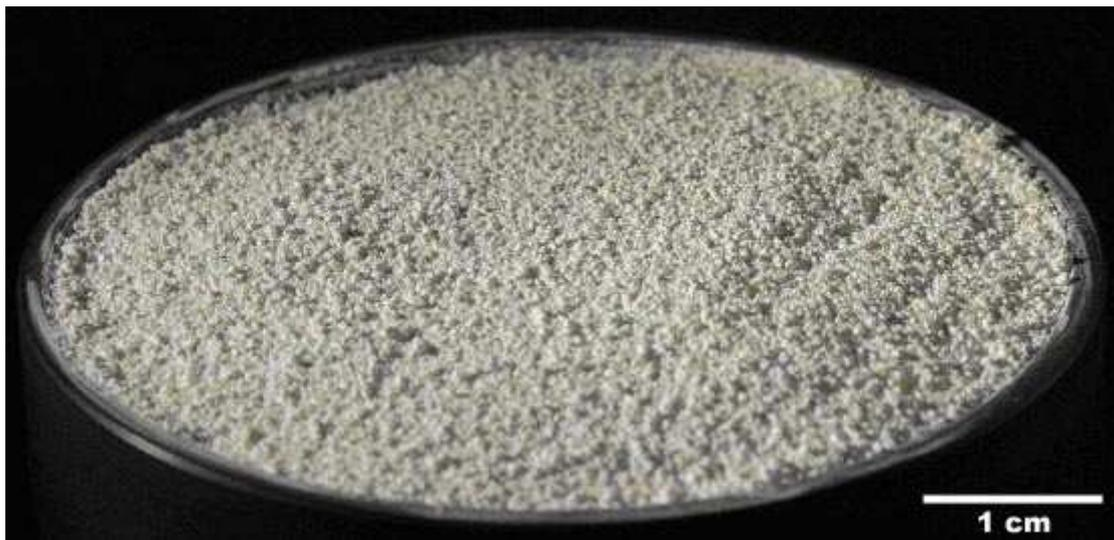
*Fig. 3.6 Porous target. A porous target prepared by sieving powder with a 0.5mm mesh. The sieving results in a granular structure of the surface. The individual grains are up to 0.5mm in size.*
