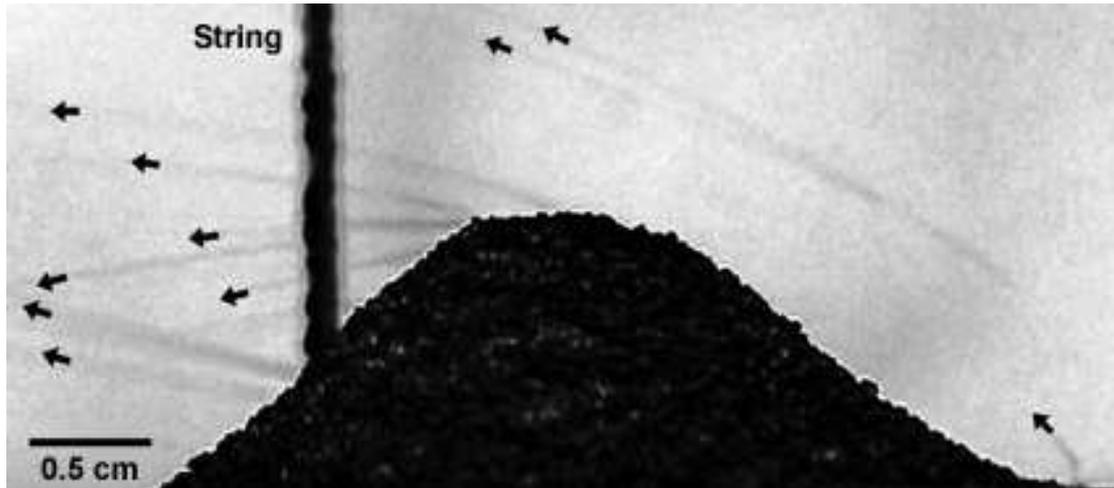
**Fig. 5.4** Video image of trajectories of dust entrained in the gas flow. The dust pile is placed in a gas flow at 3mbar and 63m/s. The direction of the gas flow is from right to left. Individual trajectories are marked by arrows. The vertical line is one of the strings of the supporting string cradle. The top of the pile is already eroded and therefore the pile is more flat with a less pronounced tip.
