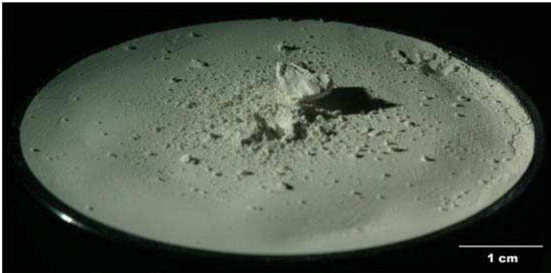
*Fig. 3.22 Impact with a compact target at  $11m/s$ . Impacts at this velocity don't give rise to a pile. The projectile survives the impact (or breaks up into 2-3 big pieces) and stays lying on the target surface. This will be not the case in microgravity.*
