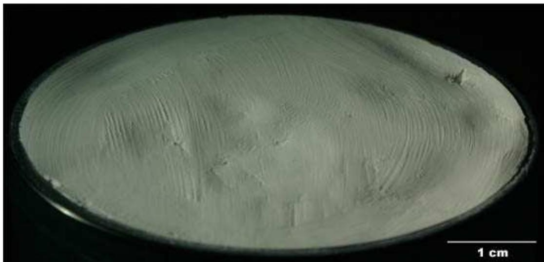
*Fig. 3.15 Compact target. A compact target prepared by manually compressing the dust in the target tray. Target porosity is  $65.7 \pm 1.0\%$ .*
