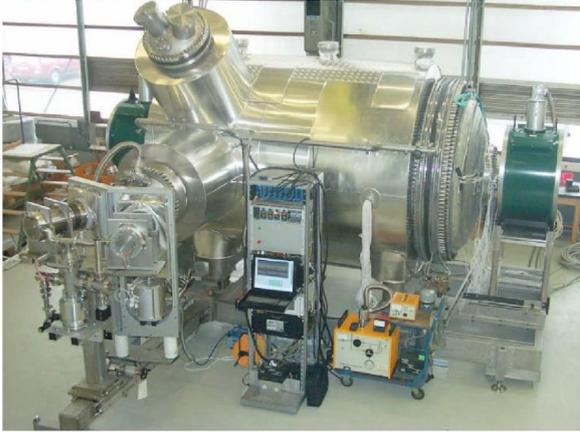
**Figure 2.8:** Photograph of the KATRIN pre-spectrometer. The stainless steel vessel is encased in the heating/cooling system. A superconducting magnet is placed at either end of the spectrometer.
