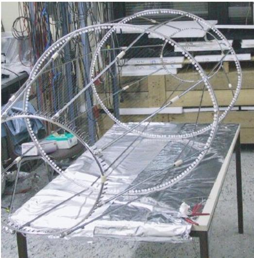
**Figure 3.2:** Photograph showing the wire electrode of the “Mainz IV” setup before insertion into the spectrometer (photo taken from [Fla04]). The grid is segmented into three parts: besides the central cylindrical section, two conical wire segments were added in order to cover a larger fraction of the solid electrodes as compared to the “Mainz III” setup.
