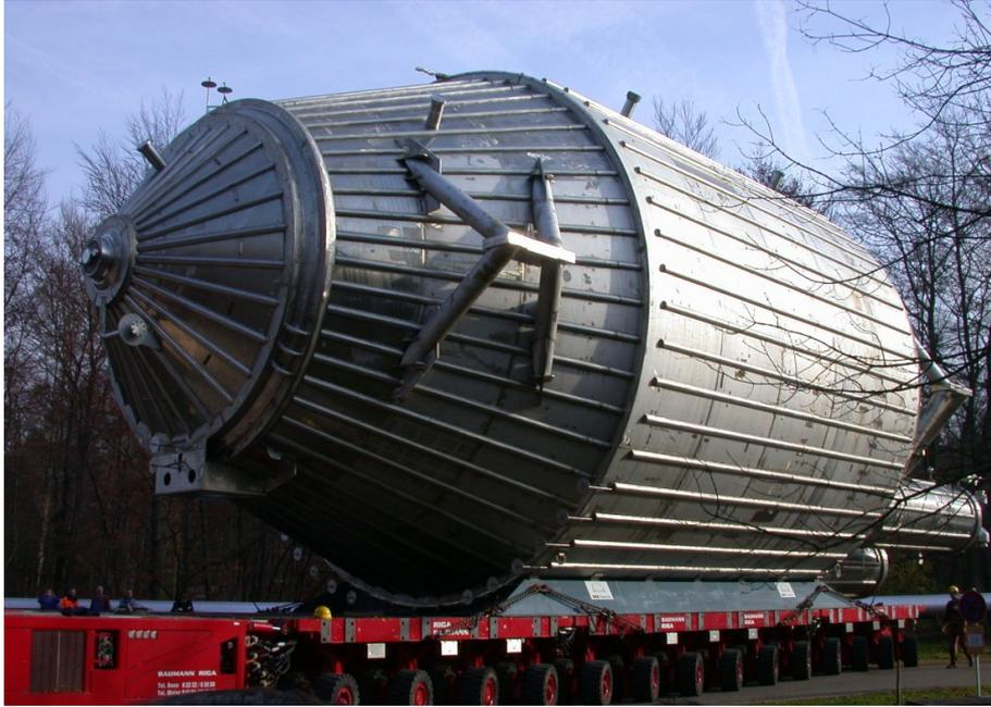
**Figure 2.7:** Photograph of the KATRIN main spectrometer vessel during transportation to the spectrometer building on site of Forschungszentrum Karlsruhe in November 2006. A comparison with the height of the person depicted in the lower right corner of the image demonstrates the dimensions of the spectrometer.
