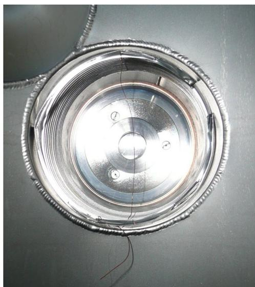
**Figure 6.32:** Stationary wire (no scanning mechanism provided) tested between the second and third wire scanner measurement phase at Mainz.
