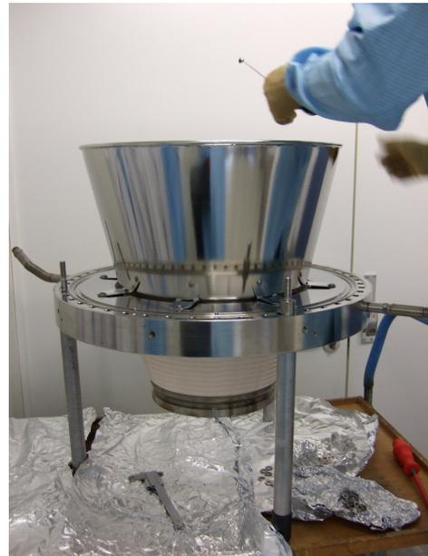
(b) shielding electrode mounted on flange (with ceramics insulator)
